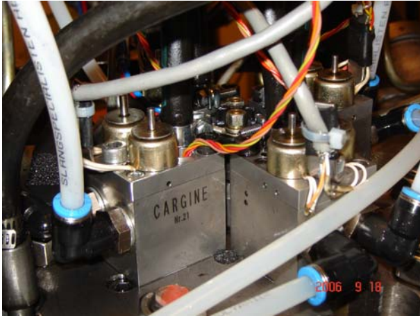
Figure 3 The pneumatic valve actuators mounted on the Scania cylinder head
