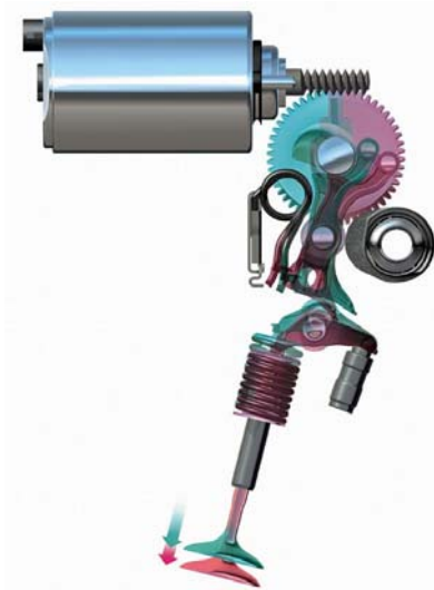
Figure 17 Illustration of BMW's Valvetronic mechanism [33].
