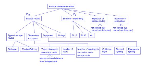
Figure 3: Provide Movement Means
