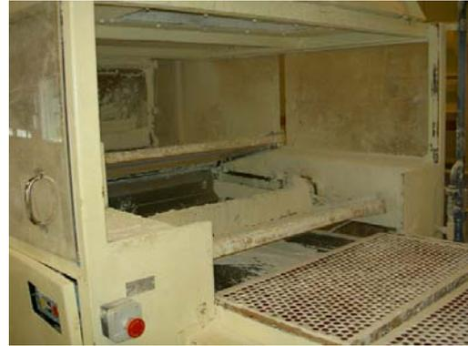
Figure 12, The dried trays are flipped over
