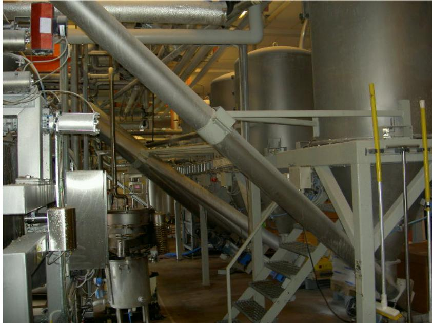
Figure 8, GA kitchen, dry powder containers to the left and screw conveyors in the centre
