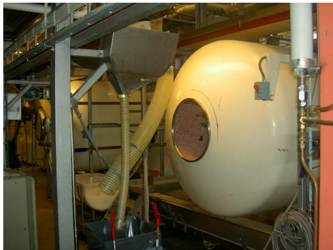
Figure 9, Automatic drageé barrel
