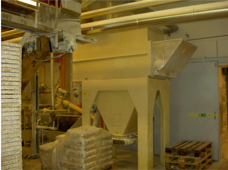
**Figure 13, Process filter in the moulding line hall;
