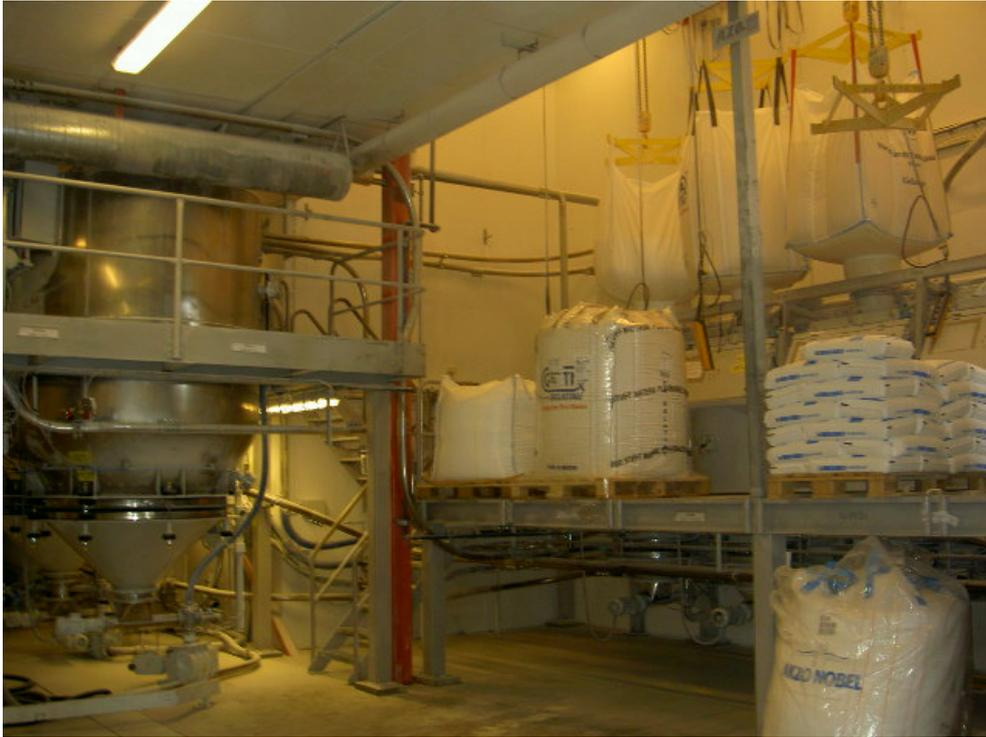
Figure 5, Main Gum Arabic silo to the left, emptying of Big Bags into hoppers to the right
