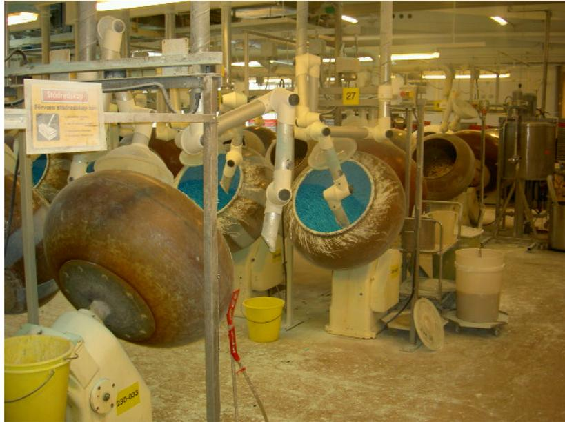
Figure 10, Manual Drageé barrels
