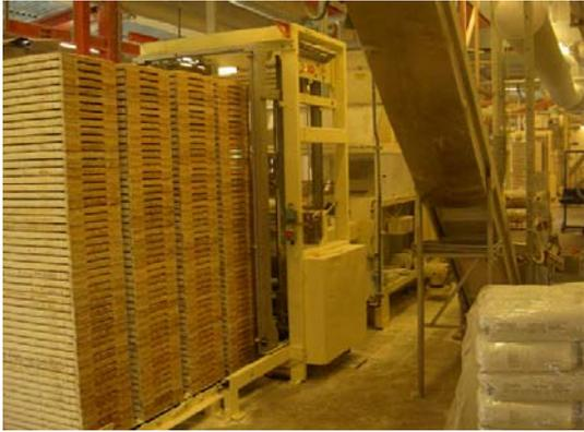
Figure 11, Start of the moulding line
