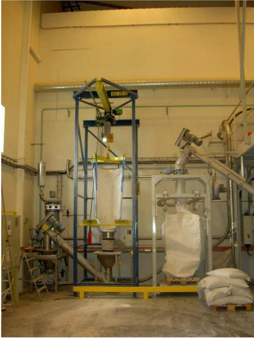
**Figure 3. Emptying sugar Big Bag to the left, filling of crushed Gum Arabic to Big Bags to the right**
