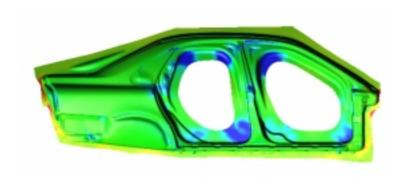
Figure 2: Thickness distribution. The scale shows blue for 20% thinning and red for 10% thickening.
