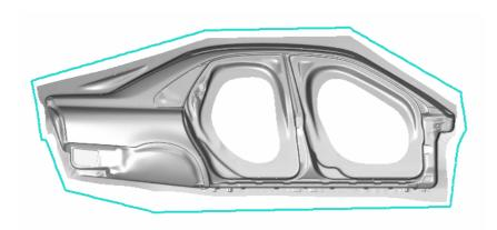
Figure 7: The line shows the sheet position after blankholder closing. The draw in can then easily be measured by a comparison with the line in bottom position.
