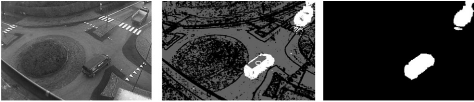
Figure 4 Background–foreground segmentation example. Left: input frame. Middle: foreground probability per pixel (white pixels have high probability of being a foreground whereas the black pixels have a very low probability). Right: resulting segmentation
