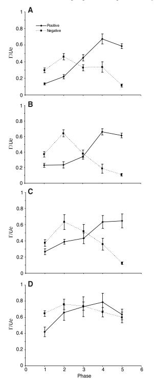
Fig. 7. Normalized total circulation in each phase of the wingbeat, where phase 5 at the right of the abscissa is the beginning of the downstroke and phase 1 at the left marks the end of the upstroke: (A) inner wing (X in Fig. 2), (B) mid-hand (Y in Fig. 2), (C) outer-hand (Z in Fig. 2) and (D) directly behind the body (LR in Fig. 2). Error bars represent ±s.e.m.
