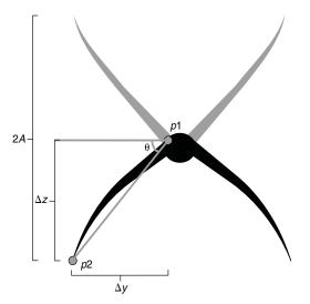
Fig. 1. Rear view of the flying swift showing the method of digitizing from high-speed films. The shoulder joint (p1) and wingtip (p2) are located and with the measurements of distance in the horizontal  $(\Delta y)$  and vertical  $(\Delta z)$  direction between these, the stroke angle  $(\theta)$  can be calculated. The peak-to-peak amplitude, 2A, is the distance between the wingtip at the upper and lower turning point.
