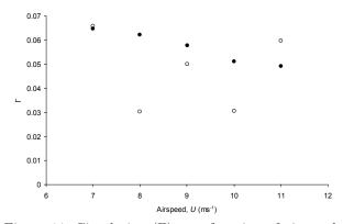
Figure 11. Circulation ( $\Gamma$ ) as a function of airspeed. Filled circles represent wingtip circulation and open circles represent tail circulation. Wingtip circulation decreases with speed, whereas tail circulation shows no apparent relationship with speed. At several speeds the circulation of the tail is of the same order as that of the wingtip.
