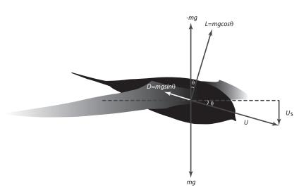
Figure 1. Forces acting on the swift in equilibrium gliding. The glide path is inclined at an angle  $\theta$  to the horizontal and the resultant of the vectors lift (L) and drag (D) is equal and opposite to the weight of the bird (mg). Total speed (U) involves the component sink speed  $(U_s)$ , which is directed downwards and perpendicular to the horizontal.
