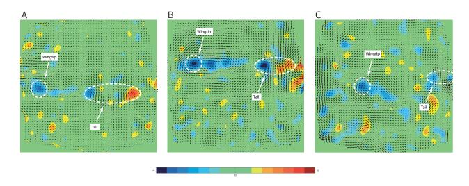
Figure 9. Example images of the vector and vorticity fields at (A) 7 ms<sup>-1</sup>, (B) 9 ms<sup>-1</sup> and (C) 11 ms<sup>-1</sup>. The wingtip vortex is similar at all speeds, but the tail vortices differ. At 7 ms<sup>-1</sup> the tail vortices are farther apart compared to the higher speeds.
