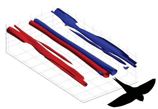
Figure 10. Vorticity isosurface plot at airspeed of 9 ms<sup>-1</sup>. The view is obliquely from above and from the front of the bird's flight path, as indicated by the birdsilhouette. The plot is based on data from one side of the bird, wing and tail, that have been mirrored in the plot to illustrate the complete wake. Tail vortices and wingtip vortices are the major structures in the wake of the gliding swift and appear clearly in this plot.
