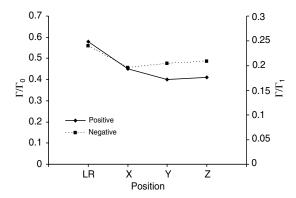
Fig. 8. Maximum observed circulation of any coherent structure in the swift wake relative to two reference circulations,  $\Gamma_0$  and  $\Gamma_1$ , for the power-glider and pulsed ring generator, respectively. On the abscissa, LR to Z are positions given in Fig. 2.
