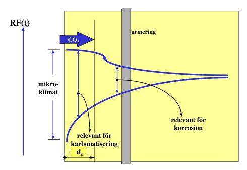
Fig. 3 Carbonation during moisture variations, in principle
