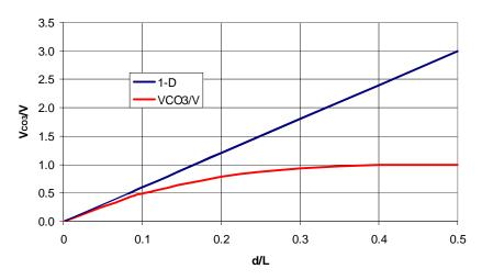
Fig. 1 The volume ratio of carbonated concrete for a cube when using the 1D-model (straight line) or a correct model (lower curve)
