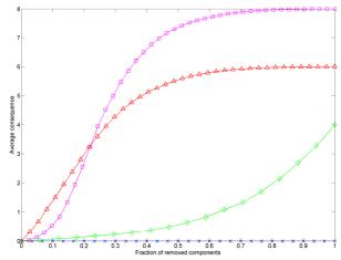
Figure 4. The consequences for the railway system for varying magnitude of the strain when applied to the traction power system ( $\square$ ), the telecommunication system ( $\Delta$ ), the auxiliary power system (x) and the in-feed system (x) are exposed to random removals. The consequences are averaged for 1000 simulations.
