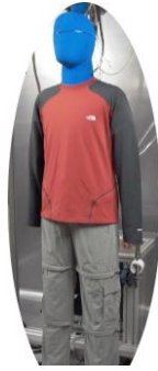
Fig.2 One-segment thermal manikin “Walter”
