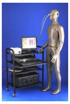
Fig.1 20-zone sweating thermal manikin "Newton"
