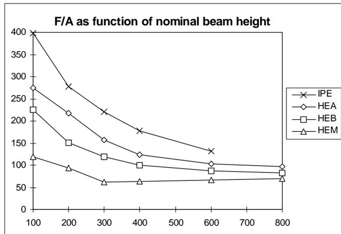
Figure 10.2a F/A as function of nominal beam height (m<sup>-1</sup>).
