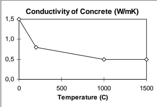
Figure 4.4 b) Conductivity of concrete.
