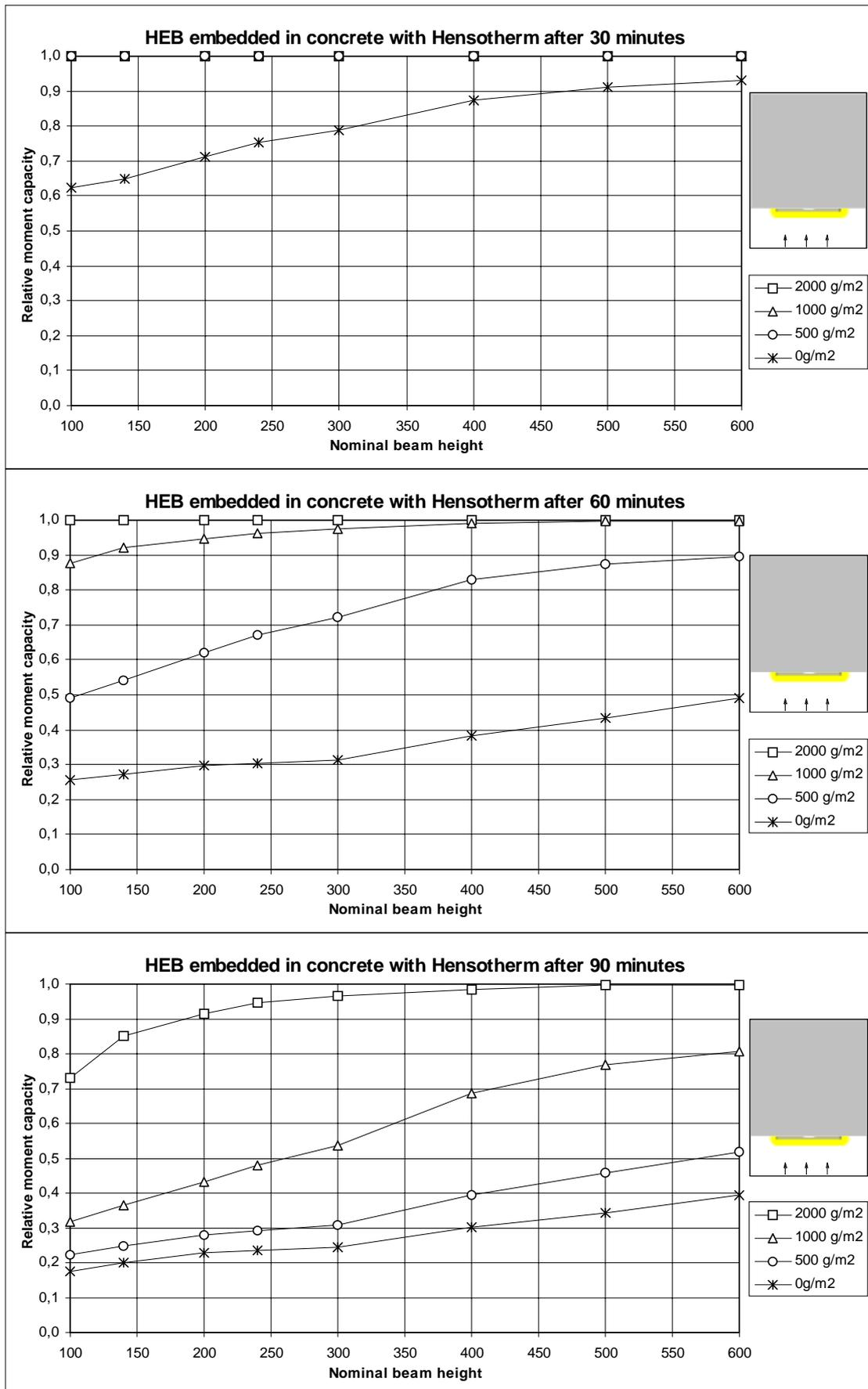
Figure 7.5 Relative moment capacity of HEB-beams embedded in concrete.
