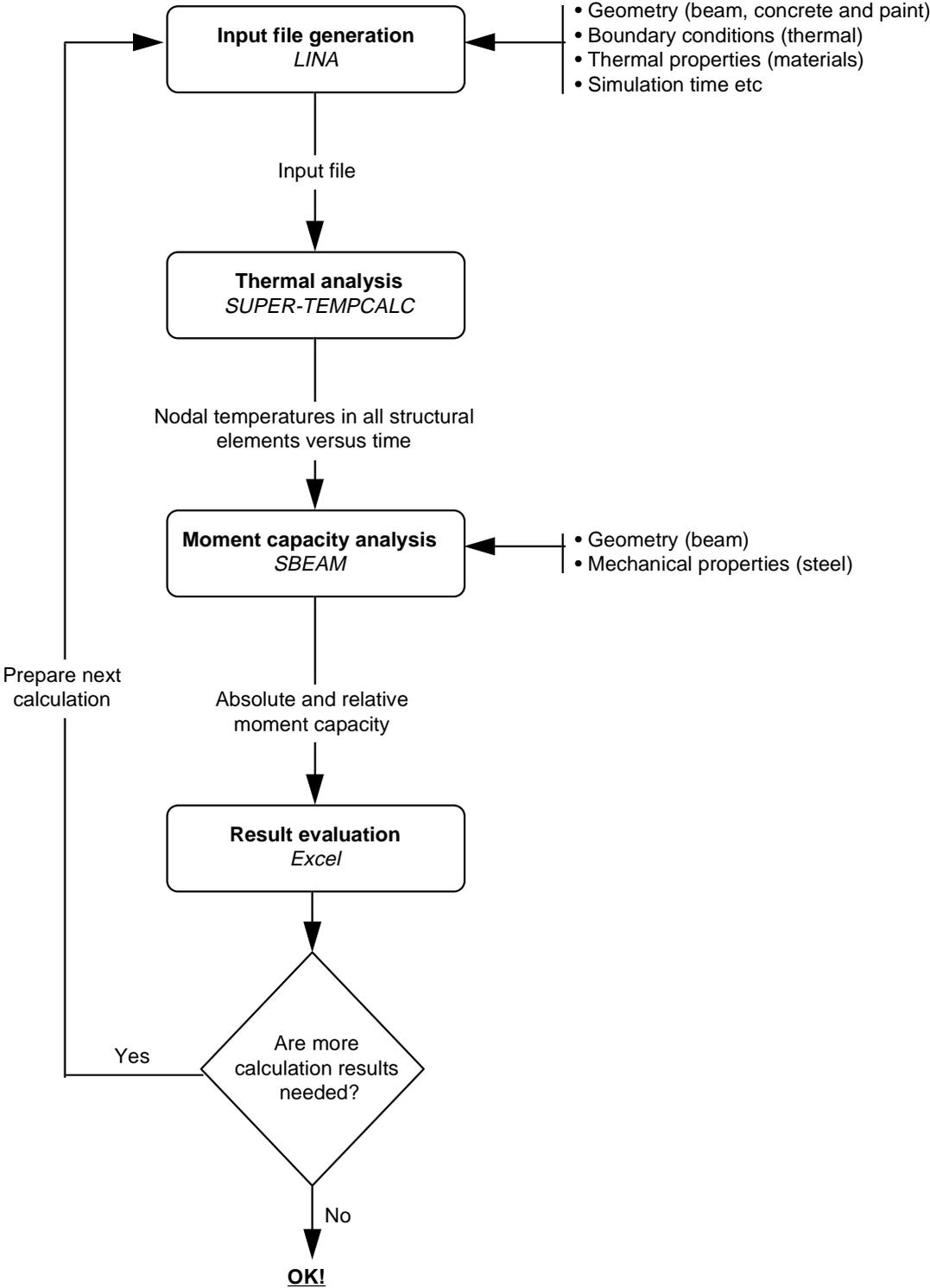
Figure 2.1 Method for calculation of moment capacity /18/.
