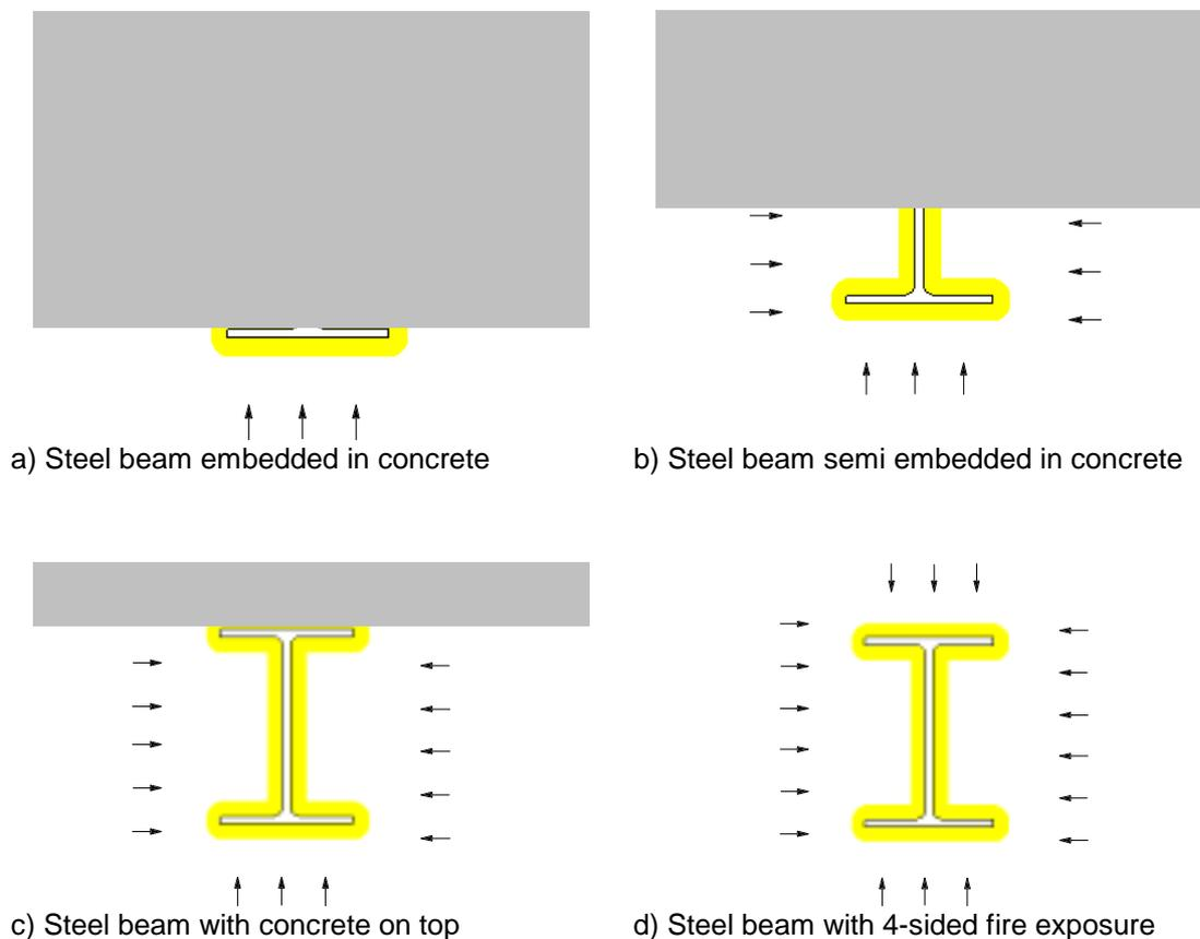
Figure 3.1 The four studied geometrical configurations.
