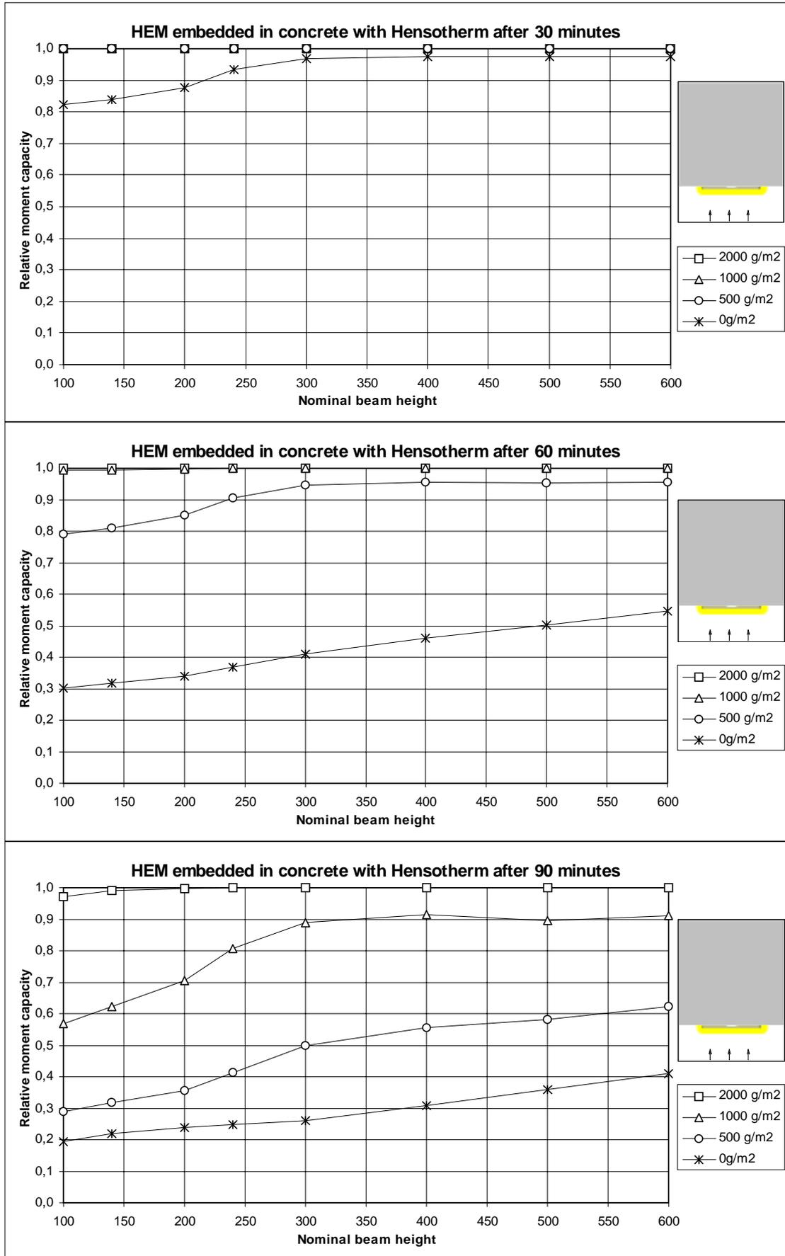
Figure 7.6 Relative moment capacity of HEM-beams embedded in concrete.
