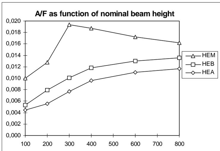
Figure 9.2b A/F as function of nominal beam height (m).
