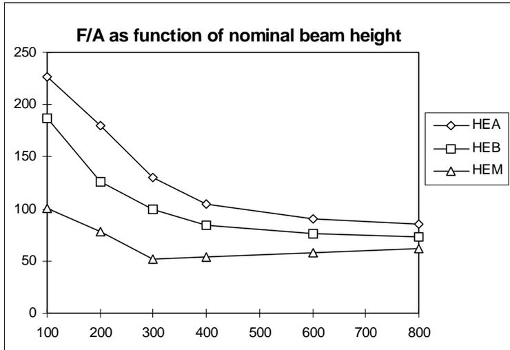
Figure 9.2a F/A as function of nominal beam height (m<sup>-1</sup>).
