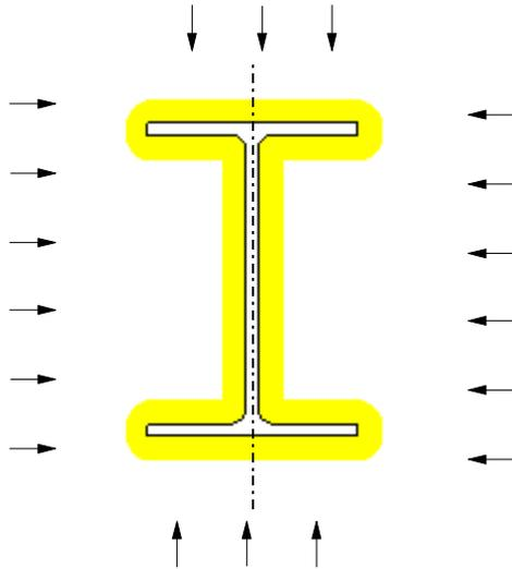
Figure 10.1 Steel beam with 4-sided fire exposure.
