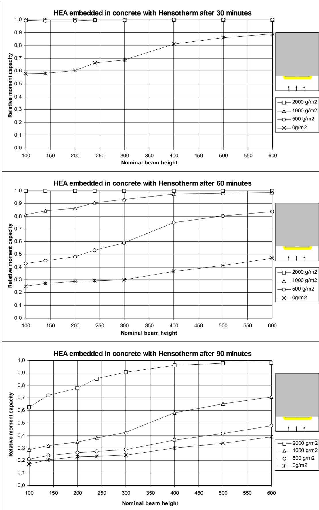
Figure 7.4 Relative moment capacity of HEA-beams embedded in concrete.
