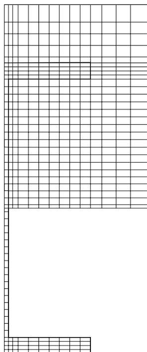
Figure 5.1 Grid of HEB 500 semi embedded in concrete.
