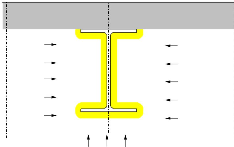
Figure 9.1 Steel beam with concrete on top.
