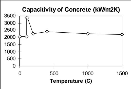
Figure 4.4 a) Capacity of concrete.
