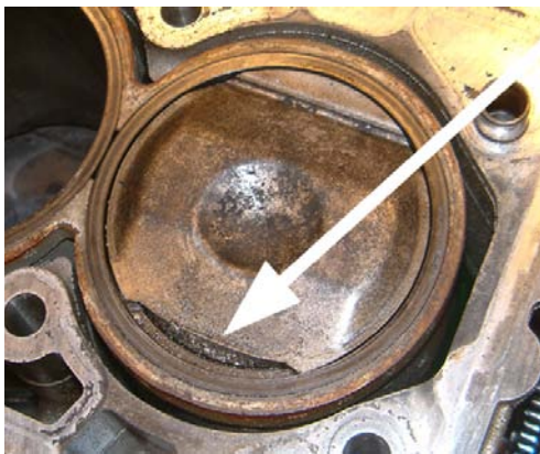
Figure 42: Damaged piston due to high PCP
