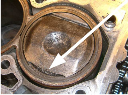
Figure 7: Damaged piston due to high PCP
