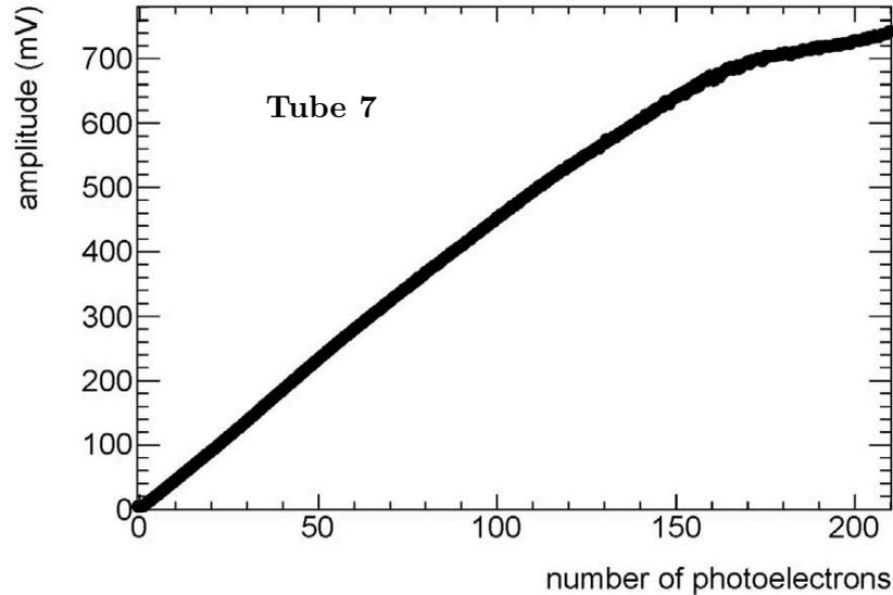
Figure 6.20: *The relationship between the amplitude recorded by the Flash analog-to-digital converter (FADC) and the charge measured by the QDC. The charge has been converted to the number of photo electrons produced in the photomultiplier. It can be seen that the FADC saturates when the number of photo-electrons exceeds a value of about 150.*
