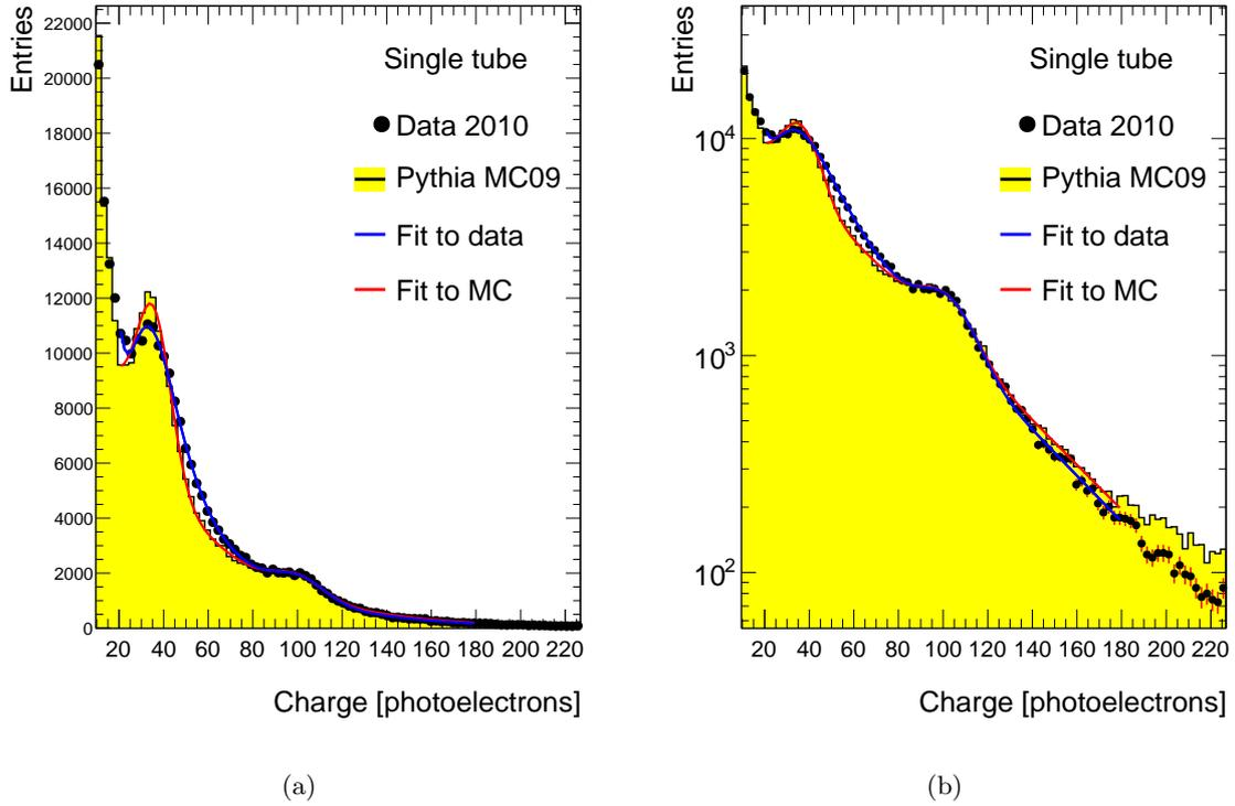
Figure 7.1: An example of a charge distribution of a single tube recorded by the QDC presented in linear scale (a) and logarithmic scale (b). Fits to both distributions have been superimposed on the plots.
