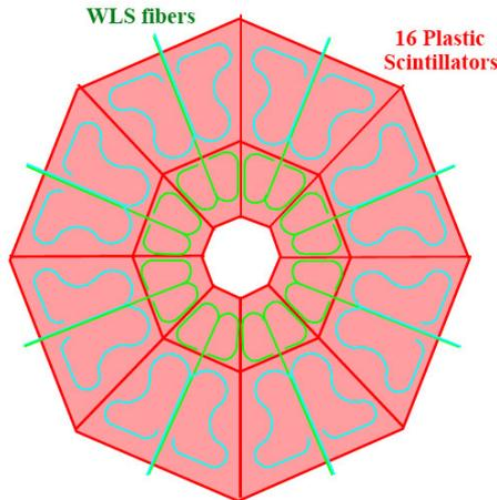
Figure 3.11: *schematic view of the MBTS disk configuration.*
