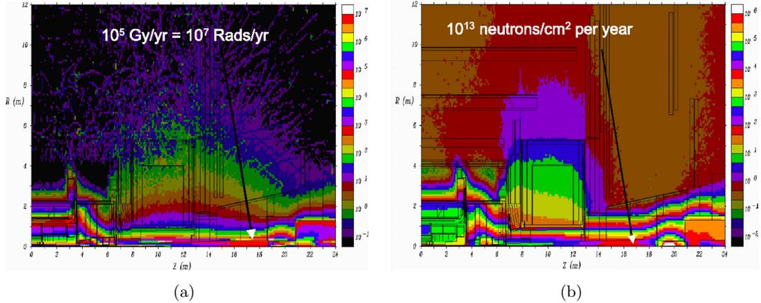
Figure 5.2: Simulation of the radiation levels in a full Atlas quadrant [71]. (a) Ionizing radiation (b) The neutron flux ( $E_n > 100\text{keV}$ ). The approximate dose in the region of LUCID is indicated in the plots.
