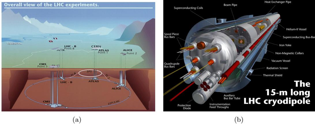
Figure 2.2: (a) Location of the LHC accelerator system [30] (b) Cross-section view of one of the LHC dipole magnets [30].
