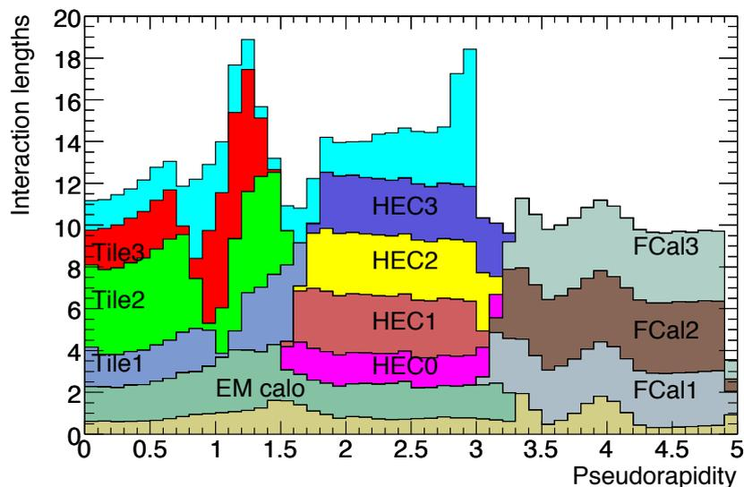
Figure 3.6: Cumulative amount of material, in units of interaction length, as a function of  $|\eta|$ . The contribution from the different parts of EM and hadronic calorimeters are indicated by the name of specific module [41]. Also shown for completeness is the total amount of material in front of the first active layer of the muon spectrometer (up to  $|\eta| < 3.0$ ).
