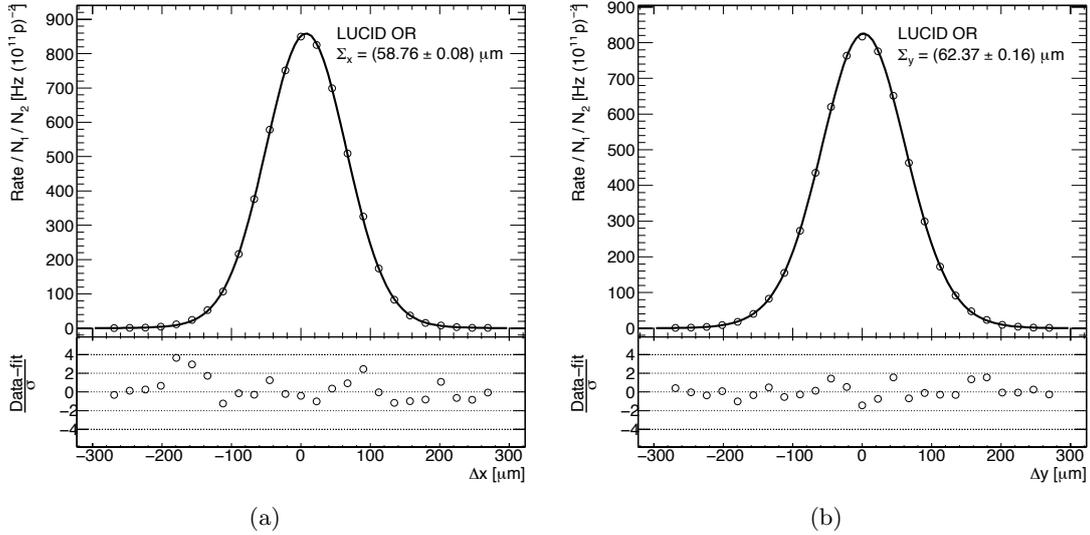
Figure 4.2: Results of a luminosity scan in the horizontal (a) and vertical plane (b) using the LUCID detector [65] [66]. The plots show the specific rate per  $10^{22}(\text{protons/bunch})^2$  as a function of beam separation. A Double Gaussian fit with a common mean is superimposed, together with the resulting values for  $\Sigma_x$  and  $\Sigma_y$  as defined in equation 4.9.
