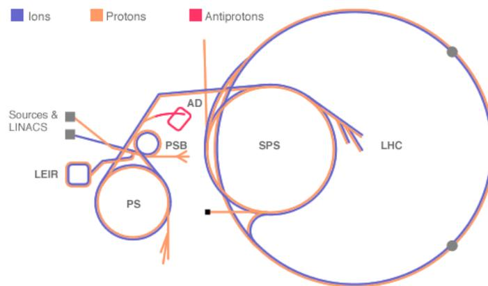
Figure 2.3: The LHC injector chain. Before the protons enter the LHC they are pre-accelerated in the following accelerators: (i) Linac, (ii) PSB (Booster), (iii) PS, (iv) SPS and finally (v) LHC.
