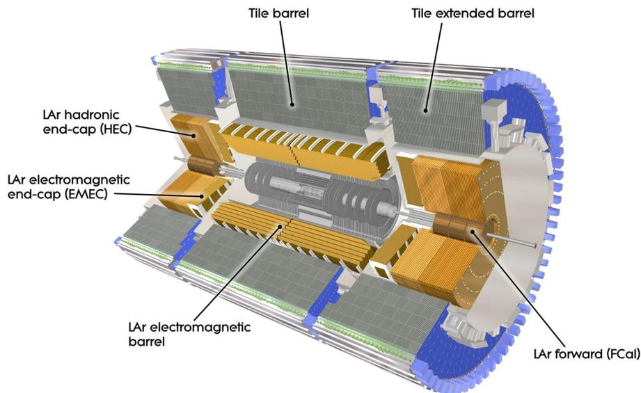
Figure 3.3: *Cut-away view of the ATLAS calorimeter system [30].*
