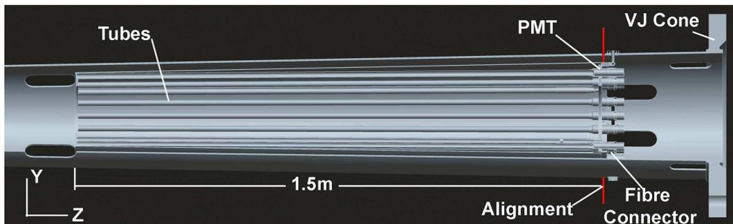
Figure 5.3: Schematic side view of a LUCID module.
