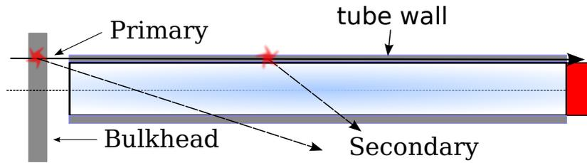
Figure 6.8: Sketch of a primary particle interacting with the detector material and thereby creating secondaries.
