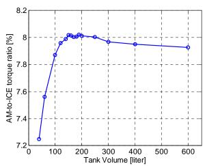
Figure 30 AM usage ratio as a function of tank volume for the FIGE drive cycle
