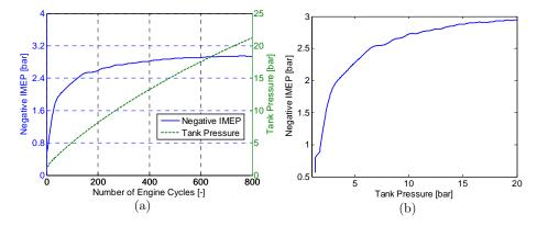
Figure 43 (a) Negative IMEP and mean tank pressure during transient compressor mode operation as a function of engine cycle number, (b) Negative IMPE as a function of mean tank pressure. Engine speed = 600 rpm.
