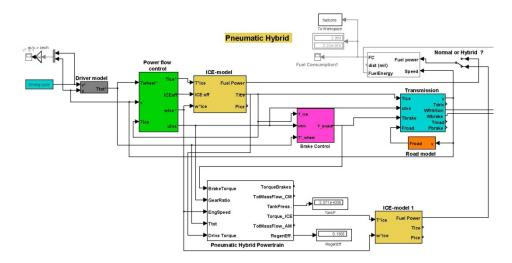
Figure 28 Top level of the pneumatic hybrid bus model
