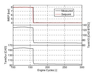
Figure 12 (Negative) Load step from 8 to 4 bar IMEP at a tank pressure of 10 bar
