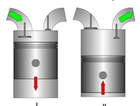
Figure 1 Illustration of Compressor Mode. I) Intake of fresh air, II) Compression of air and pressure tank charging.
