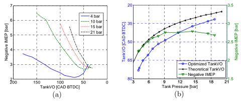
Figure 45 Steady-state optimization of the compressor mode at an engine speed of 600 rpm; (a) Negative IMEP as a function of TankVO for different tank pressures; (b) Optimal TankVO and corresponding negative IMEP as a function of tank pressure.
