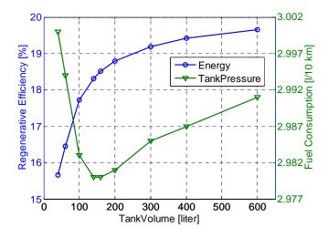
Figure 19 Regenerative efficiency and fuel consumption as a function of tank volume
