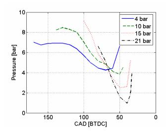
Figure 18 Pressure difference between maximum incylinder pressure and maximum tank pressure as a function of valve opening during optimization of CM at various tank pressures and an engine speed of 900 rpm.
