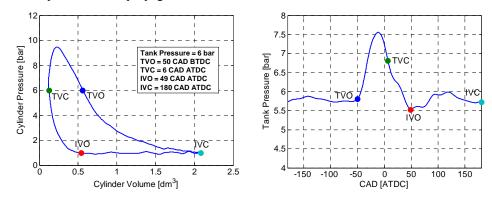
Figure 4 PV-diagram of the cylinder pressure (left) and tank pressure (right) of one CM cycle at a tank pressure of 6 bar and an engine speed of 600 rpm
