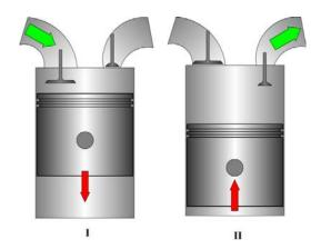
Figure 1 Illustration of Compressor Mode. I) Intake of fresh air, II) Compression of air and pressure tank charging.
