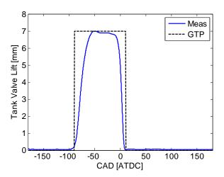
Figure 22 Tank valve lift profiles, measured and simulated.
