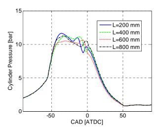
Figure 32 Cylinder pressure obtained during steadystate CM operation for various tank hose lengths vat a tank pressure of about 9.5 bar
