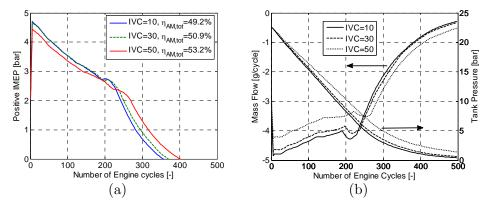
Figure 90 Transient air-motor operation for three different IVC at an engine speed of 600 rpm; (a) Positive IMEP, (b) Mass flow and tank pressure.
