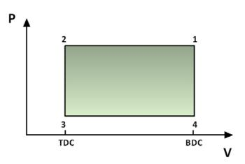
Figure 31 PV-diagram of maximum achievable engine load during on engine cycle of CM operation
