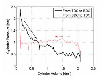
Figure 21 PV-diagram illustrates why IMEP is below 0 bars at some point during AM.
