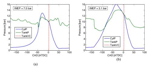
Figure 24 Cylinder and tank pressure as a function of CAD at a mean tank pressure of 10 bar and at a TankVO of 50 (a) and 140 (b) CAD BTDC. Engine speed = 600 rpm.
