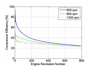
Figure 24 Total compressor efficiency as a function of engine revolutions during CM at three different engine speeds.
