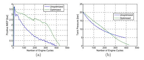
Figure 79 Comparison of transient air-motor operation with unoptimized and optimized valve timings: (a) Negative IMEP as a function of engine cycle number; (b) Tank pressure as a function of engine cycle number.
