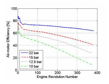
Figure 25 Total air-motor efficiency as a function of engine revolutions during CM at various tank pressures and an engine speed of 600 rpm.
