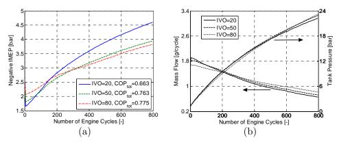
Figure 66 Transient compressor mode operation for three different IVO at an engine speed of 600 rpm; (a) Negative IMEP, (b) Mass flow and tank pressure.
