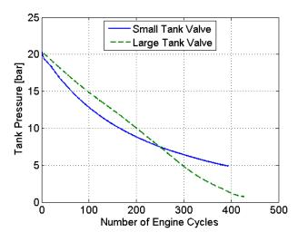
Figure 31 Mean tank pressure for two different valve geometries at an engine speed of 600 rpm
