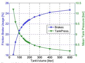
Figure 27 Friction brake usage and mean tank pressure as a function of tank volume for the FIGE drive cycle
