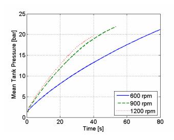
Figure 10 Mean tank pressure as a function of time for three different engine speeds.
