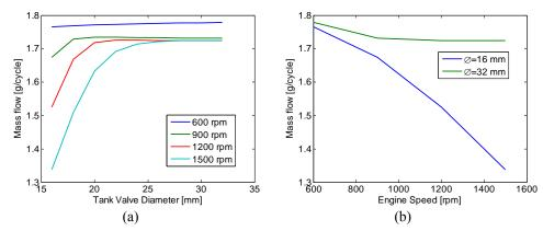
Figure 11 (a) Mass flow of compressed air into the tank as a function of tank valve diameter for various engine speeds, (b) Mass flow of compressed air into the tank as a function of engine speed for two different tank valve diameters. Tank pressure = 10 bar
