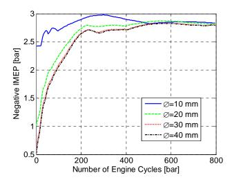
Figure 30 Negative IMEP obtained during transient CM operation as a function of engine cycle number at various tank valve diameters
