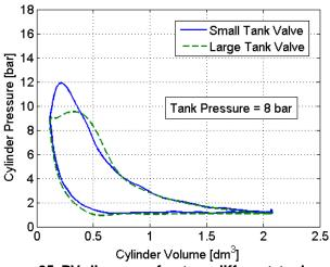
Figure 25 PV-diagrams for two different tank valve diameters at a tank pressure of 8 bars
