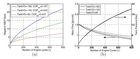
Figure 61 Transient compressor mode operation for three different TankVO at an engine speed of 1200 rpm; (a) Negative IMEP, (b) Mass flow and tank pressure.
