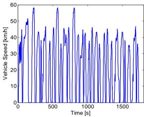
Figure 5 Vehicle speed during the Braunschweig driving cycle
