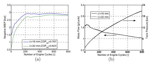
Figure 57 Transient compressor mode operation for two different valve setups at an engine speed of 600 rpm; (a) Negative IMEP, (b) Mass flow and tank pressure.
