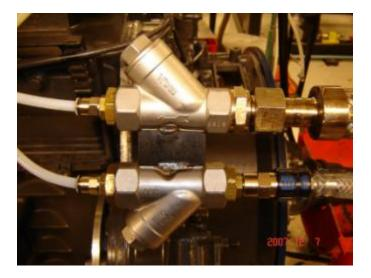
Figure 6 Pressurized air switching system built up by two check-valves
