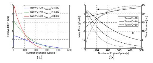
Figure 87 Transient air-motor operation for three different TankVC at an engine speed of 600 rpm; (a) Positive IMEP, (b) Mass flow and tank pressure.
