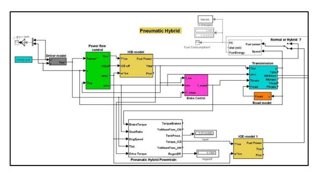
Figure 3 Top level of the pneumatic hybrid bus model
