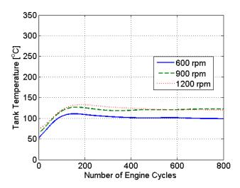
Figure 19 Pressure tank temperature as a function of engine cycle number at three different engine speeds
