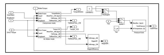
Figure 4 The Pneumatic hybrid specific subsystem
