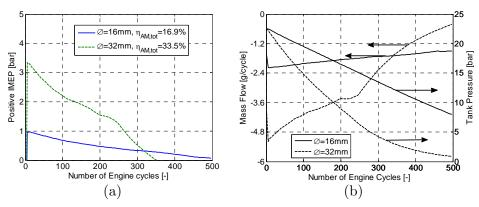
Figure 85 Transient air-motor operation for two different valve setups at an engine speed of 1200 rpm; (a) Positive IMEP, (b) Mass flow and tank pressure.
