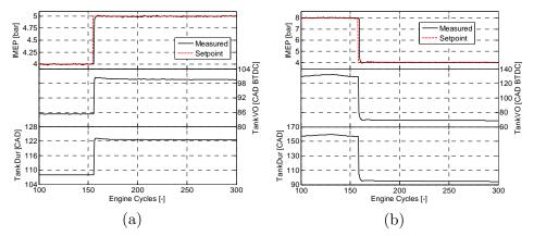
Figure 70 Closed loop process response to a set point change in IMEP during compressor mode operation at a steady-state tank pressure; (a) Positive set point change from 4 to 5 bar, tank pressure=8 bar (b) Negative set point change from 8 to 4 bar, tank pressure=10 bar.
