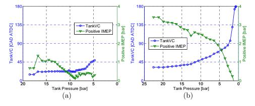
Figure 78 TankVC and corresponding positive IMEP as a function of tank pressure; (a) Theoretically calculated TankVC, (b) TankVC based on results from optimized compressor mode
