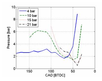
Figure 17 Pressure difference between maximum incylinder pressure and maximum tank pressure as a function of valve opening during optimization of CM at various tank pressures and an engine speed of 600 rpm.
