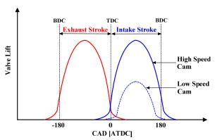
Figure 15 Illustration of two-step cam profile switching
