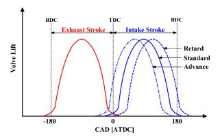
Figure 13 Illustration of inlet valve cam phasing
