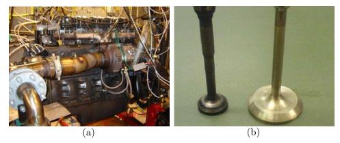
Figure 34 (a) The modified Scania D12 Diesel engine. The operating cylinder is to the left in the picture; (b) Picture illustrating the difference between the "small tank valve" ( $\emptyset=16~\mathrm{mm}$ ) and the "large tank valve" ( $\emptyset=28~\mathrm{mm}$ ).
