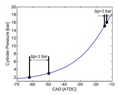
Figure 6 Illustration of how the change in CAD for a change in pressure by 1 bar changes with increasing pressure.
