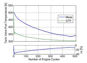
Figure 24 Tank valve port temperature and corresponding relative error as a function of engine cycle number during transient AM simulation
