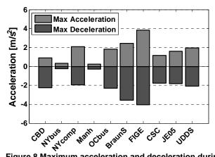
Figure 8 Maximum acceleration and deceleration during different drive cycles
