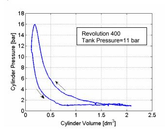
Figure 9 PV-diagram from engine testing at engine revolution number 400 and an engine speed of 600 rpm.
