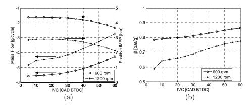
Figure 89 Various parameters as functions of IVC at a tank pressure of 20 bar; (a) Mass flow and IMEP, (b) β - the ratio between IMEP and mass flow shown in (a).
