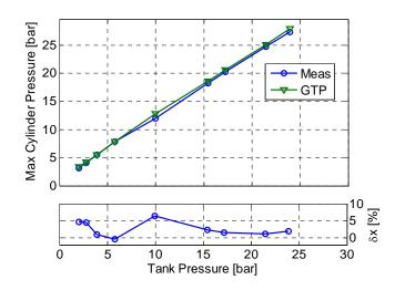
Figure 7 Maximum cylinder pressure and corresponding relative error as a function of tank pressure at an engine speed of 900 rpm
