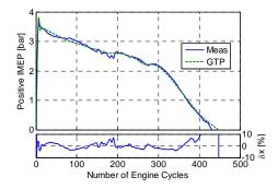
Figure 82 Positive IMEP and corresponding relative error as a function of engine cycle number during measured and simulated transient air-motor operation at an engine speed of 600 rpm.
