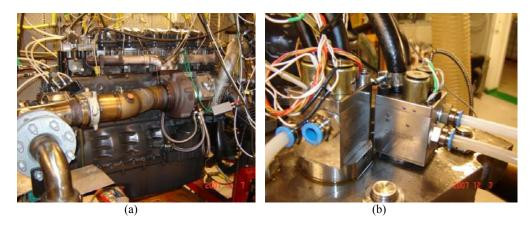
Figure 3 (a) The modified Scania D12 Diesel Engine. The cylinder modified for pneumatic hybrid operation is to the left in the picture. (b) The pneumatic valve actuators mounted on the Scania cylinder head
