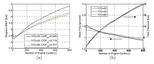
Figure 67 Transient compressor mode operation for three different IVO at an engine speed of 1200 rpm; (a) Negative IMEP, (b) Mass flow and tank pressure.
