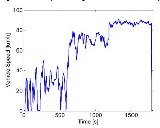
Figure 6 Vehicle speed during the FIGE drive cycle
