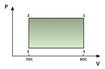
Figure 21 PV-diagram of maximum achievable engine load during on engine cycle of CM operation
