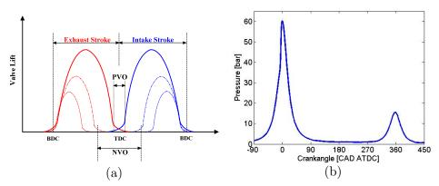
Figure 25 (a) Illustration of valve profiles for standard engines (solid lines) and for engines utilizing different degrees of NVO (dashed lines), (b) Pressure trace from an engine running with HCCI combustion and a NVO of 100 CAD
