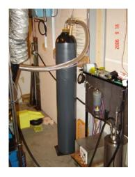
Figure 4 The pressure tank connected to the cylinder head by metal tubing.
