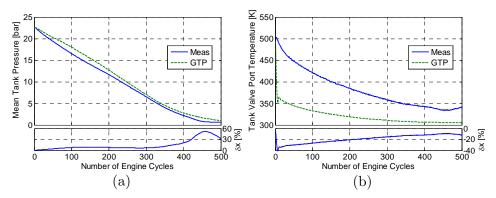
Figure 83 Mean tank pressure (a) and tank valve port temperature (b) together with corresponding relative error as a function of engine cycle number during measured and simulated air-motor mode operation at an engine speed of 600 rpm.
