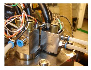
Figure 2 The pneumatic valve actuators mounted on the Scania cylinder head
