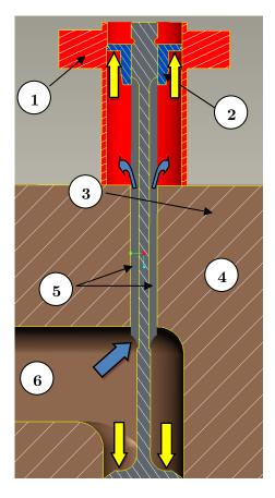
Figure 36  $\,$  A simple cross-section illustration of the pneumatic valve spring arrangement mounted on the cylinder head
