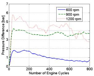
Figure 20 Pressure difference between maximum incylinder pressure and maximum pressure after the tank valve (port pressure) as a function of engine cycle number at various speeds. Tank valve with small diameter was used during this test.
