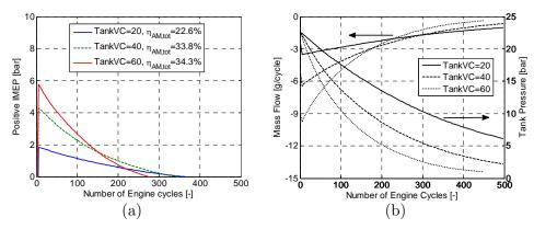
Figure 88 Transient air-motor operation for three different TankVC at an engine speed of 1200 rpm; (a) Positive IMEP, (b) Mass flow and tank pressure.
