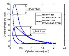
Figure 42 PV-diagram of two engine cycles at a tank pressure of 4 and 12 bar, respectively, illustrating the difference in cylinder pressure overshoot between early and late TankVO.
