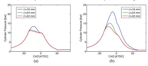
Figure 9 Cylinder pressure for various tank valve diameters at the engine speeds 600 rpm (a) and 1500 rpm (b). Tank pressure = 10 bar.
