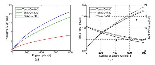
Figure 14 Various parameters as a function of engine cycles for three different TankVO at an engine speed of 600 rpm, (a) Negative IMEP, (b) Mass flow and tank pressure.
