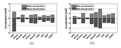
Figure 31 Acceleration and deceleration during the different drive cycles; (a) Mean acc/dec, (b) Maximum acc/dec.
