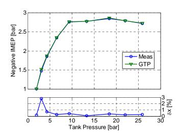
Figure 4 Negative IMEP and corresponding relative error as a function of tank pressure at an engine speed of 600 rpm
