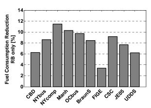
Figure 19 Fuel consumption reduction achieved only with regenerative braking for the different drive cycles (RB = Regenerative Braking)
