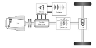
Figure 4 Illustration of a parallel hybrid drivetrain [19]
