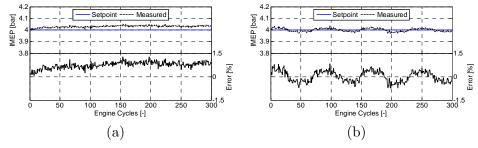
Figure 72 IMEP and the control error during steady state operation with only a feedforward controller (a) and with both PID and feedforward controller (b).
