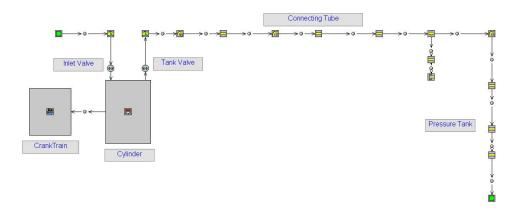
Figure 27 GT-Power model of the Scania single-cylinder engine
