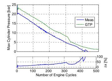
Figure 21 Maximum cylinder pressure and corresponding relative error as a function of engine cycle number during transient AM simulation
