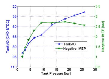
Figure 11 Optimized TankVO timing and corresponding negative IMEP during CM optimization as a function of tank pressure for the large tank valve setup at an engine speed of 600 rpm
