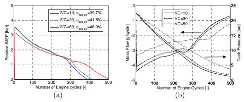
Figure 91 Transient air-motor operation for three different IVC at an engine speed of 1200 rpm; (a) Positive IMEP, (b) Mass flow and tank pressure.
