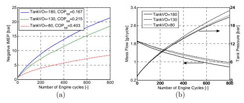
Figure 60 Transient compressor mode operation for three different TankVO at an engine speed of 600 rpm; (a) Negative IMEP, (b) Mass flow and tank pressure.
