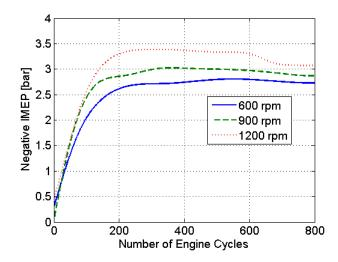
Figure 15 Negative IMEP during optimal CM as a function of engine cycle number at three different engine speeds for the tank valve setup
