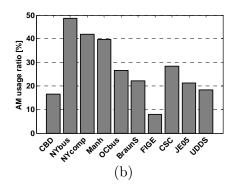
Figure 98 (a) Fuel consumption reduction achieved with and without (w/o) regenerative braking for the different drive cycles, (b) Air-motor mode usage ratio for the different drive cycles.
