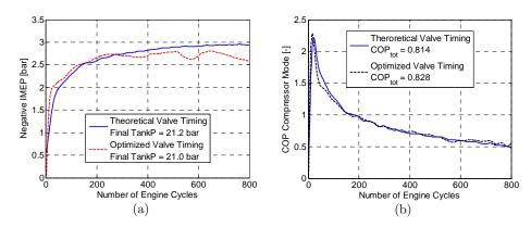
Figure 46 Comparison of transient compressor mode operation with theoretical and optimized valve timings: (a) Negative IMEP as a function of engine cycle number; (b) COP as a function of engine cycle number.
