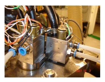
Figure 4 The pneumatic valve actuators mounted on the Scania cylinder head
