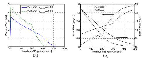
Figure 84 Transient air-motor operation for two different valve setups at an engine speed of 600 rpm; (a) Positive IMEP, (b) Mass flow and tank pressure.
