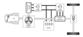
Figure 5 Illustration of a power-split hybrid drivetrain [19]
