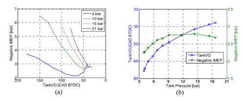
Figure 7 Steady-state optimization of the Compressor Mode at an engine speed of 600 rpm;
