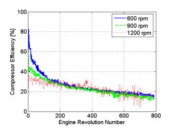
Figure 22 Compressor efficiency calculated for every engine revolution during CM at three different engine speeds.
