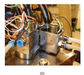
Figure 5 (a) The Engine used in the study. (b) The pneumatic valve actuators mounted on top of the modified Scania cylinder head
