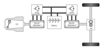
Figure 3 Illustration of a series hybrid drivetrain [19].
