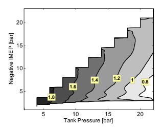
Figure 7 Mass flow rate (g/cycle) in to the tank as a function of both negative IMEP (2-sroke scale) and tank pressure during Compressor Mode.
