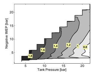
Figure 11 Mass flow rate (g/cycle) in to the tank as a function of both negative IMEP (2-stroke scale) and tank pressure during Compressor Mode.
