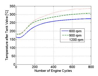
Figure 18 Temperature after tank valve (port temperature) as a function of engine cycle number at three different engine speeds
