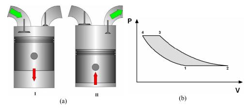
Figure 1 (a) Illustration of Compressor mode, I – intake of fresh air, II – Compression of air and pressure tank charging, (b) Illustration of the idealized PV-diagram of one Compressor Mode cycle
