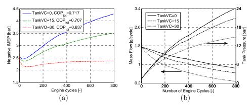
Figure 64 Transient compressor mode operation for three different TankVC at an engine speed of 1200 rpm; (a) Negative IMEP, (b) Mass flow and tank pressure.
