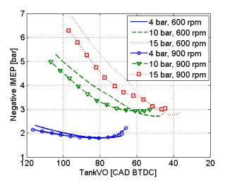
Figure 10 Negative IMEP obtained during steadystate CM as a function of TankVO for the large tank valve setup at various tank pressures for engine speeds of 600 and 900 rpm
