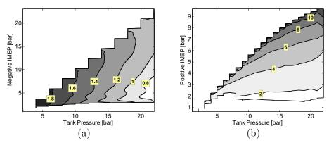
Figure 92 Performance maps illustrating the mass flow rate (g/cycle) across the tank valve as a function of both IMEP and tank pressure; (a) Compressor mode, (b) Air-motor mode
