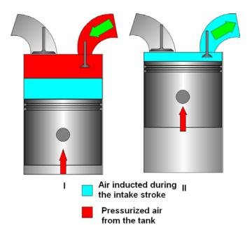
Figure 12 Illustration of blowdown of compressed air from the tank into the cylinder at an early tank valve opening.
