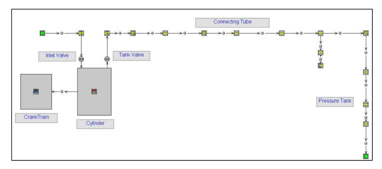
Figure 3 GT-Power model of the Scania single-cylinder engine.
