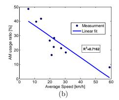
Figure 99 (a) Fuel consumption reduction as a function of air-motor mode usage ratio for the different drive cycles, (b) Air-motor mode usage ratio as a function of average speed for the different drive cycles.
