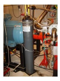
Figure 5 The pressure tank connected to the cylinder head by metal tubing
