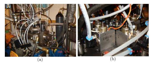
Figure 33 (a) The single-cylinder Scania diesel engine used in Paper I; (b) The pneumatic valve actuators mounted on the Scania cylinder head.
