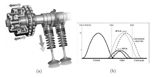
Figure 17 (a) Porsche VarioCam Plus system, (b) VarioCam Plus valve lift curves [67].
