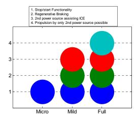
Figure 2 An illustration of the different hybridization levels and their characteristics
