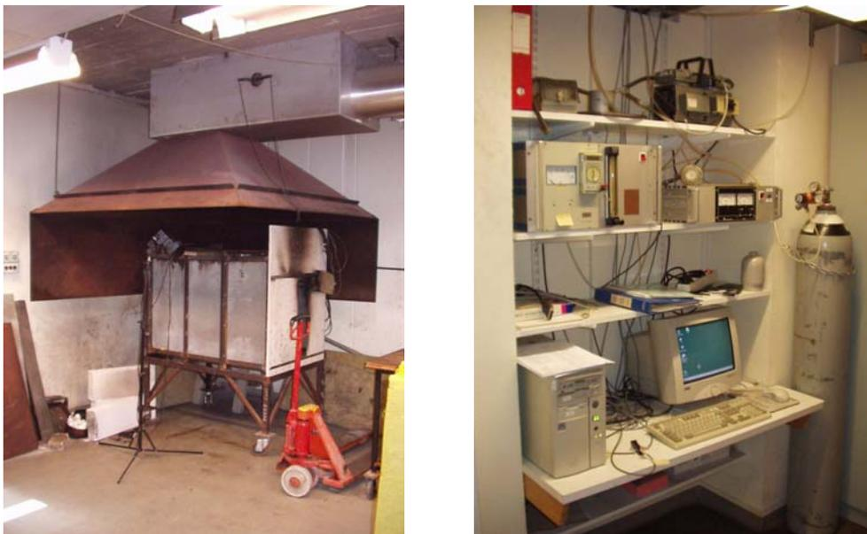
**figure 11.6** The furniture calorimeter at Brandteknik (left) and the computer used for logging the measurements (right)
