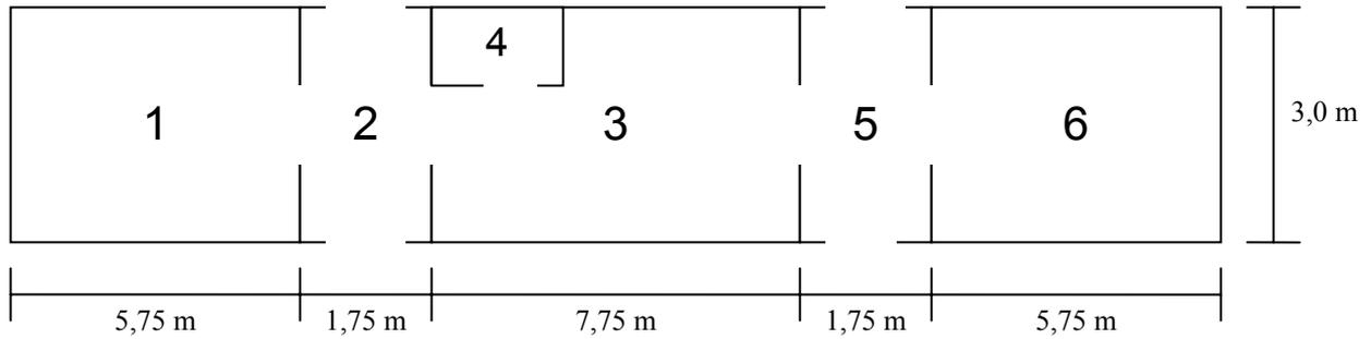
**figure 8.2** The model of the train Regina used in Hazard. This figure only gives a schematic overview of the compartments and openings used in the model and does not depict their relative sizes accurately.
