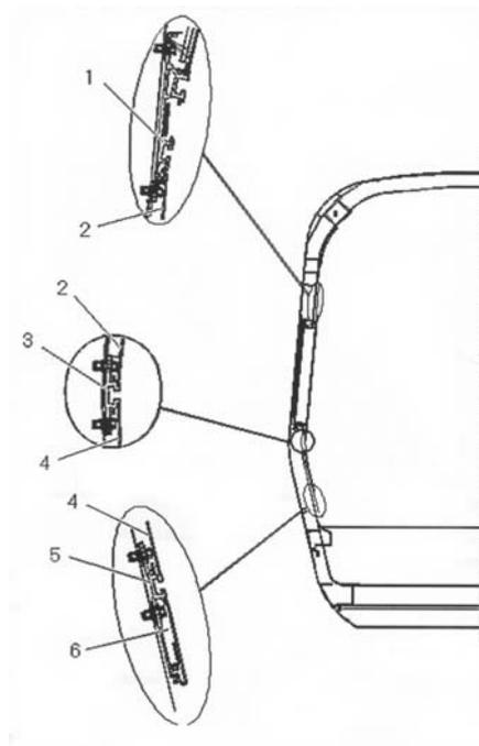
figure 4.4 A cross-section of the car-body's side wall
