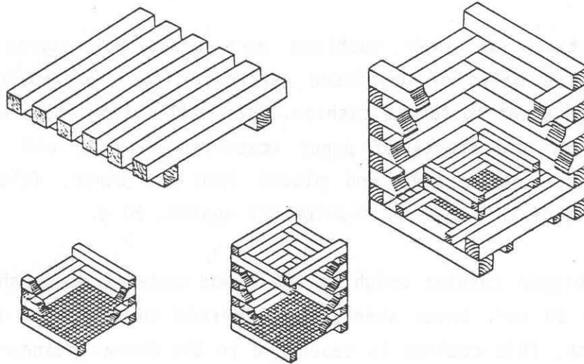
figure 11.1 Different crib ignition sources.
