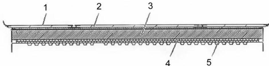
figure 4.5 A cross-section of the floor construction
