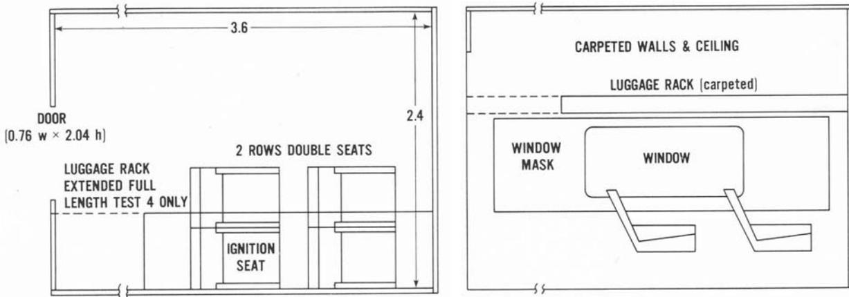
figure 3.2 The full-scale mock-up.
