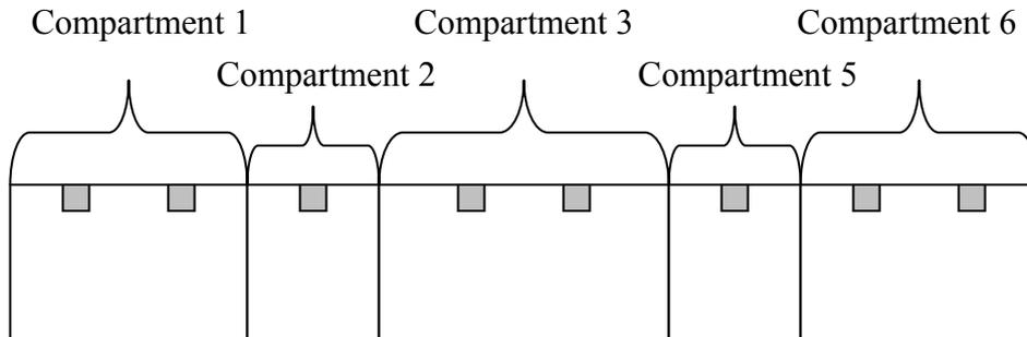
**figure 10.1** The placing of the water mist nozzles. One nozzle, which is not included in the figure, should be placed in compartment 4, i.e. the lavatory.
