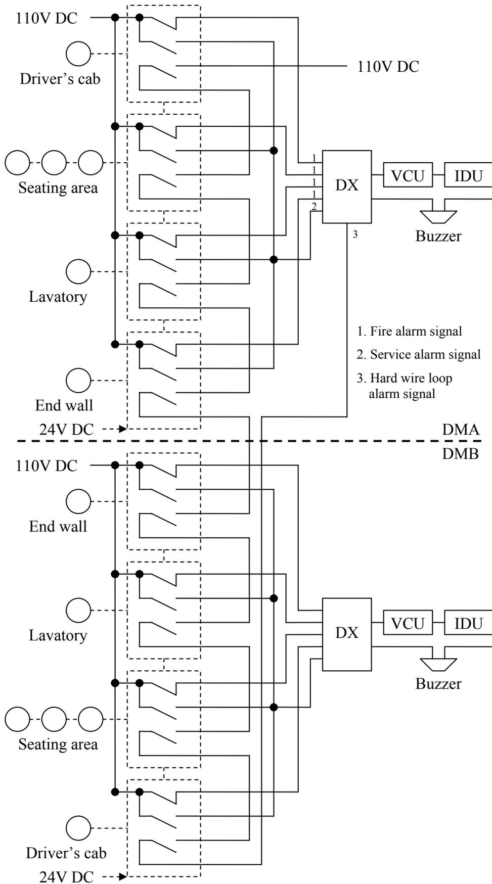
figure 4.9 Outline diagram of the detection system onboard Regina.
