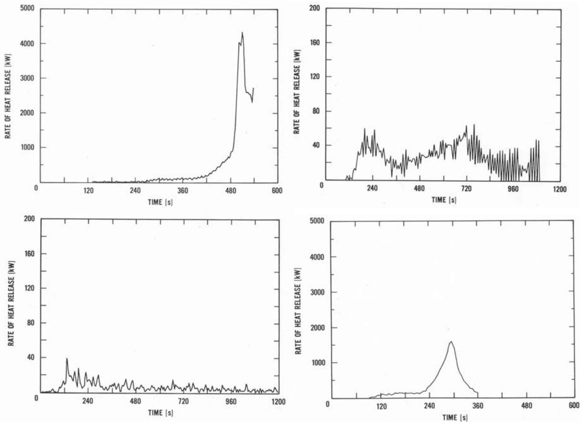
figure 3.3 Heat release rate curves for the full-scale tests (test 1 upper left, test 2 upper right, test 3 lower left and test 4 lower right).
