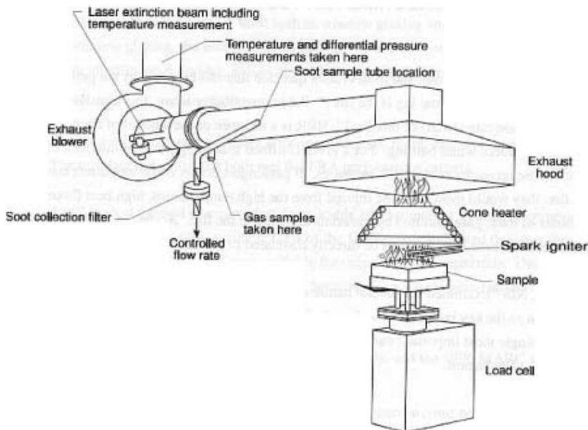
figure 11.5 The cone calorimeter.
