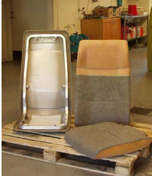
**figure 11.10** Passenger seat without the seat covering fabric.
