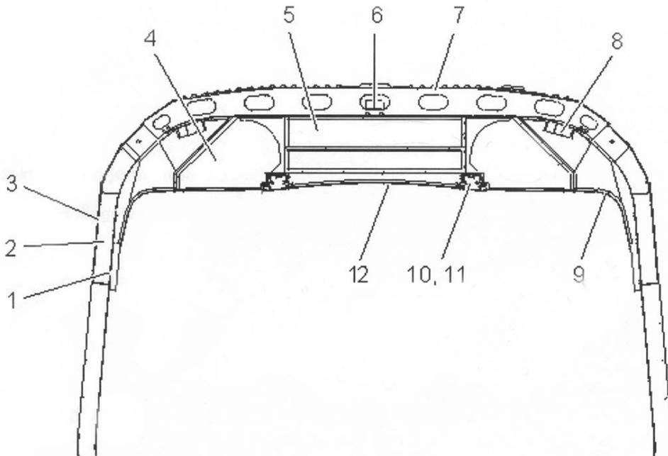
figure 4.3 A cross-section of the upper part of the car-body
