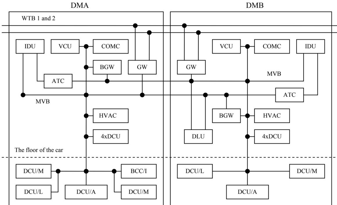
**figure 4.7** Simplified outline diagram of the MITRAC system and its connections to some non-MITRAC systems. The non-MITRAC systems included in this figure are the automatic train control system (ATC), brake gateway (BGW), door control unit (DCU), heating, ventilation and air conditioning system (HVAC) and data logging unit (DLU).
