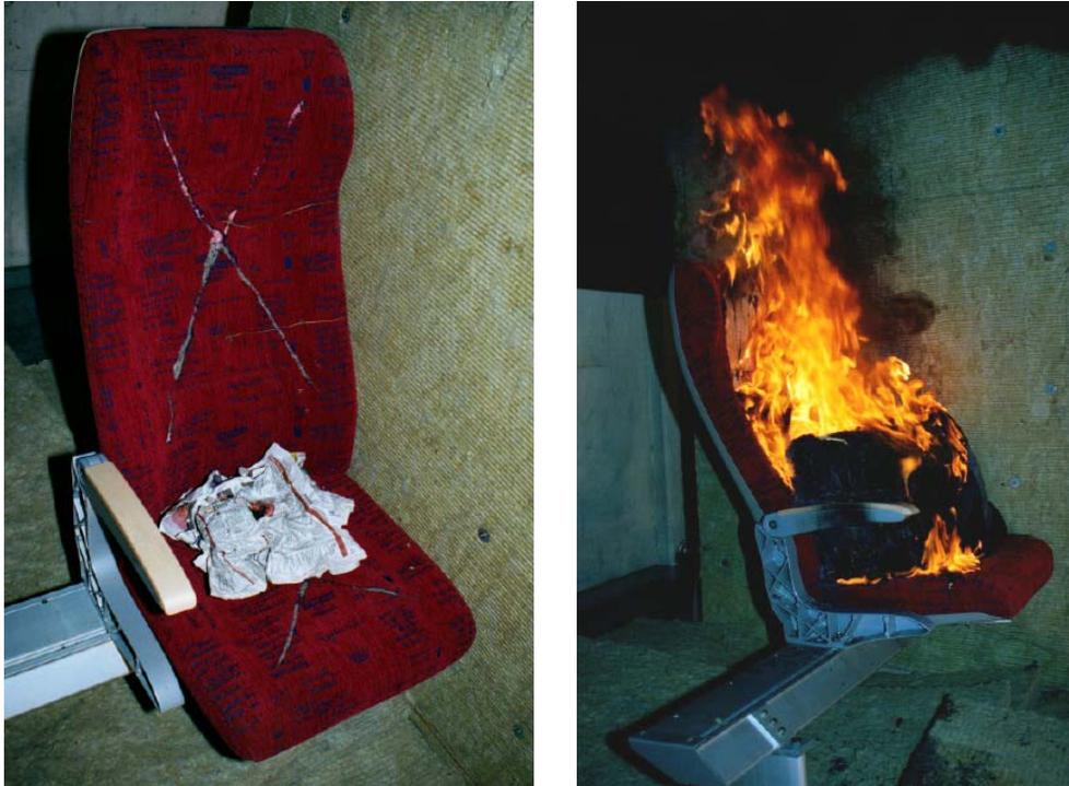
**figure 11.19** Vandalized seat with paper ball (left) and fully developed fire in the seat (right).
