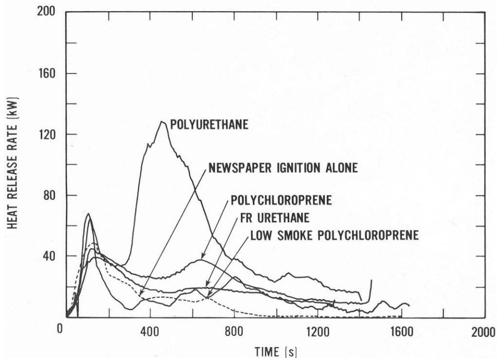
**figure 3.1** Heat release rate curves for the experiments with seats in the furniture calorimeter.
