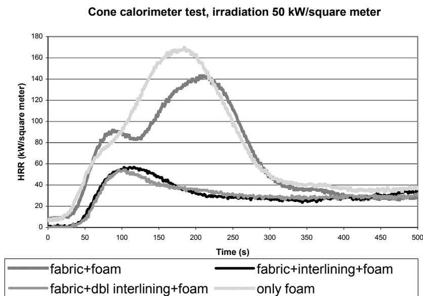
figure 11.12 Results from test of different cushions
