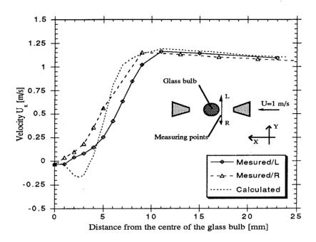
Figure 11 Comparison between the computed Ux velocity profile with FLOPAC and the experimentally determined profile using LDV for the worst orientation. The measurements were performed sidways to the air stream between the glass bulb and the upstream frame arm. L and R denotes values on different sides of the glass bulb. The free stream velocity U was 1 m/s.
