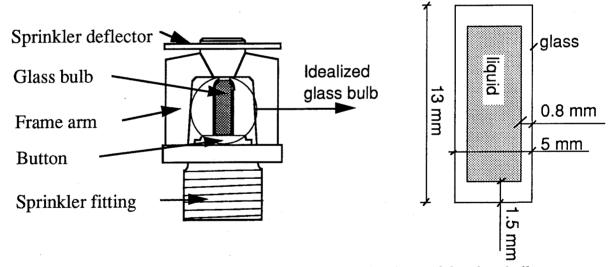
Figure 7 The Ø 5 mm sprinkler used in the test series. The shape of the glass bulb is simplified to a rectangular form to facilitate the calculations.
