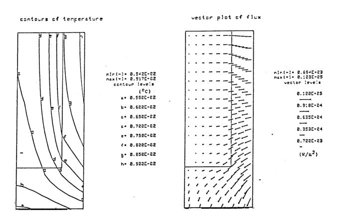
Figure 9 Temperature contours and heat flux vectors under plunge test conditions with heat losses to the sprinkler fitting. Tg=197, T1=30 °C, u=2.5 m/s. A quarter of the glass bulb is shown.
