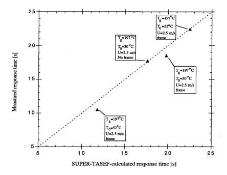
Figure 8 The measured response time versus calcualted response time with SUPER-TASEF in different plunge test situations.
