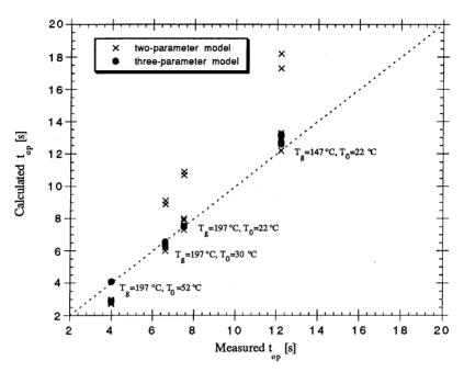
Figure 5 Calculated versus measured response time for a Ø 3 mm sprinkler in plunge tests under different test conditions. Both two- and three-parameter models were used.
