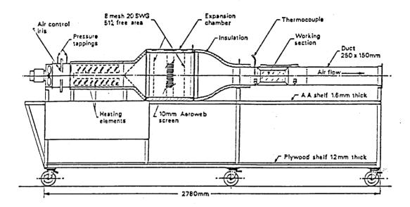
Figure 2 The wind tunnel used in the experiments presented in [1] was constructed in accordance with drawings from the Fire Ressearch Station in the UK.
