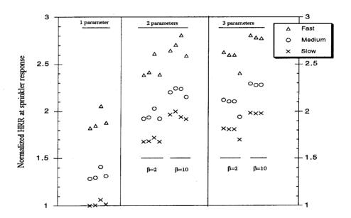
Figure 6 Normalized HRR at sprinkler response of a  $\emptyset$  3 mm sprinkler at a height of 3 m. The lowest HRR value obtained was used to normalize the other values. Distinction is made between calculations with parameters determined from ramp tests with  $\beta$ =10 °C/min and  $\beta$ =2 °C/min, respectively.
