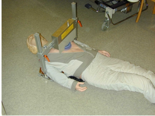
Fig 4. The first model used on patients at Lund University Hospital. This apparatus was the first to save the life of a patient after conventional CPR failed, see paper I.
