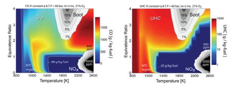
Figure 8 -  $NO_x$  and soot yield as function of equivalence ratio and temperature. The left figure is extended with the CO yield and the right figure is extended with the UHC yield. The yield is obtained from a homogeneous reactor simulation of an n-heptane/air mixture. The ambient pressure is 60 bar and the reaction time is 2.0 ms. [37]
