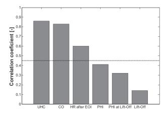
Figure 16 - Correlation coefficients between engine-out soot particle mass and different parameters. The UHC and CO emissions has the unit  $g/kg_{fuel}$ . The dashed line indicates the level that the correlation coefficient should exceed to be statistically significant, based on a one-tailed t-test with the confidence level of 95%.
