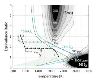
Figure 7 - Soot and NO production zones as function of temperature and equivalence ratio. The yield is obtained from a homogeneous reactor simulation of an n-heptane/air mixture during  $2.0\,$ ms. The adiabatic flame temperature is shown by the turquoise line at 21% ambient oxygen concentration, and the green line at 15% ambient oxygen concentration. [18]
