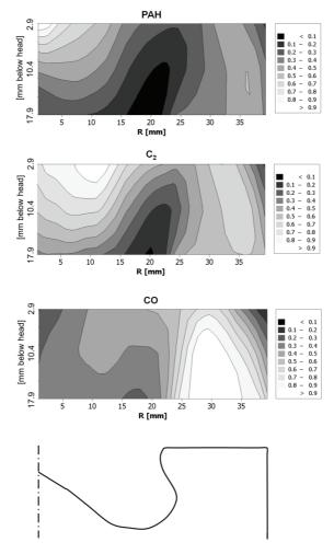
Figure 25 - Spatial distribution of PAH,  $C_2$ , and CO in the clearance volume 50 CAD ATDC. The contours are generated by averaging all measurements in the test matrix.
