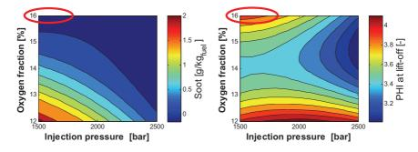
Figure 15 - Contour plot of  $\Phi$  at lift-off and engine-out soot emissions. The graphs show the combined effect of injection pressure and  $O_2$  mole fraction. The red oval indicates where the highest soot forming rate is expected.
