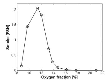
Figure 17 - Engine-out emissions of smoke as function of inlet  $\mathcal{O}_2$  mole fraction.
