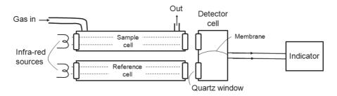
Figure 4 - NDIR gas analyzer. [23]
