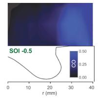
Figure 27 - Distribution of CO 50 CAD ATDC for the baseline load 3 bar IMEP $_{\rm g}$ . The  ${\rm O_2}$  mole fraction is 15% and the start of injection timing in CAD ATDC is indicated in the images.
