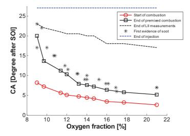
Figure 20 - Start of combustion, end of premixed combustion, time for the first soot appearance, and end of injection as function of inlet  $O_2$  mole fraction. All values expressed as CAD after SOI. The heat release is calculated using a volume trace according to Eq 28 and heat losses according to Eq:s 17, 18, and 19.
