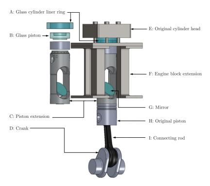
Figure 1 - Optical engine of Bowditch design. Items A, B, C, F, and G are added to achieve optical access to the combustion chamber while the rest are all-metal engine parts.
