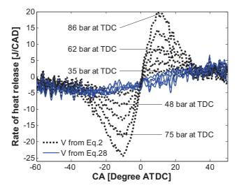
Figure 9 - Motored heat release rate traces for different pressure traces. The dotted curves are calculated with a volume trace according to Eq. 2 using a compression ratio that gives the true clearance volume for a TDC pressure of 34 bar. The solid curves are calculated with volume traces according to Eq. 28. The pressure at TDC are indicated for the black dotted curves.
