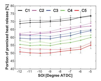
Figure 13 - Portion of heat release in the premixed combustion phase as a function of SOI for configuration 1 (C1) to C5 at 2.4 bar  $\mathrm{IMEP_g}$ . C1 is an all-metal engine and C2 to C5 are different set-ups of an optical engine. Higher configuration numbers are equal to more optical components. The deformations are considered for dashed curves but not for solid curves.
