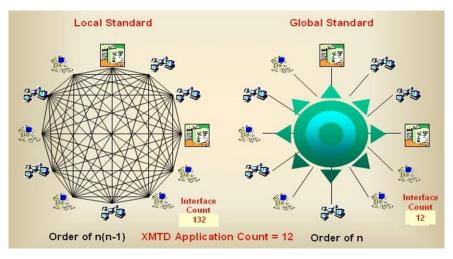
**Figure** 3.1 Calculation of interface-connections for local and global standards (BSharah, 2003).
