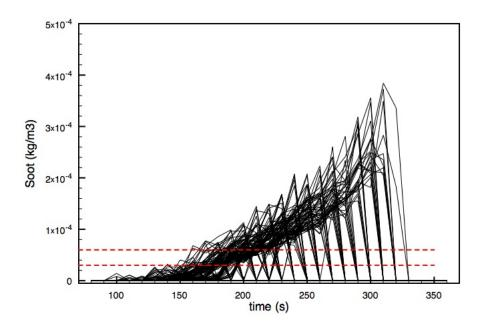
Figure 29. Soot concentration (kg/m³) for each person in the simulations for cable M
