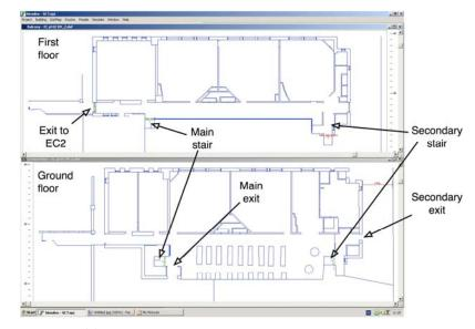
Figure 22. The geometry that was used in the evacuation scenarios (screen shot from SIMULEX)
