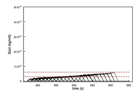
Figure 28. Soot concentration (kg/m³) for each person in the simulations for cable I
