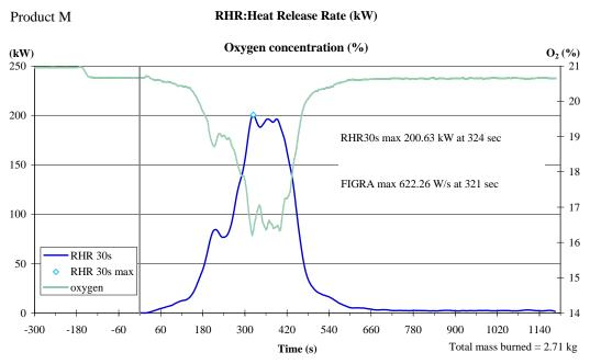
Figure 11. Heat release curves for cable M<sup>2,3</sup>
