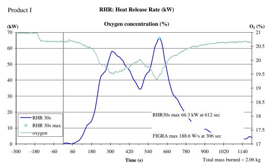
Figure 10. Heat release curves for cable I<sup>2,3</sup>
