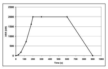
Figure 2. Example of a Design Fire
