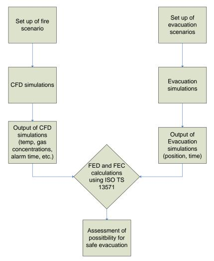
Figure 3. Schematic overview of the procedure
