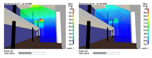
Figure 19. Comparison of temperatures at 600s between cable M (left) and cable I (right)
