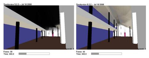
Figure 15. Comparison of soot concentration at 300s between cable M (left) and cable I (right)
