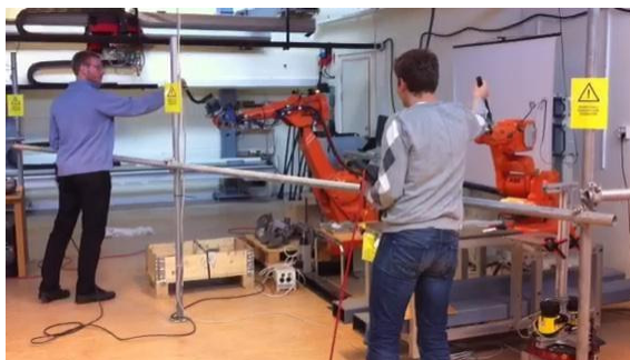
Figure 10.1 Lead-through of virtually connected robots.
