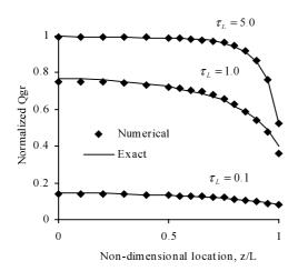
Fig. 6 Non-dimensional gas radiative flux along z direction on the cylinder wall. Note:  $Q_{gr} = q/\sigma T_g^4$ , z=0 at the middle height of the cylinder.
