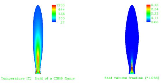
Fig. 3 Temperature and soot volume fraction distribution in a C3H6 flame
