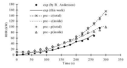
Fig.12 Calculated and measured heat release rates in the 1/3 scale scenario. The symbol (c) denotes using Cone data input method and (p) the pyrolysis model.
