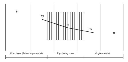
Fig. 10 Temperature solution grid and its refinement (Example with N = 5, M = 10, where N is the coarser grid number and M is the refined grid number in a coarser grid)
