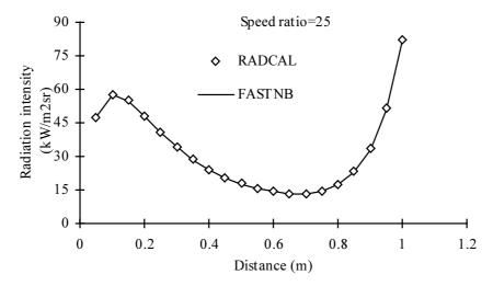
Fig. 9 Comparison of total intensities, for a path of parabolic minimum temperature and concentrations, with an even soot volume fraction of  $2.0 \times 10^{-6}$ . Note: speed ratio is defined as the CPU time required by RADCAL over the CPU time required by FASTNB.
