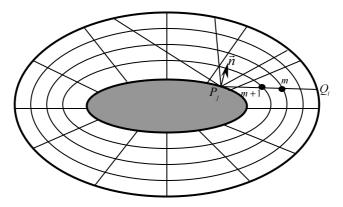
Fig. 4 Illustration of discrete transfer method
