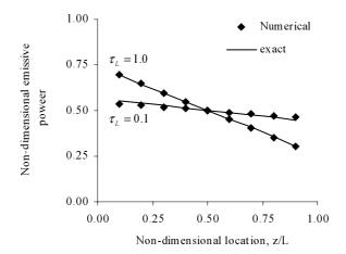
Fig. 5 Non-dimensional temperature distribution for radiative equilibrium between parallel plates. Note: z is the distance from a plate surface, the non-dimensional emissive power is defined as  $\frac{T^4-T_2^4}{T_1^4-T_2^4}$  and  $\tau_L$  is the optical thickness kL, where k is the absorption coefficient and L is the distance between plates.
