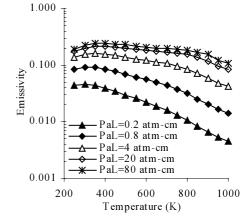
Fig. 8 Band absorption and emissivity of C2H2
