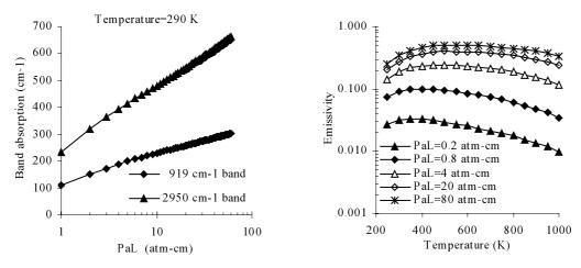
Fig. 7 Band absorption and emissivity of C3H6. Note: PaL is the pressure path length.
