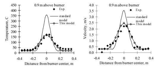
Fig. 2 Comparison of predicted and measured temperature and velocity profiles at 90 cm above a buoyant C3H6 diffusion flame
