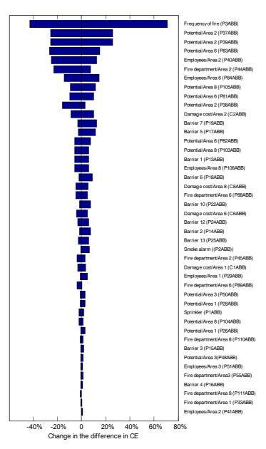
Figure 24 Tornado diagram showing the effect of epistemic uncertainty on the CE of the sprinkler alternative.
