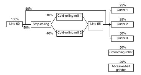
Figure 28 Flow of material within the cold-rolling mill.
