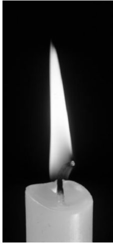
Figure 1.5: Laminar diffusion flame [57].
