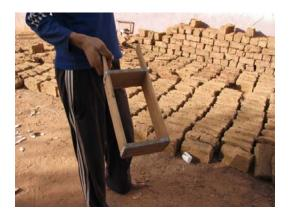
Figure 2.17 Moulds used in mud brick casting in the Dakhla oasis.
