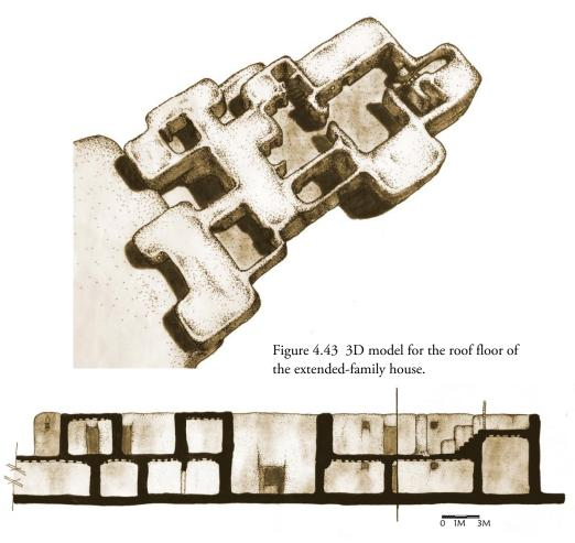
Figure 4.44 Section in the extended-family house showing internal heights.
