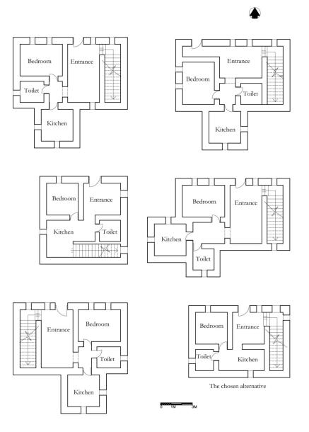
Figure 3.15 The figure shows the neo-desert vernacular model house alternatives which were designed by Balat locals. One of the alternatives was chosen for the construction phase and one of the rooms was built.
