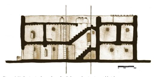
Figure  $4.40\,$  Section in the medium-family house showing internal heights.
