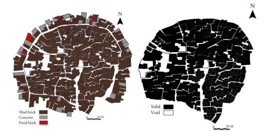
Figure 4.75 Edited map of current building materials for Balat showing the change to using concrete and fired bricks on the outskirt of the town.
