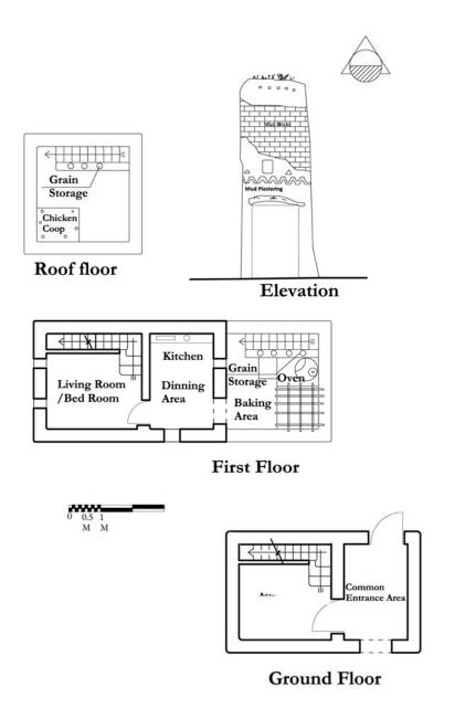
Figure 1.14 A sample of a mud brick house in the Dakhla oasis. Drawn during my site investigation in the early research stages.
