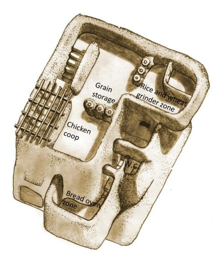
Figure 4.37~3D model of the small-family house showing roof floor functional spaces.
