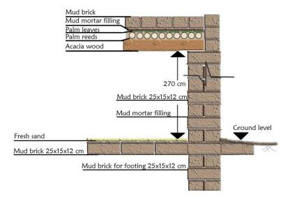
Figure 5.42 Cross section in a vernacular mud brick house in Balat to show the modification with comparison to the room of the neo-desert vernacular model house.
