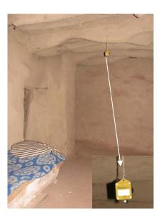
Figure 5.6 Indoor temperature measuring loggers in Balat.
