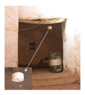
Figure 5.5 Outdoor temperature measuring loggers in Balat.
