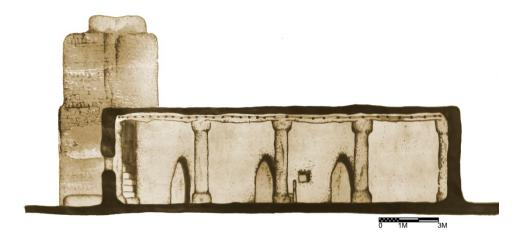
Figure  $4.72\,$  Section in the mosque showing the internal height and the proportions in comparison to the minaret.
