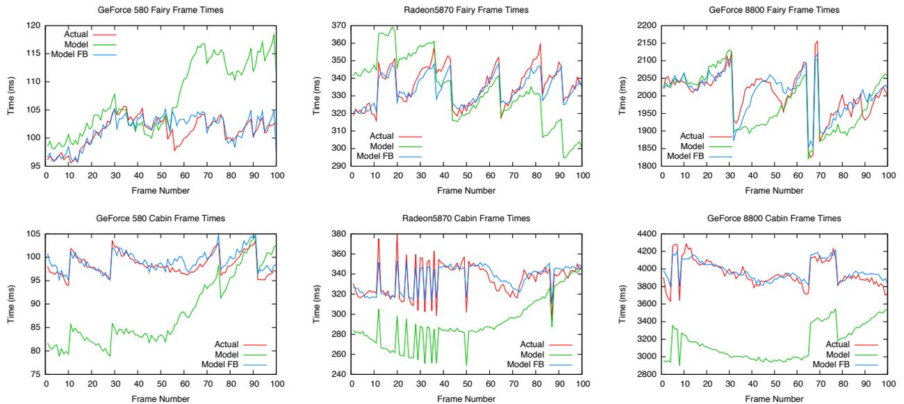
**Figure 5: Frame times for different GPUs and scenes for a 100 frame animation. The reference time for the graphs for the fairy scene on the top row are 100ms, 333ms and 2000ms, and for the cabin scene on the bottom row, they are 100ms, 333ms and 4000ms.**
