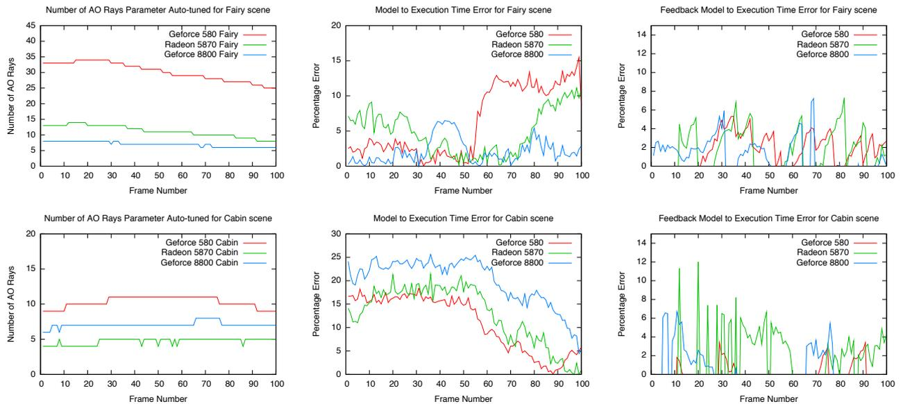
**Figure 8: Auto-tuned number of AO rays, and error for different GPUs and scenes over a 100 frame animation. The top row is for the fairy scene and the bottom row for the cabin scene. The two left graphs show the number of AO rays auto-tuned over the animation, the middle two graphs show the percentage error between the GPU model and actual execution time and the right two graphs show the percentage error between the GPU model and the outer loop feedback corrected model time.**
