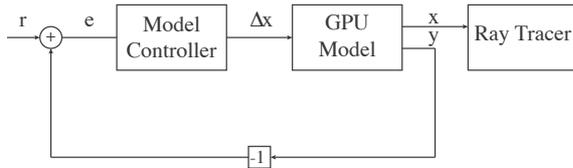
**Figure 1: Auto tuning the ray tracer using the GPU model and a feed forward controller.**
