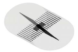
**Figure 4.5.** Illustration of the Delta<sup>4</sup> detector system, which consists of two orthogonal detector arrays in a cylindrical polymethyl methacrylate (PMMA) phantom. The detector spacing is 5 mm in the central and 10 mm in the distal part of each array.
