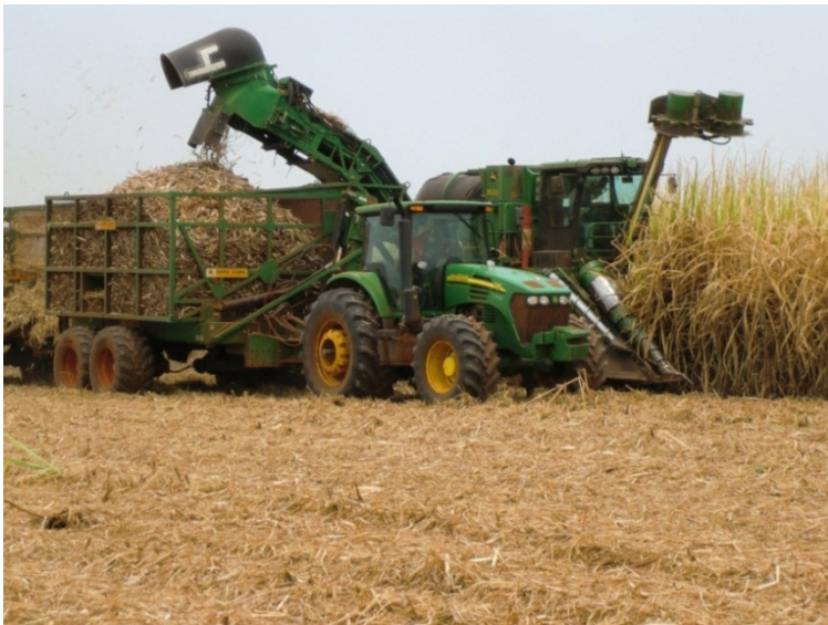
Figure 3.5. The harvester cuts the cane into short stubs
