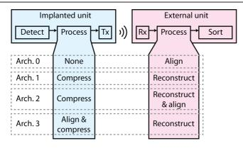
Figure 2: An illustration of the system architectures considered in the comparison. The "Tx" and "Rx" blocks refer to the wireless transmitter and receiver, respectively. In architecture 0 (the reference architecture) uncompressed spikes were transmitted, aligned and sorted. In architectures 1 to 3, spikes were compressed, reconstructed and sorted and in architectures 2 and 3, spike alignment was performed at different stages.
