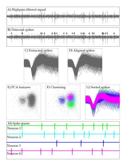
Figure 2.4: An illustration of the procedure of isolating spike trains from individual neurons in the highpass filtered signal. The procedure typically involves spike detection, spike alignment, feature extraction and clustering. In the example shown here, absolute value threshold detection, maximum absolute value alignment and principal component analysis are used for spike detection, alignment and feature extraction, respectively.
