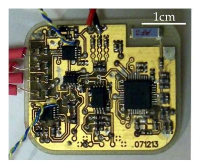
Figure 1: The dimensions of the first prototype of the wearable telemetry device are  $30 \times 37 \times 3 \text{ mm}^3$ . All components are mounted on the top side of the PCB. The analog amplifier is on the left and the nRF24E1 with it's peripheral components is on the right.
