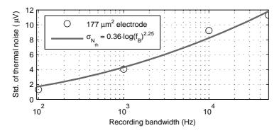
Figure 4: The standard deviation of thermal noise,  $\sigma_{N_{th}}$  at a temperature of 37°C fitted to a power law function ( $R^2 = 0.98$ ) of the logarithm of recording bandwidth  $f_B$  for an electrode of 177  $\mu m^2$  extrapolated from [20].
