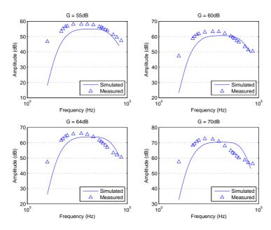
Figure 5: The amplitude of the amplifer transfer function at the four different gain settings.
