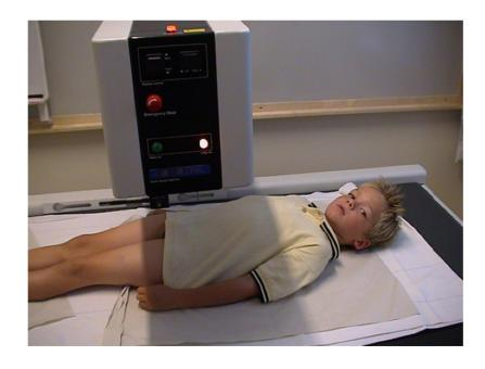
Fig. 10. The Lunar® DPX-L (DXA) apparatus Figure presented by courtesy of Christian Linden
