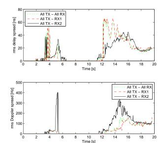
Fig. 7. Sc-1b: Time-varying rms delay spread (top) and time-varying rms Doppler spread (bottom) for scenario 2.
