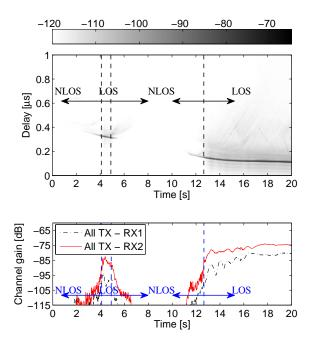
Fig. 3. Sc-1b: Averaged power delay profile (top) and channel gain of the strongest and weakest links among the  $4 \times 4$  MIMO links (bottom).
