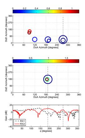
Fig. 4. Sc-1a: The azimuth direction-of-arrival (DOA) and azimuth direction-of-departure (DOD) estimates for the snapshots at time instant  $10.58\,\mathrm{s}$  (top) and  $17.56\,\mathrm{s}$  (middle), and the azimuth antenna gain of RX element-1 and element-2 (bottom) are shown. The color bar is representing the relative distance (m) w.r.t the LOS component such that the LOS component is at 0 m. The size of the circles depicts power carried by each MPC.
