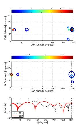
Fig. 5. Sc-1b: The azimuth direction-of-arrival (DOA) and azimuth direction-of-departure (DOD) estimates for the snapshots at time instant 13.51s (top) and 17.56s (middle), and the azimuth antenna gain of RX element-1 and element-2 (bottom) are shown. The color bar is representing the relative distance (m) w.r.t the LOS component such that the LOS component is at 0 m. The size of the circles depicts power carried by each MPC.
