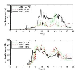
Fig. 6. Sc-1a: Time-varying rms delay spread (top) and time-varying rms Doppler spread (bottom) for scenario 1.
