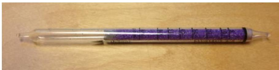
Figure 16. A test tube identical with the ones that was used to measure the gas concentration of acetic acid in the experiment.
