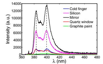
**Figure 8.7.** The background signals due to the fluorescence from the surfaces of different components in the experimental set-up resulting from illumination by the Ce excitation laser. Note that the intensities in this figure are not the same as the intensity in Figure 8.5 as the measurement conditions were different.
