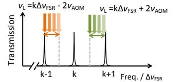
**Figure 4.2.** The discrete transmission lines of the ULE cavity (FSR of 3 GHz) and an illustration of the laser scanning range using the  $\pm 1$  orders of deflected beams from an AOM. One half of the FSR (indicated by the orange arrow) is covered by the  $+1$  order deflected beam, and the other half by the  $-1$  order deflected beam.
