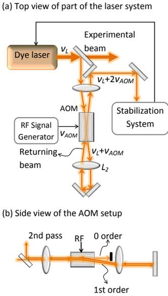
**Figure 4.1.** Setup used to tuning the frequency of the experimental beam while the laser is locked onto the stable cavity. It can be tuned within 1.5 GHz continuously using the first order deflected beam from the AOM.
