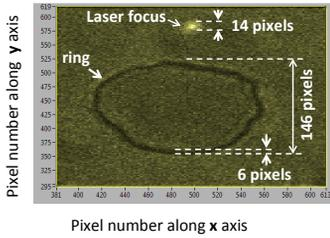
**Figure 4.9.** Image of the gold-coated plate showing an etched ring. In this measurement the focal length of  $L_f$  is 500 mm and the 20 $\times$  objective lens (effective focal length 9 mm) was used. Aberration correction was made.
