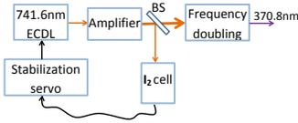
**Figure 5.1.** A stable 371 nm laser can be generated by frequency doubling a 741 nm laser that is locked to an  $I_2$  line. As a result of the frequency doubling efficiency is only a few percent, and a light amplifier is needed to increase the power.
