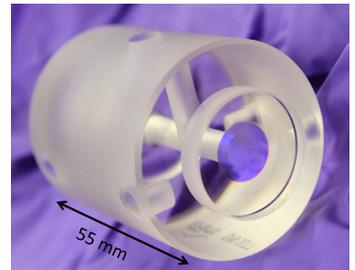
**Figure 5.7.** ULE cavity spacer with a length of 55mm and a diameter of 44mm. For the evacuation purpose, a hole with a diameter of 6 mm were drilled from the top downwards into the center, and another hole with the same diameter was drilled along the cavity length direction.
