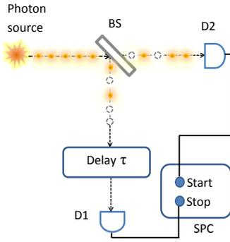
**Figure 2.11.** The photon stream is split into two paths by a 50/50 beam splitter. Detectors D1 and D2 record the photons arriving by each path. The pulse resulting from a single photon is registered by a single photon counting board, allowing a histogram of the events when both detectors are triggered to be constructed as a function the time delay  $\tau$  between the two paths.
