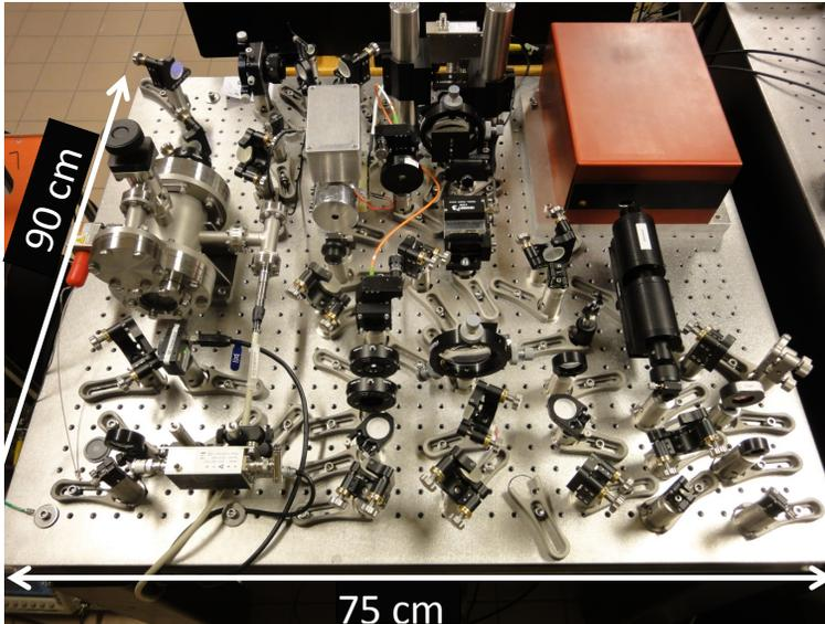
**Figure 5.12.** The 371 nm laser stabilization platform measuring 75 cm  $\times$  90 cm.
