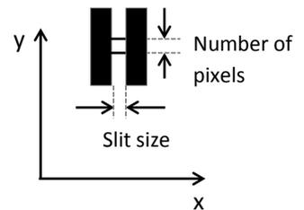
**Figure 8.11.** The size of the slit can be controlled along x axis, and the number of pixels in the CCD camera can be controlled in y axis.
