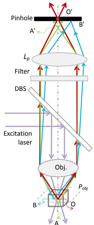
**Figure 2.8.** The working principle of a confocal microscope. A pinhole and the focal plane  $P_{obj}$  of the objective lens constitute the image planes of the lens system. Points  $O'$ ,  $A'$  and  $B'$  are the respective image point of  $O$ ,  $A$  and  $B$  in plane  $P_{obj}$ . The fluorescence signal from the out-of-focus points such as  $A$  and  $B$  are rejected by the pinhole.
