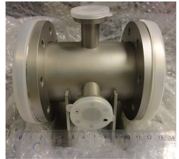
**Figure 5.6.** Steel vacuum chamber for the cavity spacer.
