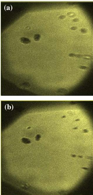
**Figure 4.6.** Tests on the aberration correction function of the objective lens (LUCPLFLN 20 $\times$ ). (a) shows the image of some micro-spheres with no aberration correction, and (b) shows the same image with correction.
