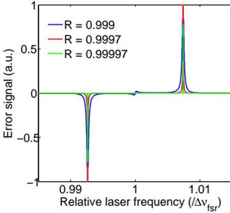
**Figure 5.5.** Error signal similar to Figure 5.4, but for an extra  $90^\circ$  phase shift in Sig2.
