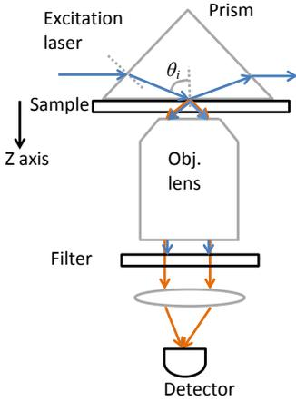
**Figure 2.9.** Evanescent field illumination to restrict the excitation volume. The light impinging to the sample has a incidence angle  $\theta_i$  larger than the critical angle  $\theta_c$ . So the incident beam is totally reflected in a stationary state. Only the penetrating evanescent field excites the sample, which limits the excitation depth to hundreds of nanometer range.
