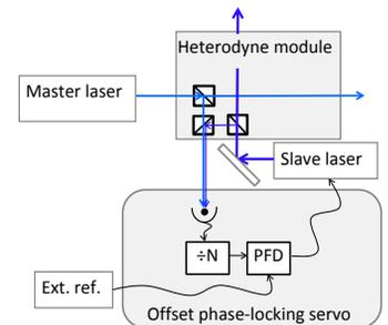
**Figure 5.13.** Schematic diagram of the offset phase-locking scheme.
