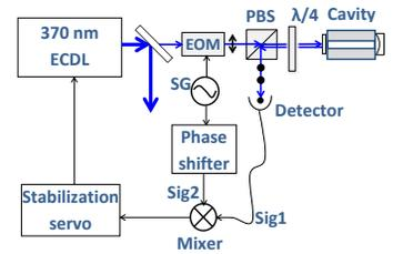
**Figure 5.3.** Schematic illustration of a PDH locking set-up. The phase modulation on the light is implemented by an EOM. The reflected beam from the cavity is detected by a photodiode, then this electronic signal further goes into a mixer, where it mixes with another signal with the same frequency. With proper phase adjustment between these two signals, an error signal is produced. Then it is fed back to the laser. The symbols  $\uparrow$  and  $\bullet$  indicate the light polarizations.
