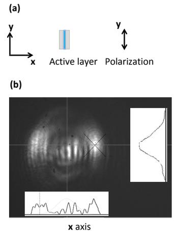
**Figure 4.4.** (a): The polarization of the light relative to the orientation of the active layer. (b): Spatial mode of the free running laser diode with a centre output wavelength of 372.1 nm. The curves show the intensity distribution along two axes.
