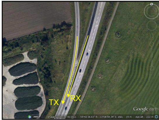
Figure 1: Google Earth TM [14] aerial image shows the investigated merging lane scenario outside the city of Lund. The TX enters the highway while RX is approaching the merging point on the highway. (N 55°42'36\", E 13°8'53\")
