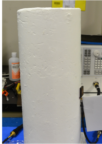
Figure 1.16: A cylindrical semisolid phantom used for the measurement of the channel around the body.
