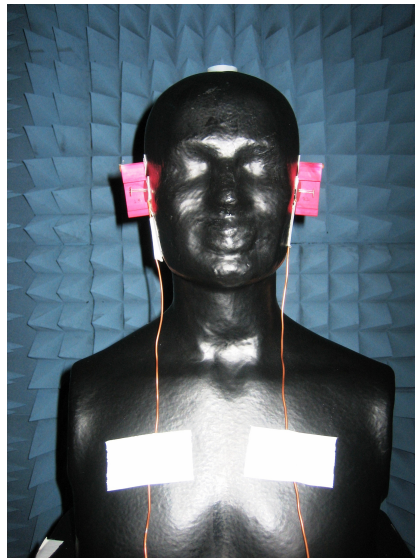
Figure 13: Phantom used for the measurement. The placement of the antennas and the pinna can also be seen.
