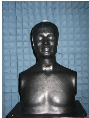
Figure 1.15: A Physical Shell Phantom with Head and Shoulder
