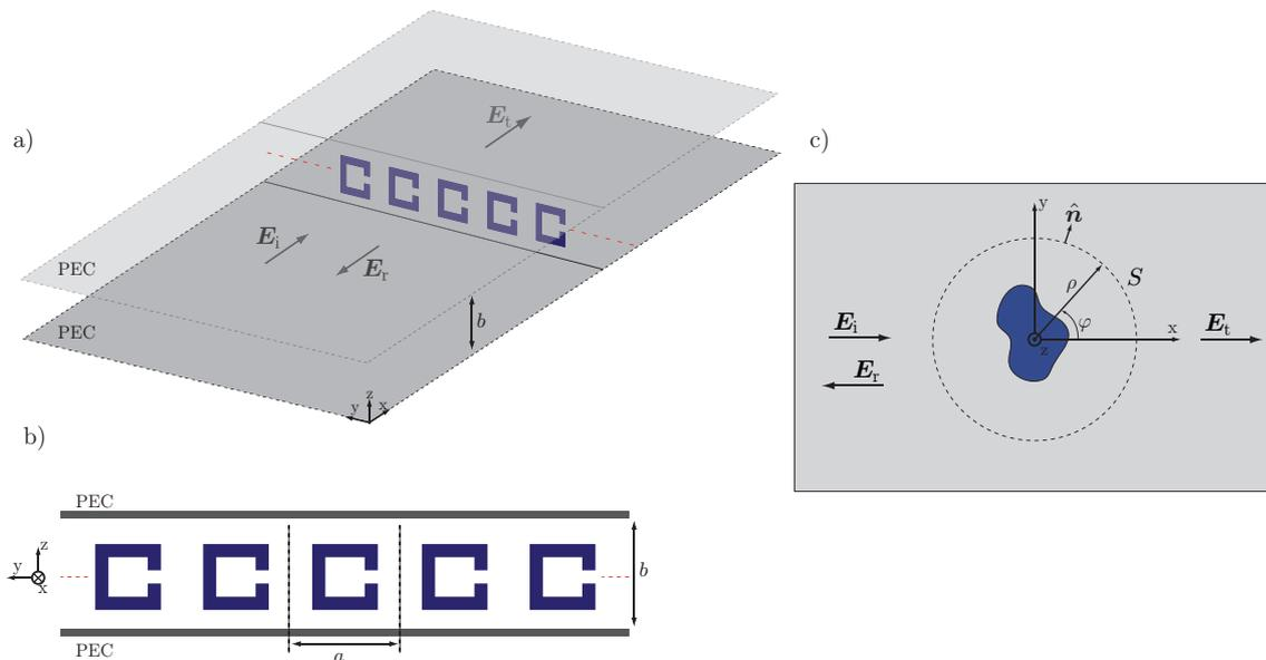
**Figure 1:** Scattering geometry for periodic objects inside the parallel plate waveguide. a) perspective view.  $\mathbf{E}_i$  is the incident field,  $\mathbf{E}_t$  the transmitted field, and  $\mathbf{E}_r$  denotes the reflected field. b) front view. The unit cell size is  $a \times b$ . c) top view of the parallel plate waveguide. The imaginary surface  $S$  is a cylinder of radius  $\rho$  and normal vector  $\hat{\mathbf{n}}$ , that encloses the object.
