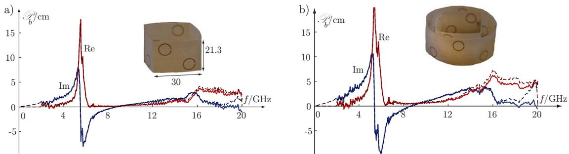
**Figure 5:** a) Measured values (solid curves) and the optimal solution (dashed curves) for the forward scattering of a) a cube of SRRs with the diameter of the unit element,  $\ell = 8$  mm and b) a cuboid-shaped SRR structure inside a cylinder of split ring resonators with the diameter of unit element,  $\ell = 8$  mm.
