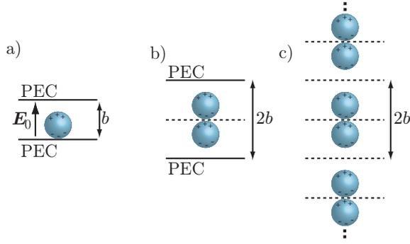
**Figure 2:** Periodic equivalence problem. a) An object is placed in an arbitrary position between the plates of a capacitor. b) An equivalent problem for part-a by placing the object and its image at the mid point between two plates. c) The equivalent periodic problem.
