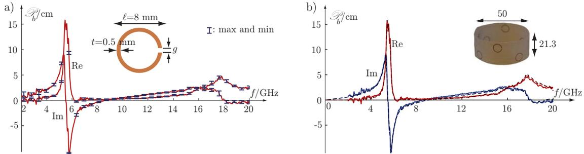
**Figure 4:** a) Average of the 10 measurements (solid curves) for the forward scattering for an array of circular split rings, see Fig. 4b. Maximum and minimum values over the 10 measurements are illustrated by the bars. b) Measured values (solid curves) and the optimal solution (dashed curves) for the forward scattering of a cylinder of split ring resonator with the diameter of unit element,  $\ell = 8$  mm.
