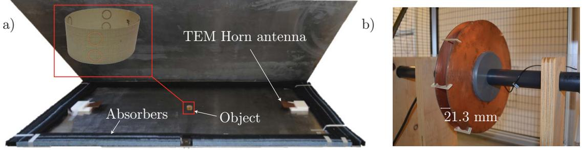
**Figure 3:** a) The parallel plate waveguide setup consists of two TEM horn antennas and microwave flat absorbers. The distance between the antennas is 98 cm and the object is placed at the midpoint between the antennas. The two plates are  $150 \times 100 \text{ cm}^2$  and separated by 21.3 mm. b) The parallel plate capacitor setup consists of two circular copper plates held by plastic arms. The distance between the plates is 21.3 mm and is fixed by plastic distance supports
