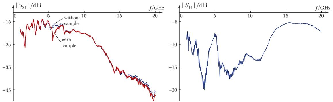
**Figure 7:** Measured values of  $|S_{21}|$  in the presence (solid) and the absence (dashed) of the object is shown in the figure on the left. The figure on the right side shows the  $|S_{11}|$  in the absence of the object.
