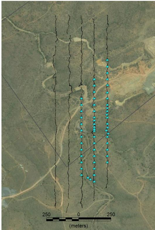
Figure 29. Detailed magnetic profiles 1-5 (west to east) and location of the SP measurements (turquoise triangles).
