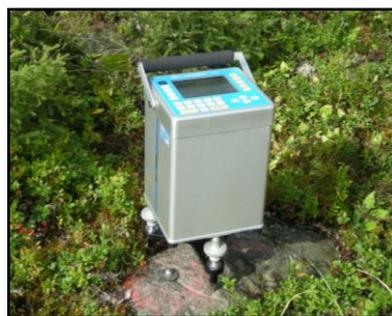
Figure 19. The gravity meter used in the project is of the type Autograv Scintrex CG-5. (Photo: Patrick Johansson, 2013)
