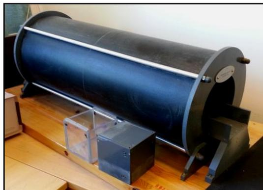
Figure 21. The Remanence Meter R4 used in the project. In front of the apparatus are the boxes in which the sample are placed. (Photo Cecilia Jönsson, 2013)
