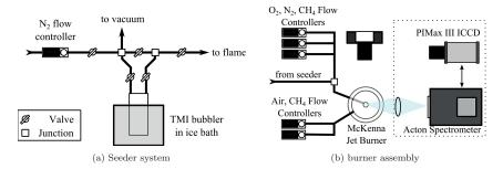
Figure 2: Burner assembly with attached indium seeding apparatus. Imaging systems are changeable between a Princeton Instruments ICCD camera and Acton  $\frac{1}{2}$  meter spectrometer.
