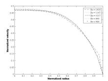
Figure 4 The normalized velocity profiles for the 4 mm nozzle The marker (x) shows the interpolated flow profile for Re = 948, which corresponds to the A1 gas measurement at  $\emptyset$  = 1.41.
