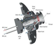
Figure 1 Scaled 4<sup>th</sup> generation DLE burner. The red arrows indicate fuel flow and blue arrows air flow. RPL thermocouple placements are indicated by yellow dots. The throat section of the burner is highlighted in red.
