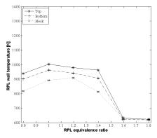
Figure 8 Temperature measurements for methane. Volume flow 0.12 m<sup>3</sup>/s
