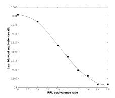
Figure 11 Change of blowout limit for syngas when varying RPL equivalence ratio. Volume flow 0.09 m<sup>3</sup>/s
