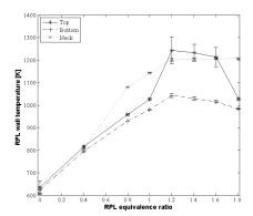
Figure 12 Temperature measurements for syngas. Volume flow 0.09 m<sup>3</sup>/s
