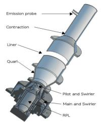
Figure 1: Burner Assembly
