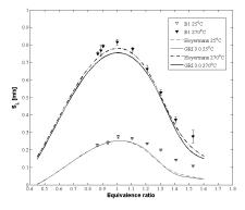
Figure 9 The measured laminar flame speeds for gas B1 at  $T_u$ =25 °C and  $T_u$ =270°C.
