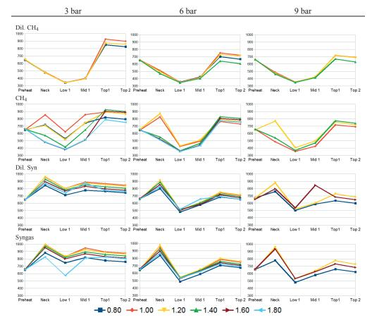
**FIGURE 3**: Temperature averages for preheater and RPL mounted thermocouples for the various pressures, fuels and equivalence ratios tested. Images show from top to bottom; dilute methane, methane, dilute syngas, and syngas. Pressures are shown from left to right; 3, 6 and 9 bar
