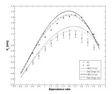
Figure 8 The measured laminar flame speeds for gases A1 and A2 at  $T_u$ =25 °C.
