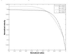
Figure 3 The normalized velocity profiles for the 10 mm nozzle. The marker (x) show the interpolated flow profile for Re = 892, which correspond to the methane measurement at  $\emptyset$  = 1.056.
