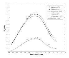
Figure 7 The measured and computed flame speeds for methane at  $T_u$ =25 °C and  $T_u$ =270°C.
