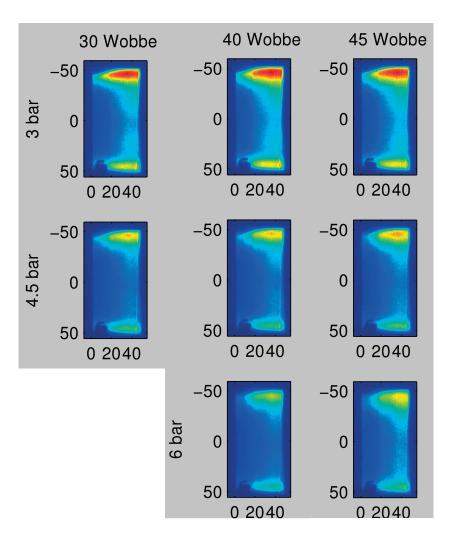
Figure 6.3: Elevated pressure testing of DLE burner using natural gas of various energy content after dilution with nitrogen. Burner is at left of the image region, laser sheet enters from the bottom. Scale is uniform for all images, with blue being the lowest intensity, red the highest.
