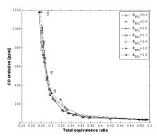
Figure 13 CO emission from lean blowout measurement for diluted syngas. Volume flow 0.13 m<sup>3</sup>/s
