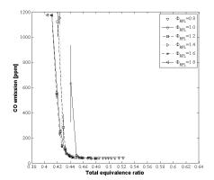
Figre 6 CO emission from lean blowout measurement for methane. Volume flow 0.12 m³/s
