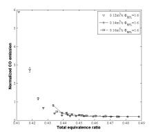
Figure 9 CO emission from lean blowout measurement for methane
