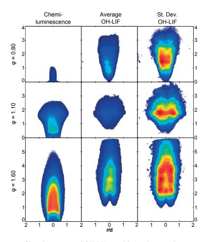
Figure 5.5: Chemiluminesce and OH-LIF signal for methane combustion in pilot sector. Three typical flame distributions shown.
