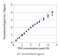
Figure 4: Calibration of seeding system, linearity of response. Purple values are from 410 nm emission and blue from 451 nm emission. Left image is data collected from several measurements, right image is data corrected against the 10 ppm signal level.
