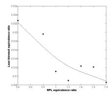
Figure 14 Change of blowout limit for diluted Syngas when varying RPL equivalence ratio Volume flow 0.13 m<sup>3</sup>/s
