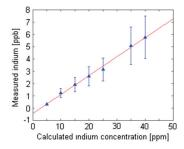
Figure 9: Indium concentration as measured by laser absorbtion versus the calculated concentration of TMI. Negative Y intercept indicates that there is a loss of Indium to the walls.
