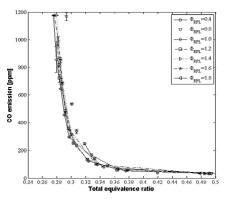
Figure 4: Dilute syngas, CO emission with total equivalence ratio for relevant RPL equivalence ratios.
