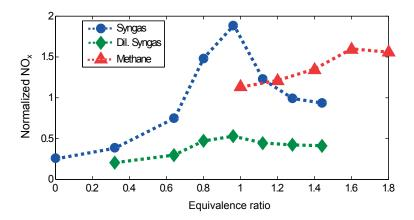
Figure 5.4: Normalized  $NO_x$  emission values for methane, syngas and dilute syngas as a function of the pilot sector equivalence ratio.
