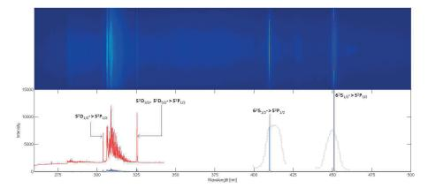
Figure 3: Flame spectrum from 26mm above the flame surface for 10 ppm TMI seeding. Indium lines are noted in the image. Overlayed with the spectrum is a 20x magnification of region from 260-340nm and the transmission curves for two Schott filters used in further experiments
