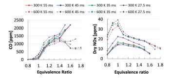
FIGURE 3: Emission collected at various operating conditions. CO shown to the left, NOx emissions at right. NOx values have been corrected for water content and normalized to 15% oxygen.
