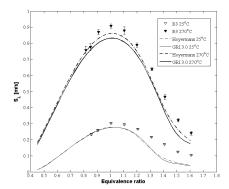
Figure 11 The measured laminar flame speeds for gas B3 at  $T_{\rm u}{=}25~^{\circ}\text{C}$  and  $T_{\rm u}{=}270^{\circ}\text{C}.$
