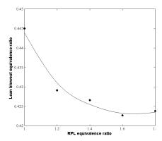
Figure 7 Change of blowout limit for methane when varying RPL equivalence ratio. Volume flow 0.12 m<sup>3</sup>/s
