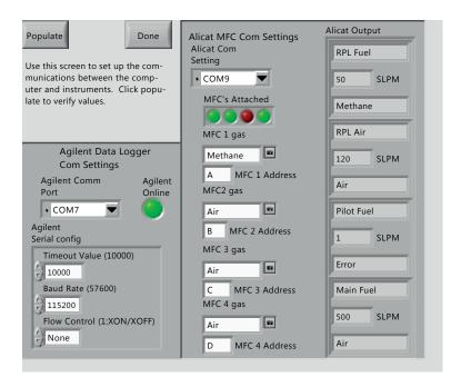
Figure 10.1: Atmospheric Burner Control Program, setup panel.
