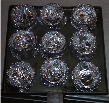
Figure A.3: 9 Ø 5cm aluminium containers used for accelerants.
