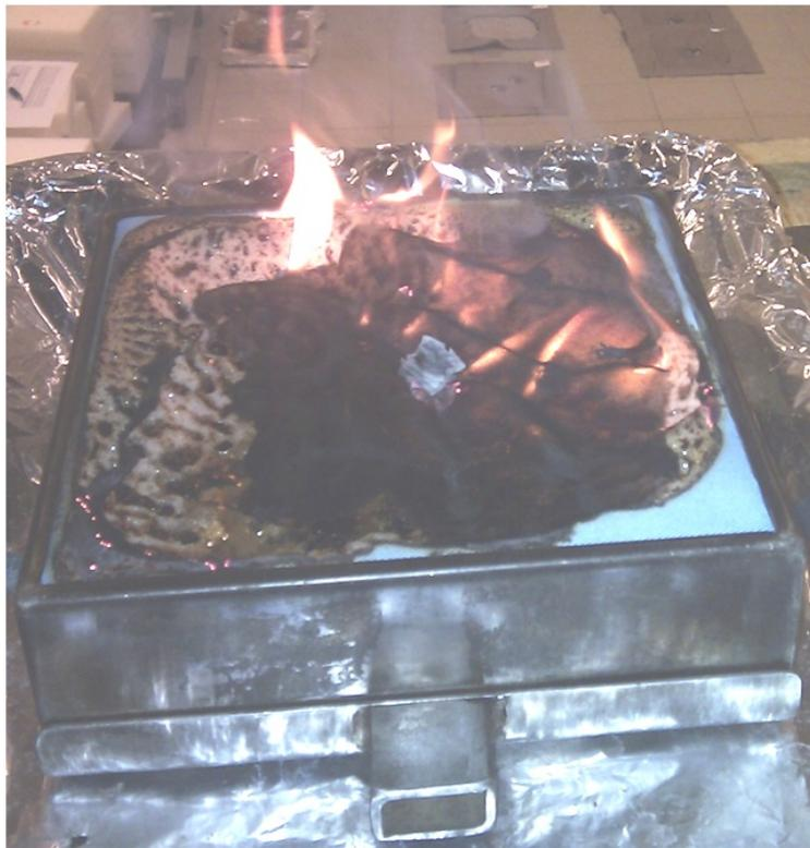
Figure 3.3: Picture of NFRC and how the cotton leaves a residue lattice protecting the foam.
