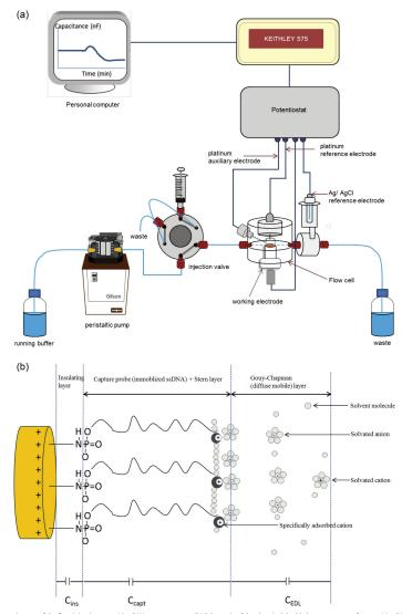
Fig. 1. (a) Experimental set up of the flow injection capacitive DNA-sensor system. (b) Schematic of the electrical double layer structure of a capacitive DNA-sensor electrode with the built-up of capacitors in series.
