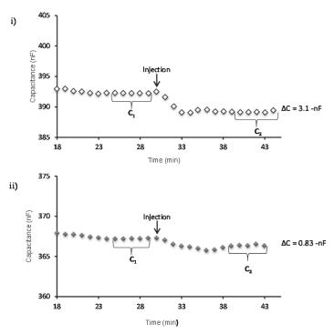
Fig. 8a: Time course graphs showing the responses from (i) Pty-ssDNA modified sensor-chip and (ii) MCH-ssDNA modified chip, to injection of 250  $\mu$ L of 10<sup>-8</sup> M target ssDNA.
