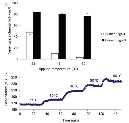
Fig. 5. (a) Capacitance change of modified electrode surface at different temperatures: 23, 30, 40, 50 and 60 °C. (b) Capacitance change from an electrode with immobilized 25-mer oligo-C, for injections of 10<sup>-8</sup> M complementary (oligo-G) and non-complementary (oligo-T), at different temperatures.
