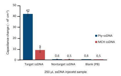
Fig. 9b: Amplitude of the responses from Pty- and MCH-ssDNA modified sensor-chips to injection of 250  $\mu$ L of a 10<sup>-8</sup> M target and nontarget ssDNA each at 50 °C.
