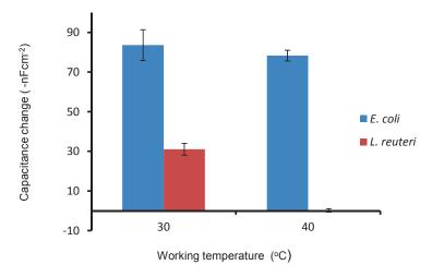
**Fig. 4-3**: Selectivity study without DNA amplification: capacitive responses from DNA-sensor chip immobilized with 30-mer *E. coli* 16S rDNA following injection of unamplified whole genomic DNA samples at concentration corresponding to  $10^5$  cell ml<sup>-1</sup> of *E. coli* and *L. reuteri* samples. Working (hybridization) temperatures were 30 and 40 °C, and constant concentration of 30 % formamide in the mobile phase.
