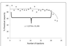
**Figure 6:** Response from a 30-mer *E. coli* 16S rDNA modified electrode to 23 injections of a 250  $\mu$ L of standard complementary 30-mer *E. coli* 16S rDNA (1.0 × 10  $^{\circ 1}$  M) with intermittent regeneration steps.
