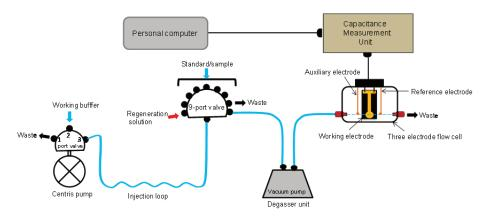
Fig. 1: Schematic illustration of an automated sequential injection flow system.
