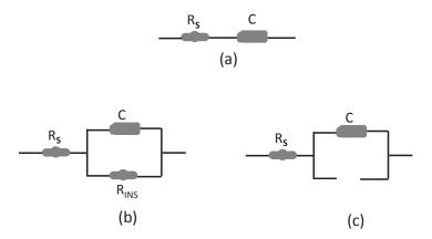
Fig. 2-13: Different model of circuits: a) RC b) R(RC), with very high resistance at  $R_{INS}$  the circuit behaves like open circuit c), very similar to RC model, since extremely large current will flow through  $R_S$  and C, which are serially connected.
