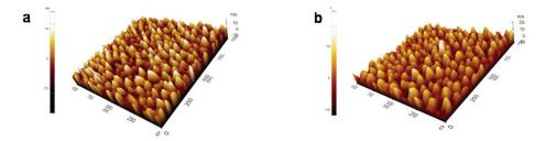
Fig. 2-8: Three dimensions (1  $\mu$ m x 1  $\mu$ m) AFM images of (a) gold electrode surface modified with Pty subsequently coupled with ssDNA (b) gold electrode surface modified with MCH and thereafter coupled with ssDNA. The images were mapped by non-contact mode AFM. The dark brown and white colours represent valley and peak, respectively.
