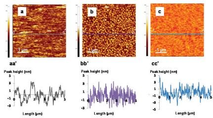
Fig. 6: The 5  $\mu$ m x 5  $\mu$ m AFM images tapped in contact mode: a) bare- (b) Pty-film-modified-, and (c) MCH SAM-modified- gold sensor-chips. The peak height profiles along the lines for (a), (b) and (c) are shown in the figures marked (aa'), (bb') and (cc'), respectively.
