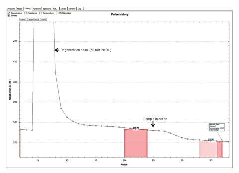
Fig. 2-20: Time course graph showing decrease of capacitance upon injection of a target analyte (25-mer *mecA* gene) in the automated flow sequential injection system (CapSenze™ Biosystem) with 10 min analysis time.
