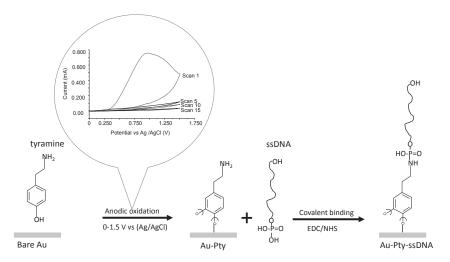
Fig. 1a: Sensor-chip surface was modified with Pty-film and followed by addition of ssDNA to form phosphoramide ester bond. The inset shows the reduction in anodic peak current during electropolymerization of tyramine on the sensor-chip surface (scan numbers 1, 5, 10 and 15).
