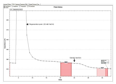
Fig. 2: Time course graph showing a signal ( $\Delta C$ ) after injection of target sample into the CapSenze<sup>TM</sup> Biosystem. The analysis took 10 minutes.
