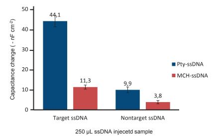
Fig. 9a: Amplitude of the responses from Pty- and MCH-ssDNA modified sensor-chips to injection of 250  $\mu$ L of a 10<sup>-8</sup> M target and nontarget ssDNA each at 23 °C.
