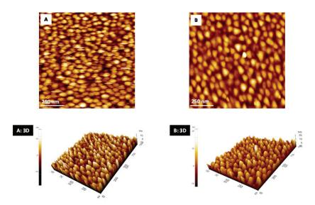
Fig 7: Non contact mode AFM images (scan size 1  $\mu$ m x 1  $\mu$ m) of (A) gold sensor-chip surface after modified with Pty and coupled with ssDNA (B) gold sensor-chip surface after modified with MCH and coupled with ssDNA. The three dimensions (3D) images of (A) and (B) are shown in the figures marked (A: 3D) and (B: 3D), respectively.
