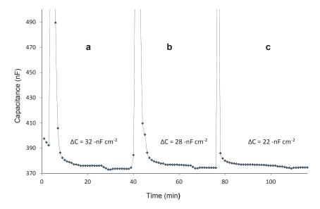
Fig. 6: Showing the observed matrix-borne signals resulted from injecting different dilutions of unspiked human saliva samples in to the capacitive DNA-sensor (a)  $10^2$  times diluted (b)  $10^3$  times diluted and (c)  $10^5$  times diluted.
