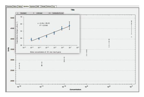
Fig. 2-21: The automatically plotted calibration curve for capacitance change vs. concentrations of injected sample (25-mer *mecA* gene). The inset shows linearity of the molar concentrations of sample (25-mer *mecA* gene) vs. capacitance change. The mean of three signal values for each concentration with its standard deviation was manually calculated from same data of the automated plotted curve
