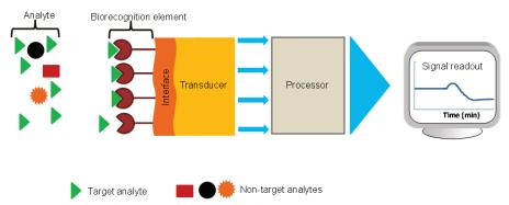
Fig. 1-1: Schematic illustration of a biosensor and its components
