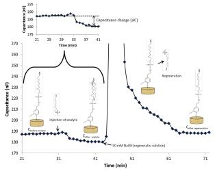
Fig. 3. Time course graph showing the capacitance; (i) before injection of analyte ( $C_{beforeanalyte}$ ) (ii) after injection of analyte ( $C_{afternaplyte}$ ) and (iii) after regeneration ( $C_{afternaplyte}$ ). Inset shows how to determine the capacitance change upon injection of analyte.
