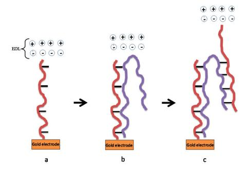
**Fig. 3-1:** Schematic representation of sandwich hybridization approach. (a) 25-mer oligo-C capture probe (b) hybridization of a target 50-mer oligo-G to the capture probe, (c) hybridization of 25-mer oligo-C after (b).
