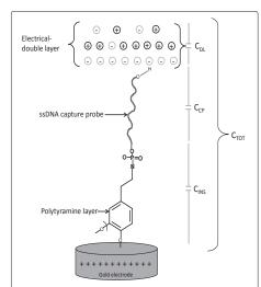
**Figure 4:** Schematic drawing of different layers covering the electrode surface comprising the total capacitance ( $C_{\rm tot}$ ),  $C_{\rm tot}$  is the insulating layer capacitance,  $C_{\rm tot}$  the capture probe capacitance; and  $C_{\rm tot}$  the double layer capacitance.
