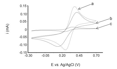
Fig. 5a: Cyclic voltammograms of (a) bare gold sensor-chip (b) gold sensor-chip modified with MCH-ssDNA (c) gold sensor-chip modified with Pty-ssDNA studied in 10 mM ( $K_3[Fe(CN)_6]$ ) in 100 mM KCl. The CV potential was swept at 100 mVs<sup>-1</sup> between a potential range of - 300 to 700 mV (vs. Ag/ AgCl).
