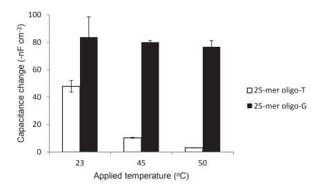
Fig. 3-3: Capacitance change from an electrode immobilized with 25-mer oligo-C (capture probe), for injections with  $10^{-8}$  M complementary 25-mer oligo-G and non-complementary 25-mer oligo-T.
