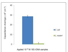
Figure 9c: Selectivity study after DNA amplification: capacitive responses from DNA-sensor chip with immobilized 30-mer *E. coli* 16S rDNA; following injection of 10.5 M amplified 16S rDNA samples from *E. coli and L. reuteri cells*, at working (hybridization) temperature of 30°C, and 30% formamide in the mobile phase.
