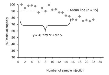
Fig. 4: Reusability of the sensor-chip. A volume of 250  $\mu$ L of a 10<sup>-9</sup> M target *mecA* gene was repeatedly applied on the sensor-chip up to 22 times with regeneration step between each individual assay.
