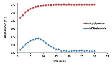
Fig. 3: Baselines for Pty and MCH modified sensor-chips at 50 °C for 30 min.
