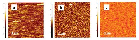
Fig. 2-7: Contact mode AFM (5  $\mu$ m x 5  $\mu$ m) images of (a) bare gold electrode surface (b) gold electrode surface after deposited with Pty film (c) gold electrode surface after deposited with MCH. The dark brown colour and white spots represent valley and peaks, respectively.
