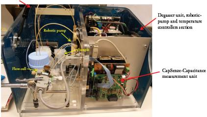
Fig. 4-5: CapSenze<sup>TM</sup> Biosystem: automated sequantial injection flow sytstem used for detection of MRSA mecA gene (for more details about the CapSenze<sup>TM</sup> Biosystem see section 2.4.2).
