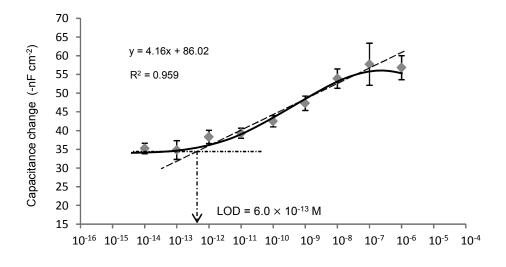
Fig 4-6: The capacitive DNA-sensor calibration curve, presenting LOD and linearity range for the detection of 25-mer *mecA* gene, prepared in PB.
