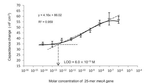
Fig. 3: The established calibration curve of the capacitive DNA-sensor showing a linearity range and LOD for 25-mer *mecA* gene sample in PB. The curve was established at 23 °C.
