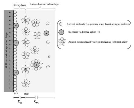
Fig. 2-10: Schematic representation of electrical double layer regions and differential capacitances in series on the gold electrode interface.
