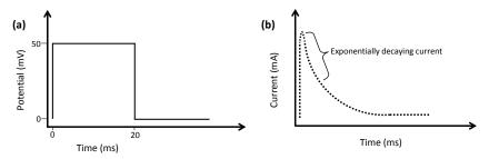
Fig. 2-14: Potential step: (a) applied potential pulse and (b) resulting exponentially decaying current.
