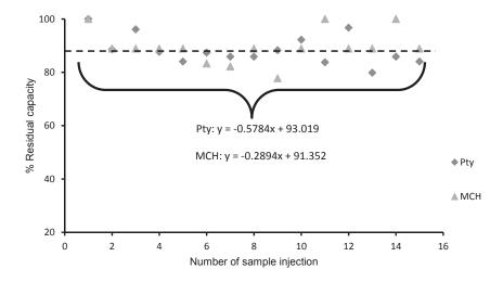
Fig. 10: Reusability of Pty- and MCH-ssDNA modified sensor-chips. 250  $\mu$ L of a 10<sup>-9</sup> M target ssDNA was repeatedly applied for 15 times on each sensor-chip with regeneration step between each individual assay.
