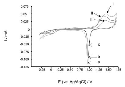
**Fig. 2-9:** The AuO reduction peaks for (a) a bare electrode surface (b) an electrode surface modified with MCH-ssDNA and (c) an electrode surface modified with Pty-ssDNA, with their Au oxidation peaks: I, II and III, respectively. Cyclic voltammograms were recorded in 0.1 M H<sub>2</sub>SO<sub>4</sub> at the sweep rate of 0.1 Vs<sup>-1</sup> and the potential range between, -0.3 to 1.7 V (*vs.* Ag/ AgCl)
