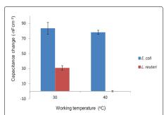
Figure 9b: Selectivity study: capacitive responses from DNA-sensor chip with immobilized 30-mer E. coli 16S rDNA, following injection of unamplified whole genomic DNA samples at concentration range corresponding to 10¹ to 10⁵ coll m¹¹ of E. coli and L. reuteri, at working (hybridization) temperature of 30°C, and 30% formamide in the mobile phase.
