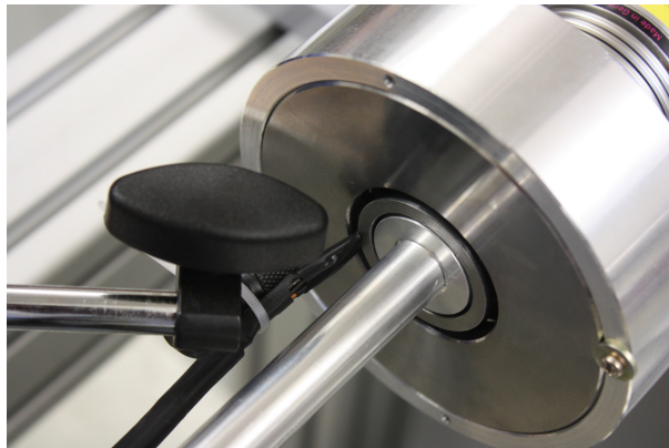
Figure 4.14: The Hall-sensor placed in the air gap of the torque sensor prototype.
