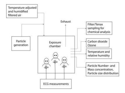
Figure 1. Simplified sketch of the experimental set-up for the chamber exposure studies.
