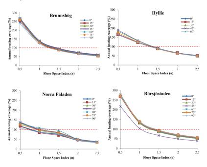
Figure 6: Annual heating coverage at different densities
