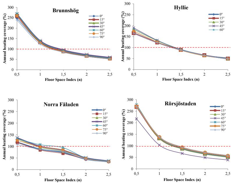
Figure 6: Annual heating coverage at different densities
