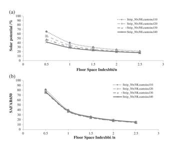
Figure 4. Solar potential as the percentage of building envelope which receives an amount of solar radiation greater than or equal  $650\,\mathrm{kWh/m^2}$ a (after Compagnon (2004)). Solar potential as the percentage of the building envelope which receives an amount of solar radiation greater than or equal  $650\,\mathrm{kWh/m^2}$ a related to the floor area (SAFAR<sub>650</sub>).
