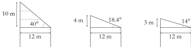
Figure 6.6 Consequences of roof types on building height
