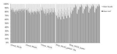
Figure 14. The share of irradiation on all suitable areas (roof and façade) per design type.
