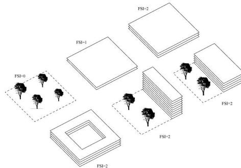
Figure 1. Principle of Floor Space Index (FSI).
