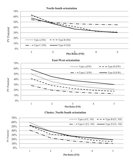
Fig. 4. PV potential of the blocks
