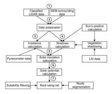
Figure 1. Methodology to produce a solar map [11]
