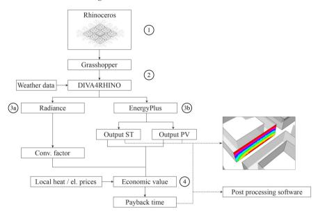
Figure 1. Workflow of the FASSADES tool.
