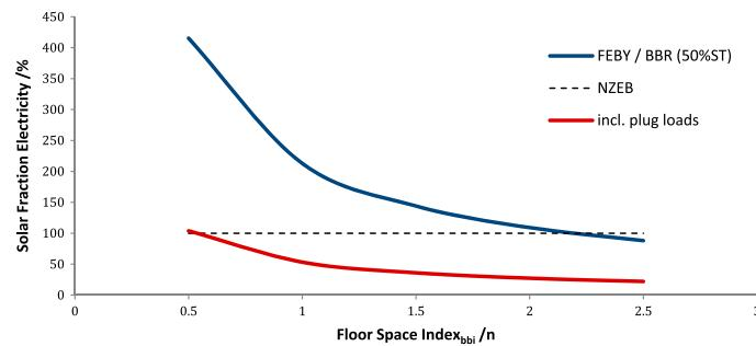
Figure 10. Load matching for electricity demand (generalised).
