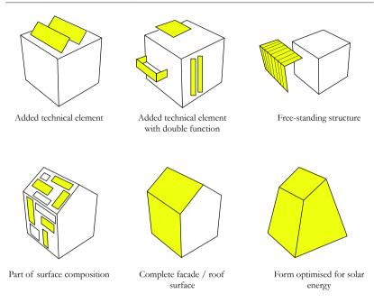
Figure 2.4 Categories of integration (adapted after Farkas et al., 2013)
