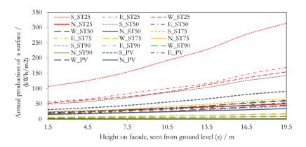
Figure 5.3 The annual energy production as a function of height from ground.
