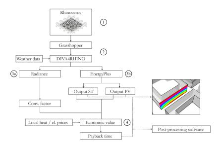
Figure 5.1 Workflow of the FASSADES tool
