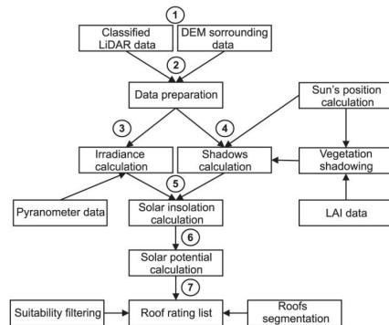
Figure 1. Methodology to produce a solar map [11]
