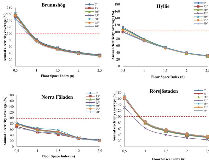
Figure 5: Annual electricity coverage at different densities
