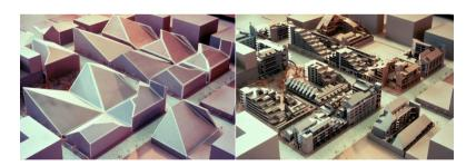
Figure 2.2 Knowles' solar envelope applied to an urban plan
