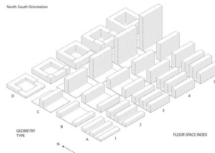
Fig. 1. Overview of geometry types in North-South orientation
