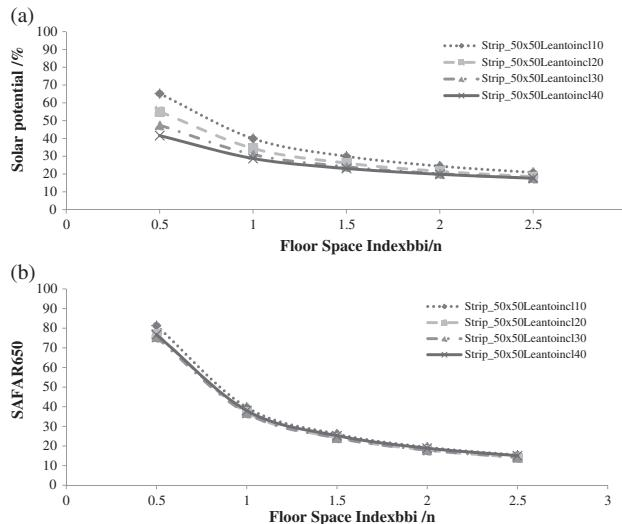
Figure 4. Solar potential as the percentage of building envelope which receives an amount of solar radiation greater than or equal  $650 \text{ kWh/m}^2\text{a}$  (after Compagnon (2004)). Solar potential as the percentage of the building envelope which receives an amount of solar radiation greater than or equal  $650 \text{ kWh/m}^2\text{a}$  related to the floor area ( $\text{SAFAR}_{650}$ ).
