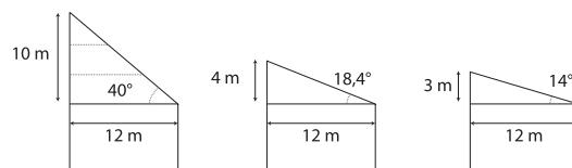
Figure 13. Consequences of roof types on building height.
