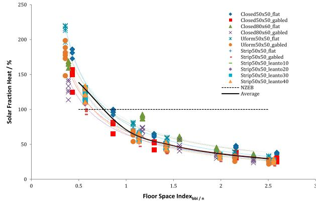
Figure 9. BBR load matching for heating demand.
