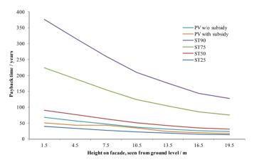
Figure 8. Payback time as a function of height.
