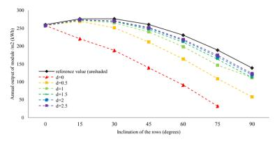
Figure 4. Output of the reference module and the shaded module in Miami.
