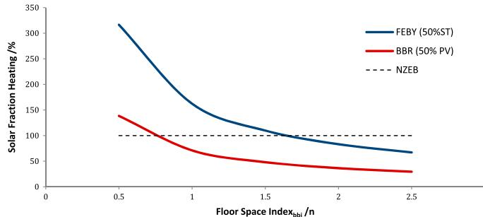
Figure 11. Load matching for heating demand (generalised).
