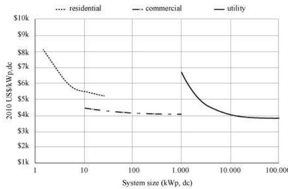
Figure 5. Residential, commercial, and utility scale PV system prices (installed) [13]
