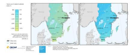
Figure 1.5 Irradiation on an optimal inclination (left) and on a horizontal plane (right) in southern Sweden (PVGIS, 2006)
