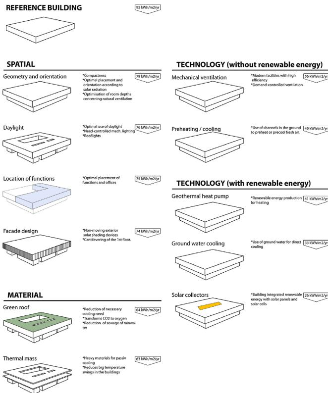
Fig. 8. Consequences of different design parameters on the energy use of a building. An example out of the design process of a Danish architect designing an office building (after Henning Larsen Architects).
