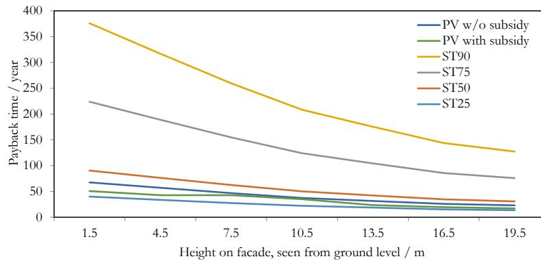
Figure 5.4 Payback time as a function of height
