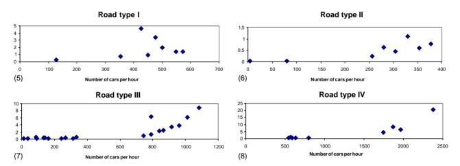
Fig. 5–8. Number of accidents per hour and kilometre ( $\times$ 1E7) at averge number of lorries per hour +/-20%. *Remark*: The total number of accidents in the figure of road type I–IV is 16, 10, 21 and 14.
