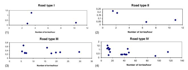
Fig. 1–4. Number of accidents per hour and kilometre ( $\times$ 1E7) at averge number of cars per hour +/-20%. *Remark*: The number of dots does not correspond to the number of accidents since more than one accident have occurred at some traffic flows. The total number of accidents in the figure of road type I–IV is 8, 18, 15 and 37.
