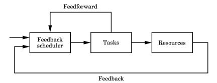
**Figure 1.3** A general feedback scheduling system. The scheduler adjusts the tasks' demands based on feedback from the current use of critical resources. The tasks may also inform the scheduler that they are about to consume more resources (feedforward).
