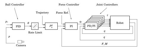
Figure 2.4 Controller structure for the slave robot.
