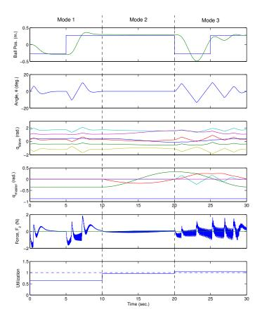
**Figure 2.8** Results using rate-monotonic scheduling. The system becomes overloaded in modes 2 and 3 with utilization close to and over 100 percent. The deteriorated control performance is clearly seen in, e.g., the plot of the ball position.
