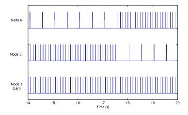
**Figure 1.13** Communication schedule showing the transmissions of node 1 (the cart), node 5 and node 6. The sampling period of the control loop is 100 ms and ping messages are sent every 500 ms. A switch between node 5 and node 6 occurs at time t=17.5.
