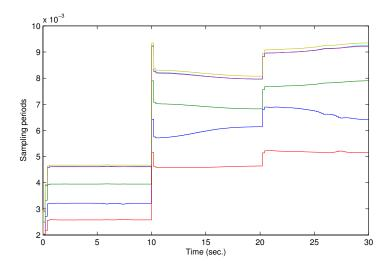
**Figure 2.10** The sampling periods of the slave robot joint controllers as functions of time. The periods increase by each mode change, but also vary within each mode as the position/orientation of the robot changes.
