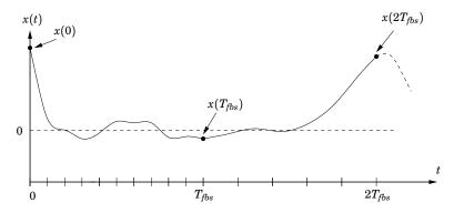
Figure 1.4 Scheduling based on plant states. Deviations in the state cause the corresponding control loop to be sampled faster.
