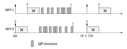
**Figure 1.6** Imprecise computation model for model predictive control tasks. The mandatory part (M) consists of finding a feasible initial solution and iterating the QP-solver until the stability requirement is fulfilled. The additional QP-iterations constitute the optional part and may be skipped.
