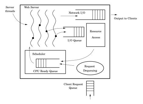
**Figure 1.7** Simplified model of a web server (adopted from [Abdelzaher *et al.*, 2003]). Requests are served by worker threads, which are put in different queues, such as the CPU ready queue or I/O access queues, during the processing of the requests.
