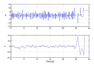
**Figure 1.14** Control signal, u, and pendulum angle,  $\theta$ , as the cart moves along the path shown in Figure 1.12. At around t=25, the cart enters a region without wireless coverage, and the pendulum falls down.
