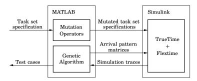
Figure 1.11 Flextime tool usage.
