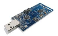
**Figure 1.15** The Telos B mote is a low power wireless module, equipped with an 8 MHz Texas Instruments MSP430 microcontroller with 10 kByte RAM and 48 kByte Flash memory.
