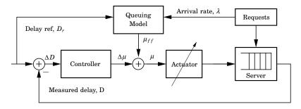
**Figure 1.8** Block diagram for combined feedforward/feedback delay control (adopted from [Sha *et al.*, 2002]).
