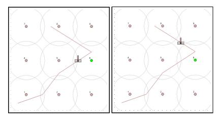
**Figure 1.12** Wireless distributed control of an inverted pendulum on a cart. The cart is moving along a pre-specified trajectory in an area of nine symmetrically distributed controller nodes. In the left figure a switch between node 5 and node 6 takes place. In the right figure the cart enters an area without coverage.
