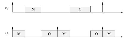
**Figure 1.5** Scheduling of imprecise computations is based on a task model where each task can be divided into two parts: a mandatory part and an optional part. The optional part may be aborted to meet scheduling constraints or to improve performance.
