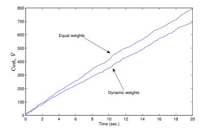
**Figure 2.11** Evaluation of the cost function (2.11) for the two feedback scheduling formulations: equally weighted cost functions and dynamically weighted cost functions based on the velocity Jacobian.
