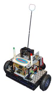
**Figure 1.16** The RBbot is an inverted pendulum on a three-wheeled cart equipped with a Telos B mote for sensing, local control and communication with other nodes in a controller network. Constructed by Rolf Braun and Anders Blomdell, Department of Automatic Control, Lund.
