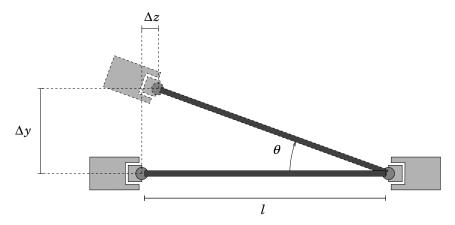
**Figure 2.5** Moving the beam an angle,  $\theta$ , from the horizontal position corresponds to translations,  $\Delta y$  and  $\Delta z$ , in the y- and z-directions, and a rotation,  $\theta$ , about the x-axis.
