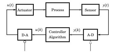
Figure 1.1 Schematic diagram of a computer-controlled system.
