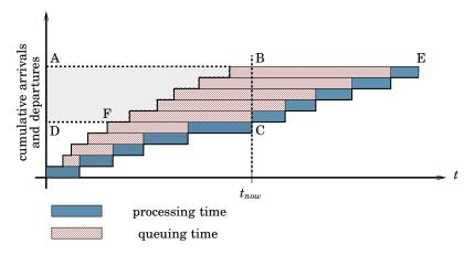
Figure 1.9 Server queuing and processing delay over time.
