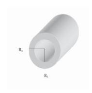
Cross-sectional moment of inertia =  $(\pi/4)$  (Ro<sup>4</sup>- Ri<sup>4</sup>) Polar moment of inertia =  $(\pi/2)$  (Ro<sup>4</sup>- Ri<sup>4</sup>)
