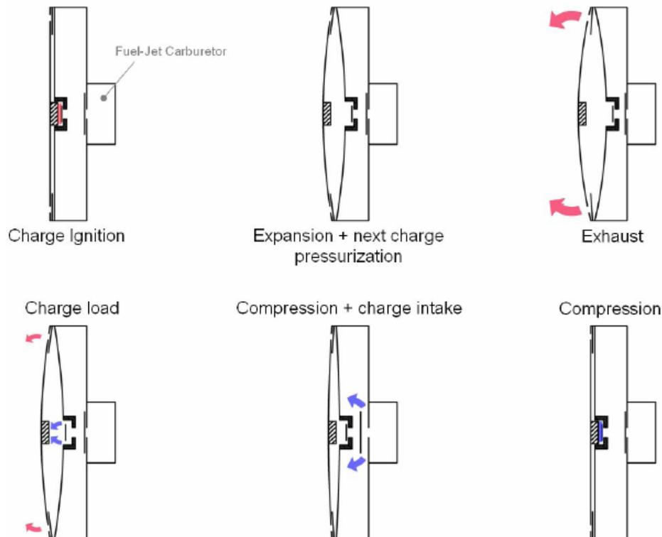
**Figure 3: The VIMPA working principle.**
