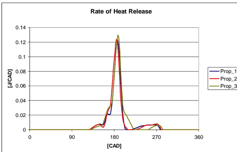
**Figure 61 a: ROHR traces for propellers: 1, 2 and 3.**
