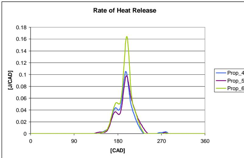
**Figure 61 b: ROHR traces for propellers: 4, 5 and 6.**
