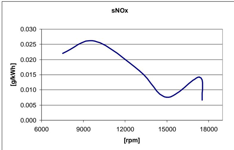
Figure 65: Specific NO<sub>x</sub> emissions versus engine speed.
