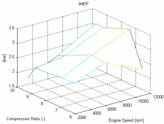
**Figure 91 a: 3-D chart of IMEP as a function of engine speed and compression ratio.**
