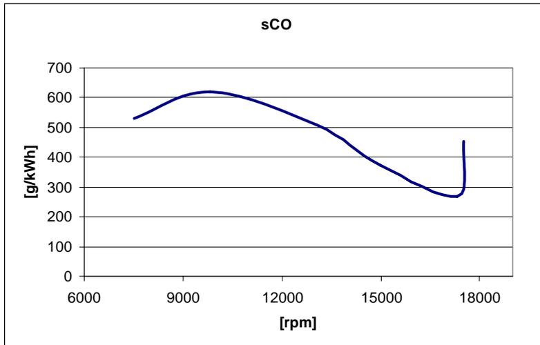
Figure 64: Specific carbon monoxide emissions versus engine speed.
