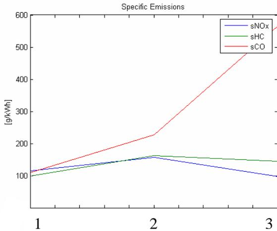
Figure 39: The variation of the specific emissions during the three tests.
