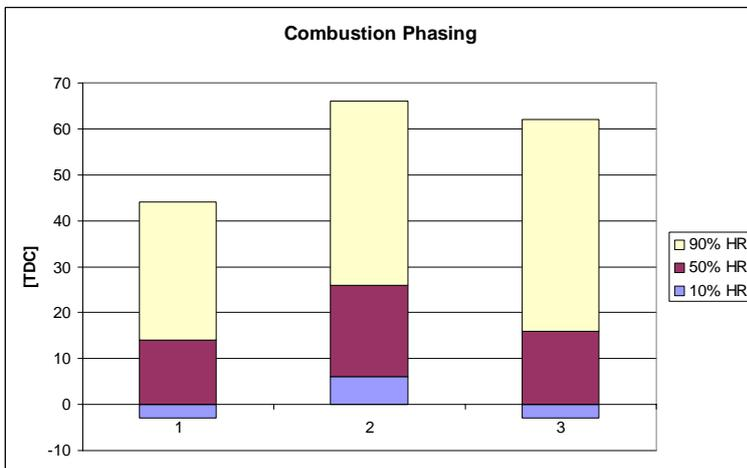
**Figure A1-8: The combustion phasing variation when heating the inlet mixture and increasing the amount of retained burned gases. 1 →  $T_{in} = 431$  [K] &  $P_{ex} = 1.12$  [bar], 2 →  $T_{in} = 298$  [K] &  $P_{ex} = 1.15$  [bar], 3 →  $T_{in} = 298$  [K] &  $P_{ex} = 1.02$  [bar].**
