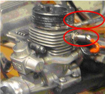
Figure 29: Glow plug and pressure sensor locations.
