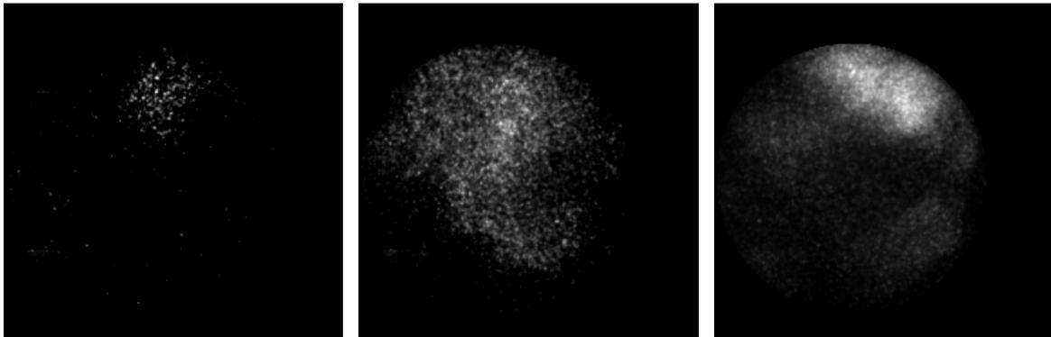
**Figure 54: Formaldehyde formation and evolution at 13400 [rpm].**
