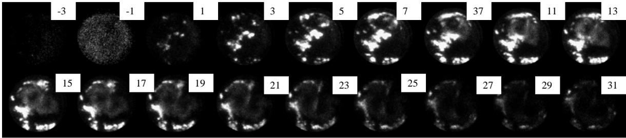
**Figure 78: C<sub>2</sub> light in a single cycle at 6500 [rpm].**
