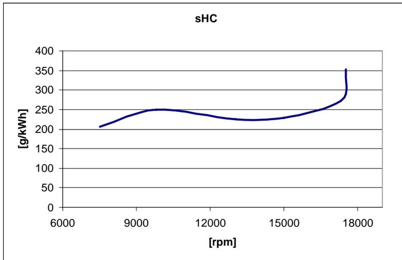
Figure 63: Specific hydrocarbon emissions versus engine speed.
