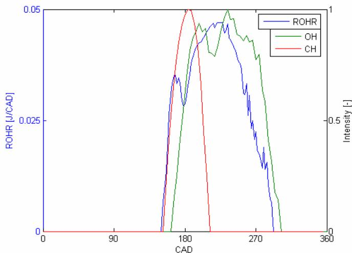
**Figure 56: CH and OH radicals as functions of the crank angle plotted together with the rate of heat release at 13400 [rpm].**
