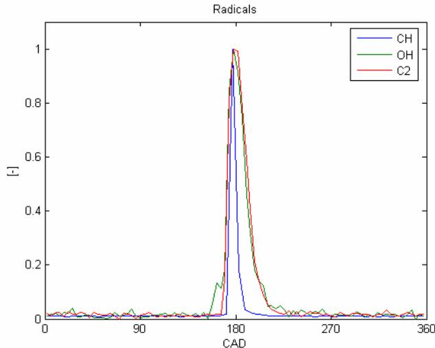
**Figure 84: Radical evolutions at 13400 [rpm].**
