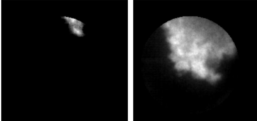
**Figure 47: The start of the combustion at 13400 [rpm].**
