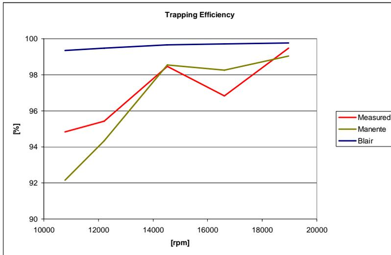
Figure 101: The measured trapping efficiency plotted with those computed with the Blair and the custom-made models.
