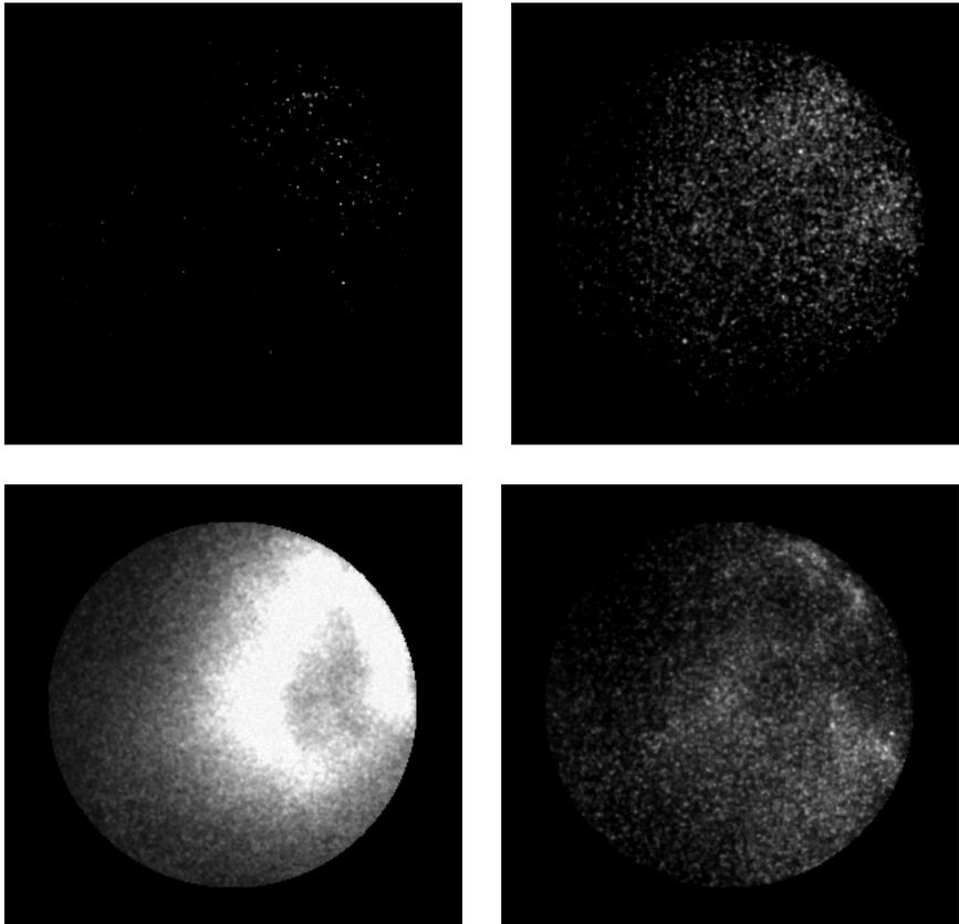
Figure 51: Formaldehyde formation and evolution at 9600 [rpm].
