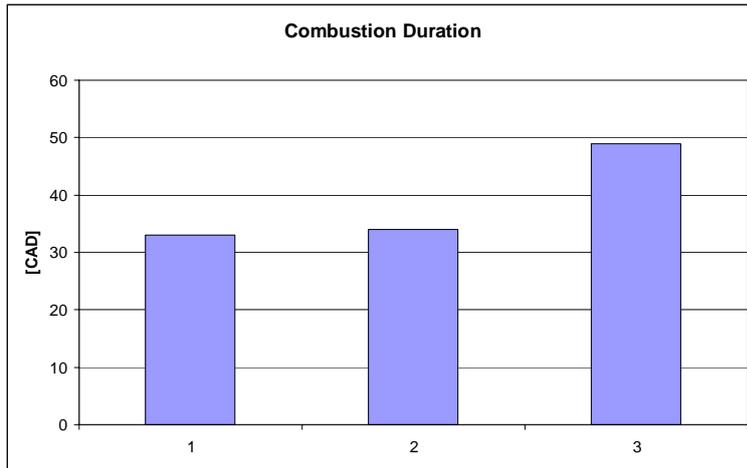
**Figure A1-9: The variation in combustion duration, 90%HR – 10%HR, when heating the inlet mixture and increasing the amount of retained burned gases. 1 →  $T_{in} = 431$  [K] &  $P_{ex} = 1.12$  [bar], 2 →  $T_{in} = 298$  [K] &  $P_{ex} = 1.15$  [bar], 3 →  $T_{in} = 298$  [K] &  $P_{ex} = 1.02$  [bar].**
