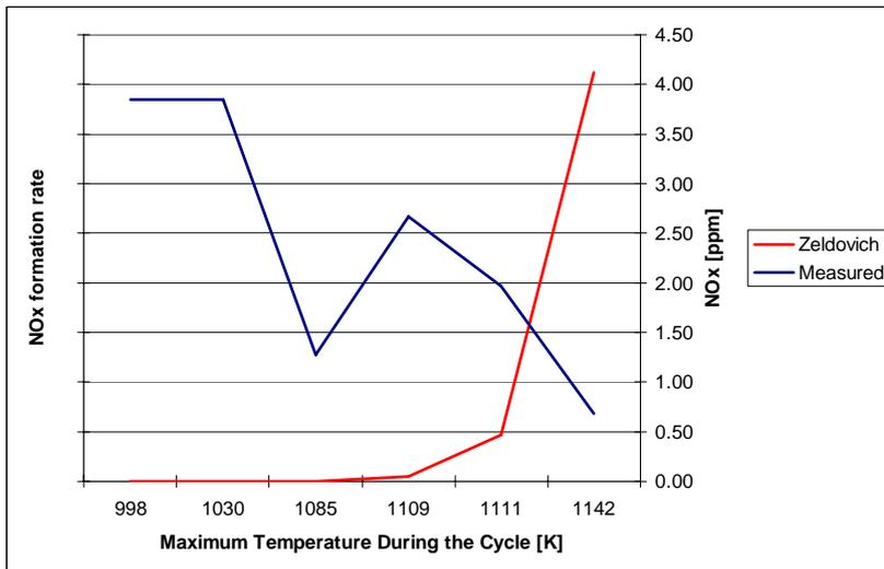
Figure 66: A comparison of the measured NO<sub>x</sub> concentrations with values predicted by the Zeldovich mechanism as a function of the maximum temperature in the cycle.
