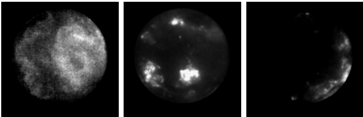
**Figure 44: Reaction distribution, soot formation and the last stage of the combustion at 9600 [rpm].**
