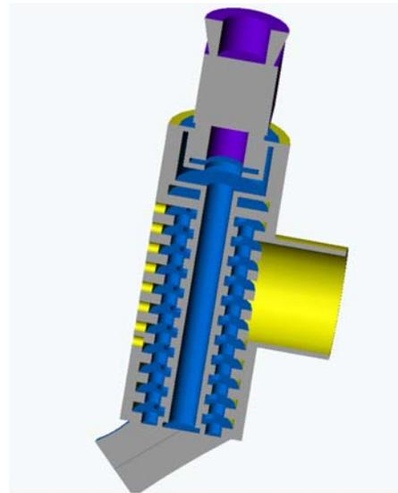
Figure 27: Heat exchanger.
