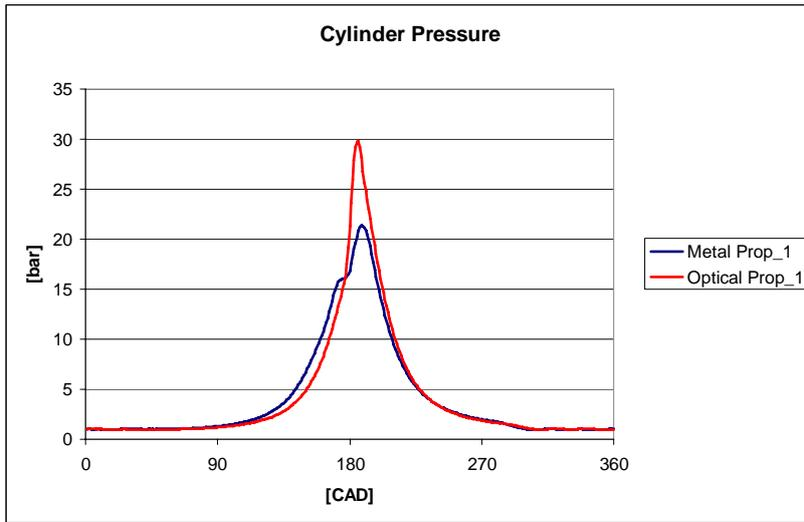
**Figure 85: Cylinder pressure traces acquired for an optical and metal engine with Propeller 1 as load.**
