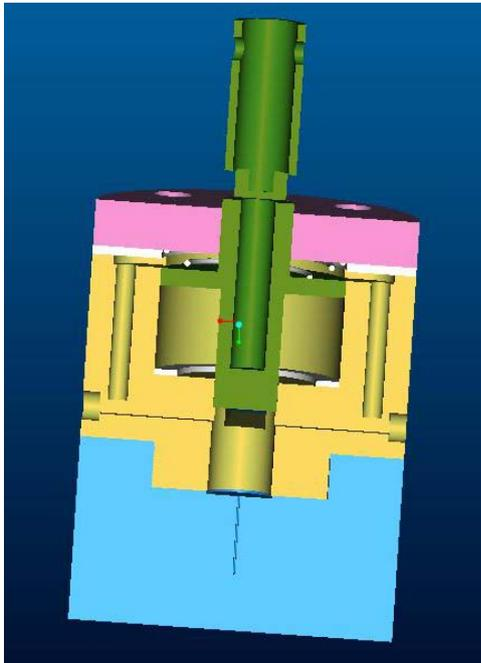
**Figure 107: Working piston at BDC and crankcase piston at TDC.**
