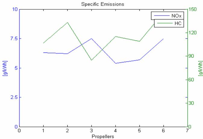
**Figure 38: HC and NO<sub>x</sub> specific emissions computed between 14500 and 17500 [rpm]. Propeller 1 is the fastest and propeller 6 the slowest.**
