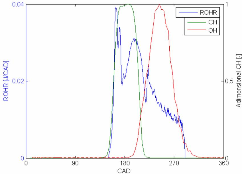
**Figure 53: CH and OH radicals as functions of the crank angle plotted together with the rate of heat release at 9600 [rpm].**
