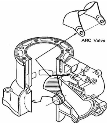
**Figure 9: A Honda ARC 2-stroke engine [23].**
