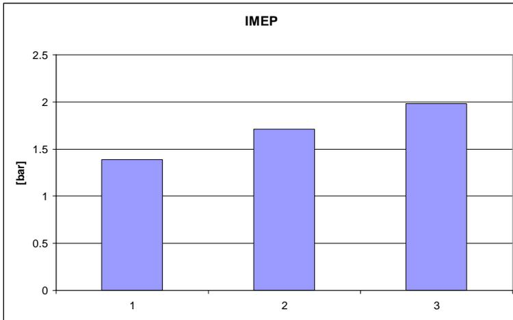
**Figure A1-7: The IMEP variation when heating the inlet mixture and increasing the amount of retained burned gases. 1 →  $T_{in} = 431$  [K] &  $P_{ex} = 1.12$  [bar], 2 →  $T_{in} = 298$  [K] &  $P_{ex} = 1.15$  [bar], 3 →  $T_{in} = 298$  [K] &  $P_{ex} = 1.02$  [bar].**
