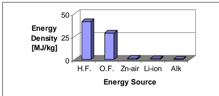
**Figure 1: The energy density of the most commonly used electrochemical batteries and average lower heating values (energy density) of hydrocarbon and organic fuels. H.F. = hydrocarbon fuel, O.F. = organic fuel, Alk. = alkaline battery**
