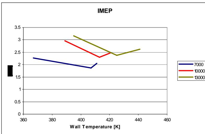
**Figure 94: The IMEP variation as a function of the wall temperature and engine speed.**
