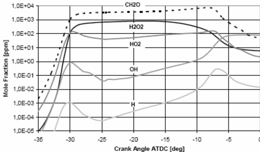
**Figure 7: Concentrations of H, OH,  $\text{H}_2\text{O}_2$  and  $\text{HO}_2$  radicals as functions of the crank angle for the 2-stage ignition of PRF 70 [18].**
