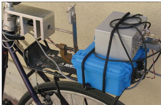
Figure 17. Rear part of the instrumented UCSB bicycle. A potentiometer is used to sense rider lean. The boxes contain a data logger and a power pack.
