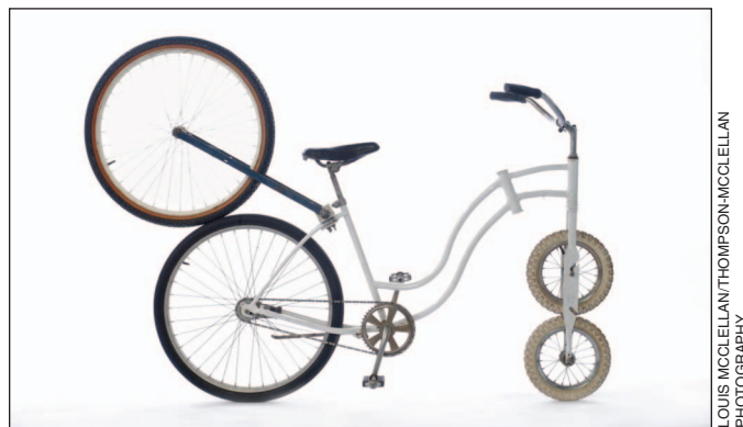
Figure 12. The UIUC naïve bicycle with precession canceling. This bicycle is used to demonstrate that a bicycle is rideable even when there are no gyroscopic effects. The bicycle is similar to the bicycle in Figure 11 but has a vertical front fork ( \lambda = 90^\circ ) and zero trail ( c = 0 , see Figure 1), which means that the front fork does not turn when the bicycle is tilted.
