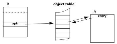
Figure 4.14 The pointer-indirection scheme of Bengtsson's incremental, compacting mark-sweep algorithm. All pointers point to an entry in an object table.
