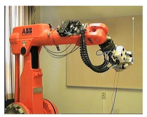
**Figure 6.3** IRB-2000 industrial robot balancing an inverted pendulum. The rod of the pendulum (to the far right) can turn freely around the shaft of a potentiometer mounted in the square housing held by the robot.
