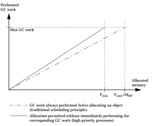
**Figure 4.8** Required performed GC work as a function of the amount of newly allocated objects in tospace. As high-priority processes may cause the current amount of performed work to be temporarily below the required amount, we must compensate for this by performing GC work in a slightly higher rate in order to avoid deadlock.
