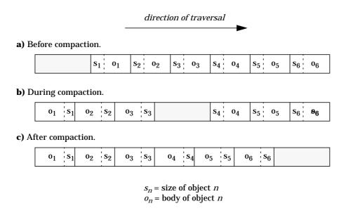
**Figure 4.16** The layout of area A of our incremental mark-sweep algorithm during an odd GC cycle. Objects are slided towards low memory. As an object is moved, the objects size word is relocated to a position immediately after the object body in order to facilitate the traversal in the opposite direction of the next, even, cycle.
