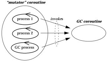
**Figure 5.2** The application program processes together with the high-priority GC process together comprise one coroutine. Another coroutine, the GC coroutine is responsible for performing GC work. The notion of real-time processes is orthogonal to the notion of coroutines. Each real-time process executes parts of both coroutines.
