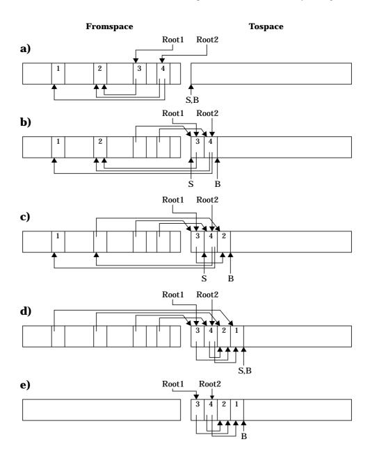
**Figure 3.2** A garbage collector cycle for a stop-the-world copying algorithm. Live objects are evacuated to tospace, after which the memory in fromspace can be reclaimed. Allocation can then proceed in tospace until it is again filled up. Then, the mean ings of tospace and fromspace are changed and the cycle starts all over again.
