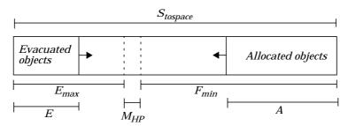
**Figure 4.7** The structure of tospace. A minimal area,  $M_{HP}$  is kept available for the high-priority process at all times.
