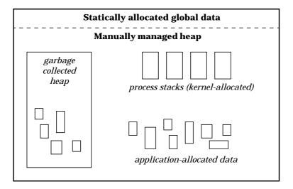
**Figure 5.3** Memory organization. The garbage collected heap is allocated at start-up on the standard system heap. The application program can chose to allocate objects on the garbage collected heap or on the manually managed system heap. Process stacks are dynamically allocated on the system heap when new processes are created.
