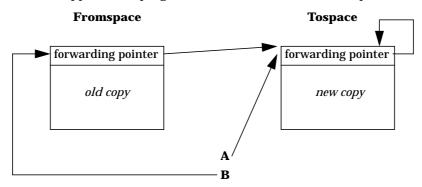
**Figure 4.3** The indirection scheme of Brooks algorithm. Dereferencing the updated A pointer or the not yet updated B pointer yields the same result, the tospace copy of the object, after following the forwarding pointer.
