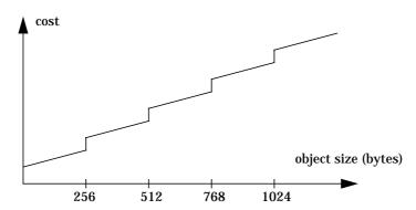
**Figure 6.5** Theoretical cost of allocation requests made by a high-priority process. The cost is slightly saw-tooth shaped due to quantification effects caused by making object initialization interruptible.
