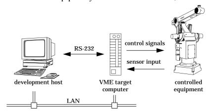
**Figure 5.1** Overview of the hardware architecture. Workstations are used to develop applications; compiling, and linking. The linked application is loaded into a dedicated control computer via the network.
