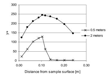
Figure 32. Variations in y<sup>+</sup> across the wall plume at two different vertical locations at the centreline, about 0.5 and 2 meters above the burner, respectively. One can note that the turbulent kinetic energy is rather low and that the entire plume falls within the fully turbulent layer, see Figure 23.
