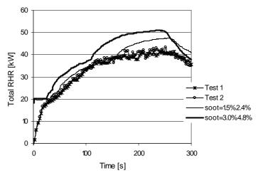
Figure 58. Effect of the prescribed soot content in the combustible gases on RHR predictions. The pyrolysis gases are modelled as being diluted propane with a prescribed soot concentration of 1.5 % and 3.0 %, respectively, the soot contribution from the propane burner being 2.4 % and 4.8 % of the fuel mass flow.
