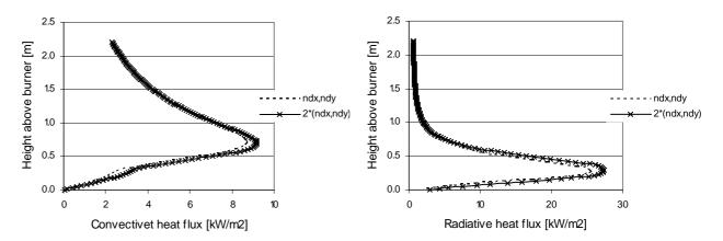
Figure 37. Dependence of the results on grid resolution in the two directions parallel to the sample surface. Results of the original simulations, termed ndx,ndy, for which there is a grid aspect ratio of about 2, are compared with those of a simulation in which the number of cells in the two directions parallel to the sample surface is twice as large.
