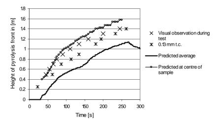
Figure 56. Predicted movement of the pyrolysis front as compared with test observations and measurements. Note that the step profile at the end of the centreline prediction is not a measure of the cell size but simply reflects the limited number of output points chosen in processing the data. The flame spread reaches a maximum at about 250 seconds, after which self-extinguishing of the panel starts.
