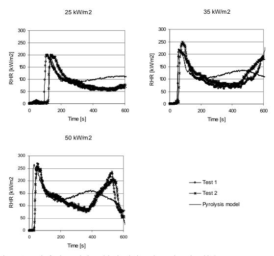
Figure 51. Results for the pyrolysis model using the input data as shown in Table 8.
