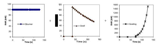
Figure 20 Contribution to the heat release rate of the different components. A comparison between the summation and the experimental data is shown in Figure 21.
