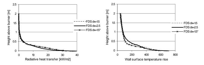
Figure 49. Radiative heat flux (left) and surface temperature rise above ambient (right) as a function of height above the burner edge. The dx denote wall-adjacent grid size in cm, the star (\*) signifying that the grid has been stretched to arrive at the resulting grid size.
