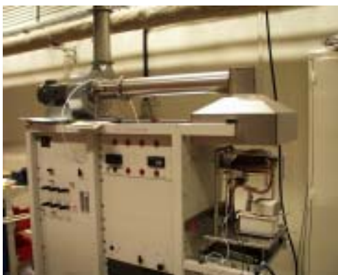
Figure 26. The Cone Calorimeter at Lund University (left) and a schematic view of the apparatus, from ref 28 (right).
