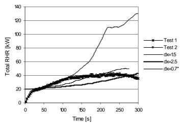
Figure 75. Comparison of measured and predicted heat release rate using different grid resolutions. The numbers designated as dx are the grid sizes in the direction normal to the sample surface, \* indicating that the grid has been stretched to obtain the resulting wall-adjacent cell size. The grid in the plane parallel to the sample is unchanged, giving a maximum aspect ratio of AR(dx=1.5)=2.0, AR(dx=2.5)=1.2, AR(dx=0.7\*)=4.3.
