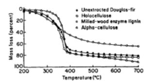
Figure 1. Mass loss of isolated wood components (Douglas fir) heated in nitrogen environment at 5 °C/min (from ref. 10).
