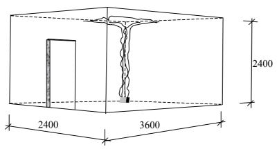
Figure 18. Sketch of the enclosure. The ceiling and the walls (except for the door-wall) have a wooden lining.
