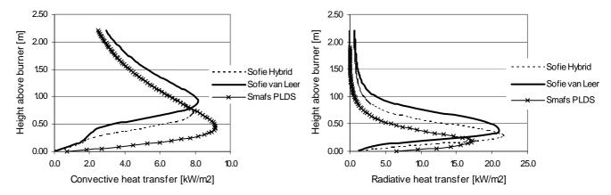
Figure 47. Incident convective and radiative heat transfer as function of height above the burner edge. The size of the wall-adjacent control volume is 2.5 cm in the direction normal to the surface.
