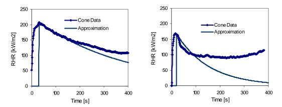
Figure 10 Data from the Cone Calorimeter at 50 kW/m<sup>2</sup> compared with an approximation using the  $\dot{Q}''_{max}e^{-\lambda t}$  relationship and the parameter values shown in Table 2. Left: MDF, Right: wooden (spruce) panel
