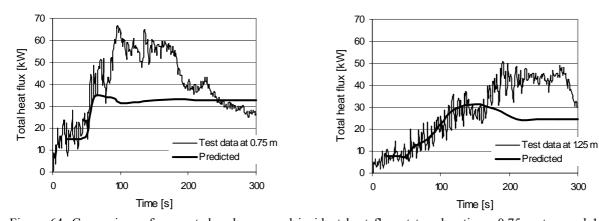
Figure 64. Comparison of computed and measured incident heat flux at two locations, 0.75 meters and 1.25 meters above the burner edge, respectively, along the centreline of the sample.
