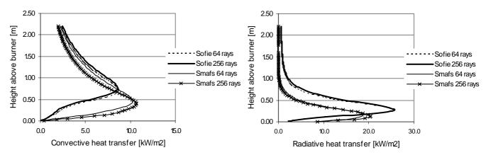
Figure 46. Incident convective and radiative heat transfer as a function of height above the burner edge. The size of the wall-adjacent control volume is 1.5 cm in the direction normal to the surface.
