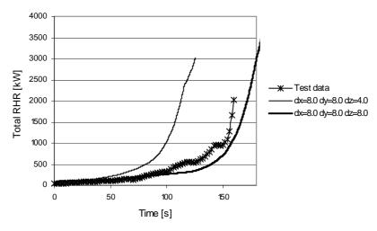
Figure 78. Sensitivity analysis of grid size in the vertical (z) direction, the symbols dx, dy and dz denoting grid sizes in cm.
