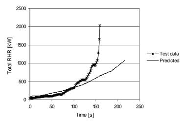
Figure 59. Total rate of heat release in the Room Corner Test. The input data is the same as used in Figure 53, with pyrolysis gas according to Fredlund being employed.
