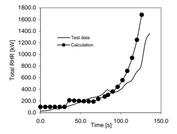
Figure 21 Fire growth in the combustible lining of a room as calculated using Equation [32]-[34].
