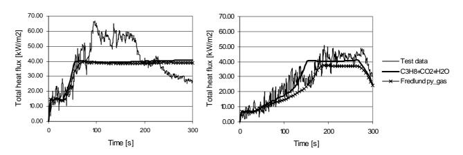
Figure 55. Total heat flux to a water-cooled probe 0.75 meters (right) and 1.25 meters (left) above the burner edge. The calculated values have been modified to apply to a probe temperature of 25 °C.
