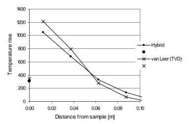
Figure 42. Temperature distribution in the direction normal to the sample surface at a location 0.5 meter above the burner edge. The values located at single points on the ordinate are wall surface temperatures.
