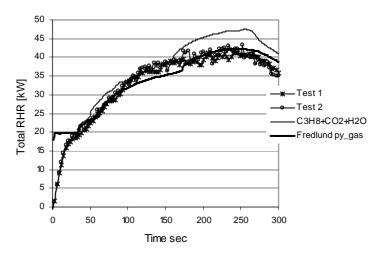
Figure 54. Influence of the composition of the pyrolysis gas. The input data is chosen in accordance with Table 8 and the wall-adjacent grid size is 0.7 cm in the direction normal to the sample.
