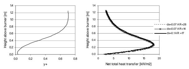
Figure 44. Resulting  $y^+$  for a wall-adjacent node size of dx=0.07 cm (left) and the total net heat flux as a function of height above burner (right). AR=Aspect Ratio, dx is the size (cm) of the wall-adjacent cell in the normal direction from the sample surface.
