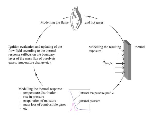
Figure 25. The flame spread calculation scheme.
