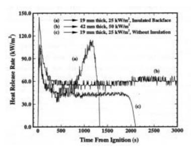
Figure 28. Effects of the thermal boundary conditions on the back face of the sample. The tests were performed with a horizontal orientation (from ref. 74).
