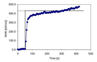
Figure 13. Representation of the rate of heat release using an average value from a Cone Calorimeter test at  $35 \text{ kW/m}^2$ .
