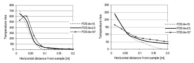
Figure 50. Horizontal temperature profiles over the fire plume at a location 0.5 meters (left) and 2 meters (right) above the burner edge, respectively. The symbol dx denotes the wall-adjacent grid size in cm, the star (\*) signifying that the grid has been stretched to arrive at the resulting grid size.
