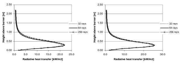
Figure 39. Influence of the number of radiation "rays" launched from the surface cells of the sample using the discrete transfer radiation model. The wall-adjacent cell size normal to the sample is 2.5 cm in the graph at the left and 1.5 cm in that at the right.
