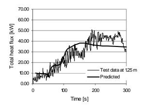
Figure 67. Computed and measured incident heat flux.
