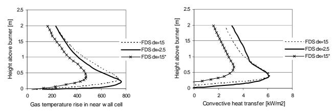
Figure 48. Rise in gas temperature over the ambient (left) and convective heat flux to the sample surface as a function of height (right). The symbol dx denote wall-adjacent grid size in cm, the star (\*) signifying that the grid has been stretched to arrive at the resulting grid size.
