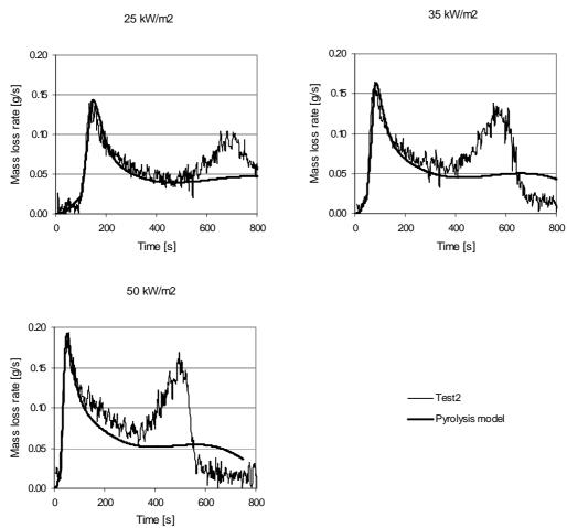
Figure 74. Predicted mass loss rate compared with experimental data.
