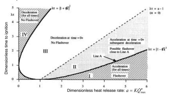
Figure 6. Graphical representations showing an interpretation of the flame spread equations in terms of accelerating or decelerating flame spread.
