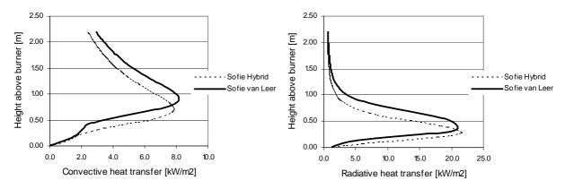
Figure 41. Influence of the numerical scheme on predictions of incident convective and radiative heat fluxes. The grid size of the wall-adjacent node, in the direction normal to the sample, is 1.5 cm.
