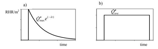
Figure 5. Mathematical representations of Cone Calorimeter data.
