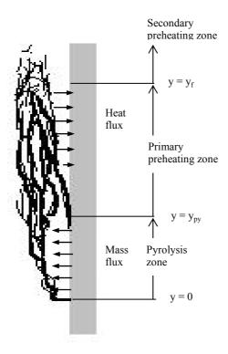
Figure 4. Diagram of upward, concurrent-flow, flame spread.
