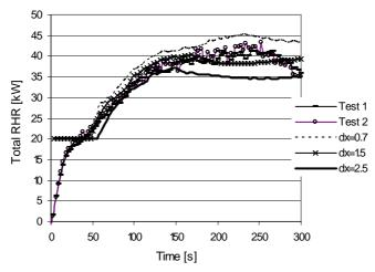
Figure 65. Effect of wall-adjacent cell size on the prediction of heat release rate using the best fit as shown in Figure 63. The grid sizes in the plane parallel to the sample are 0.026 meter large.
