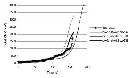
Figure 77. Comparison of total rate of heat release in the Room Corner Test, dx and dy being the node size in cm in the horizontal plane, and dz being the size in cm in the vertical direction.
