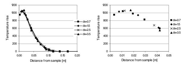
Figure 35. Temperature distribution normal to the sample surface at a location 0.5 meters above the burner edge. The graph at the right is a magnification of the left hand graph.
