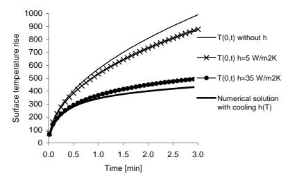
Figure 9. The effect of surface cooling in solving the heat transfer equation. In the numerical solution, cooling varies as a function of temperature but the result can be realistically approximated using Equation [24] with h=43 W/m<sup>2</sup>K. In practise, cooling originates primarily from surface re-radiation.
