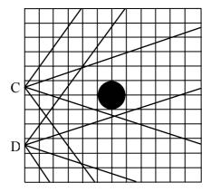
Figure 24. Two-dimensional illustration of the cause of the ray effect.
