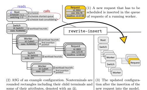
Fig. 2: Upon arrival of a new request (1), the attribute *schedule* is evaluated (2) and the request is inserted into the queue of a worker (3).
